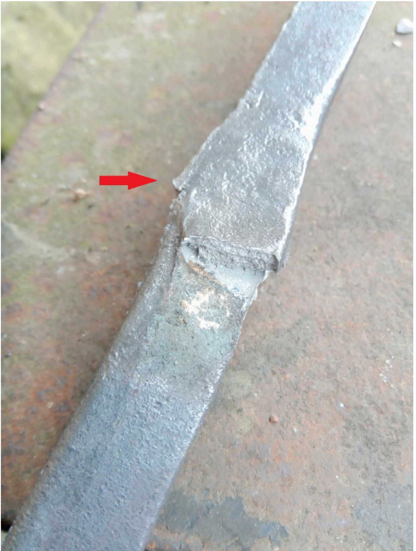
FIG 17C. THE EXPERIMENTAL RECREATION OF THE POINT B AREA, DESCRIBED FURTHER-ON IN THIS DOCUMENT, PRODUCED SIMILAR "SPLINTERS" AS A RESULT OF ADJACENT FIREWELDS SHEARING AT A POINT SLIGHTLY HIGHER-UP THE SHAFT. COPYRIGHTS BY ROWAN TAYLOR.
