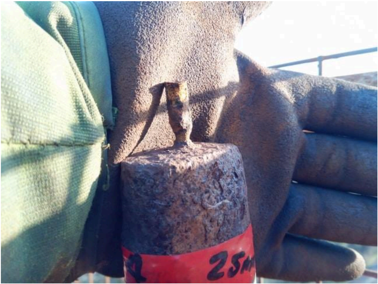
FIG 24A. EXAMPLES OF FOOTING CORROSION, SYMPTOMATIC OF AN ELECTROCHEMICAL IMBALANCE CAUSED BY THE PASSIVATION OF AN AREA OF IRONWORK. A WROUGHT IRON RIVET INCLUDED IN A CAST-IRON BALUSTER. COPYRIGHTS BY ROWAN TAYLOR
