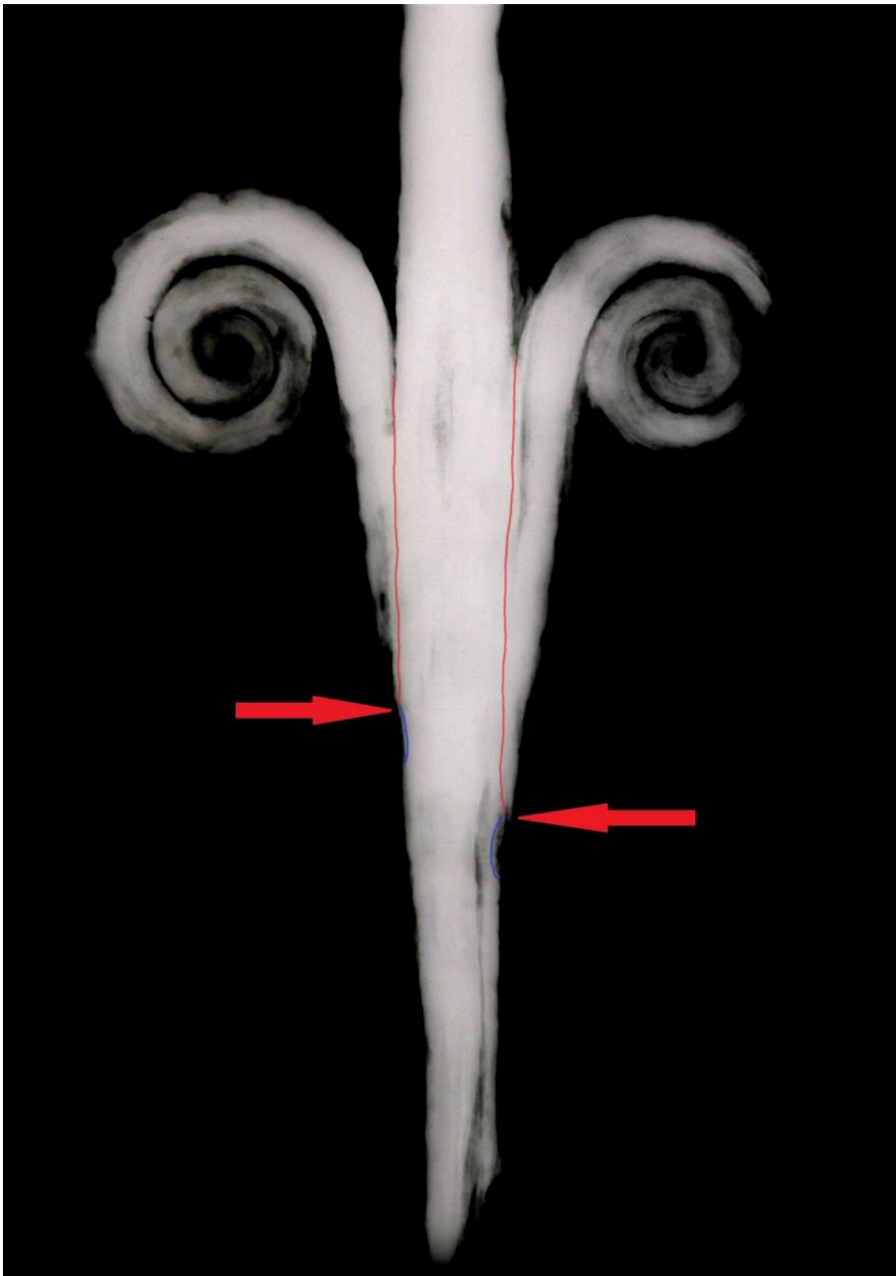
FIG 57B. THE SAME X-RADIOGRAPHY OF THE BASE OF THE STAND, WITH THE CONTRAST ENHANCED SO AS TO BETTER SHOW CONSTRUCTIONAL LINES WITHIN THE IRONWORK. THE WELD-LINES LEADING TO THE TOES ARE FAINTLY VISIBLE, HERE HIGHLIGHTED WITH RED-LINES (COMPARE TO A). IN BLUE IS THE TOE UNDERCUT, WHICH WAS DESCRIBED IN FIG 15 COPYRIGHTS BY THE TRUSTEES OF THE BRITISH MUSEUM. SHARED UNDER A CREATIVE COMMONS ATTRIBUTION-NONCOMMERCIAL-SHAREALIKE 4.0 INTERNATIONAL (CC BY-NC-SA 4.0) LICENCE.
