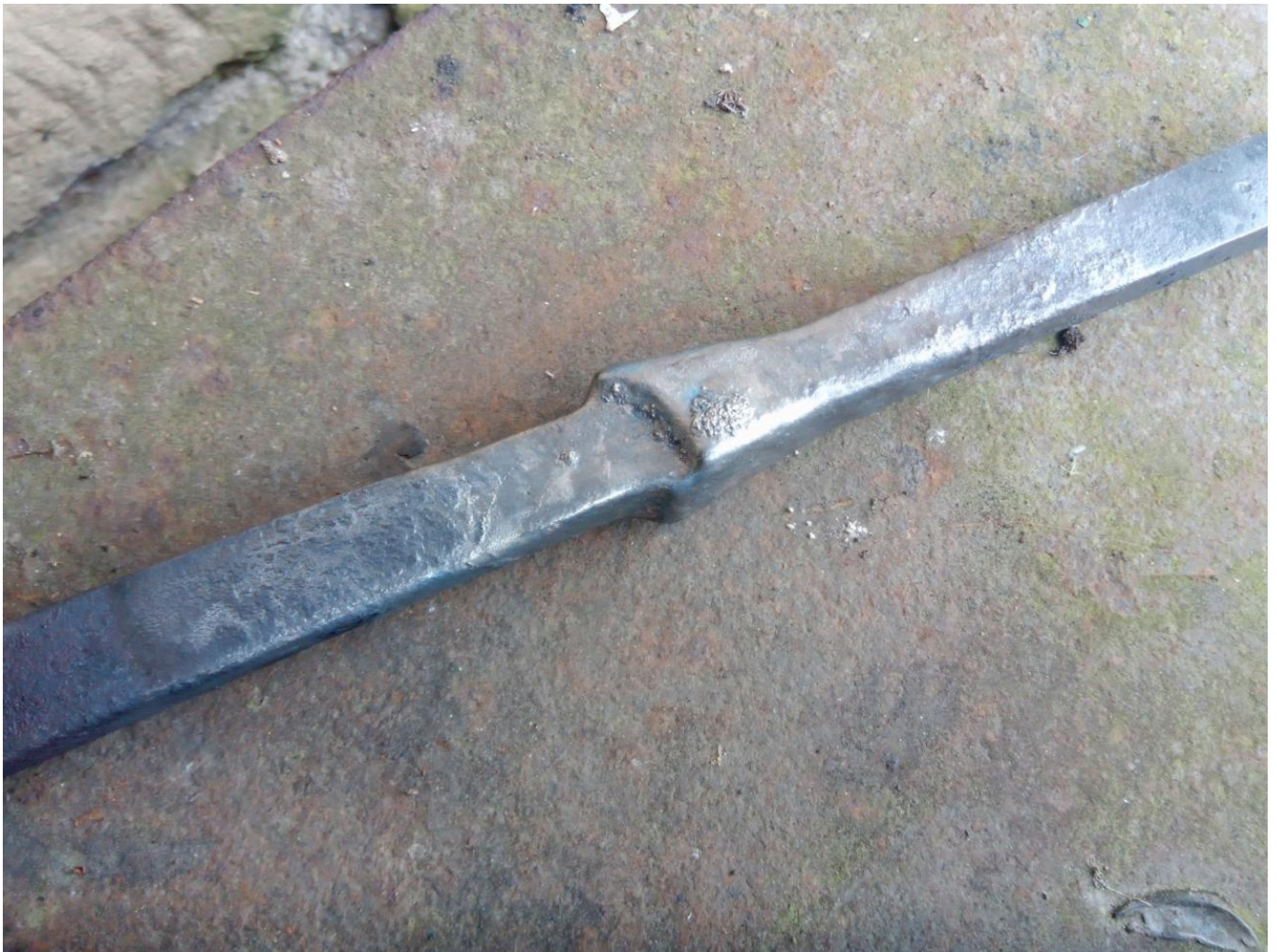
FIG 20. AFTER RECORDING THE FORMS OF THE SHEARED WELDS, A HIGH-TEMPERATURE OXIDISATION TEST WAS CONDUCTED OUT OF CURIOSITY. THE FORM CREATED IS SIMILAR IN SHAPE TO POINT B OF THE IRON STAND, HOWEVER THE CAVEAT MUST BE MADE THAT THIS METHOD PRODUCES NONE OF THE SHARPNESS OF NATURAL CORROSION. COPYRIGHTS BY ROWAN TAYLOR.
