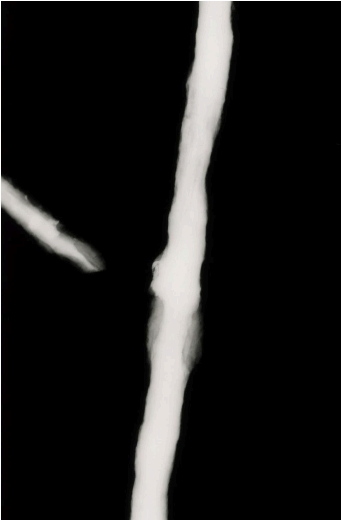
FIG 17A. X RADIOGRAPHY OF THE POINT B SWELLING SHOWS A "SPLINTER" OF IRON EXTANT ON THE SIDE OF THE SWELLING. THIS MAY REPRESENT THE REMAINS OF A FORGE-WELD MADE ON THE ADJACENT FACE OF THE SHAFT TO THE POINT B SWELLING WHICH HAS DETACHED CLOSER TO THE TOW OF THE WELD. COPYRIGHTS BY THE TRUSTEES OF THE BRITISH MUSEUM. SHARED UNDER A CREATIVE COMMONS ATTRIBUTION-NONCOMMERCIAL-SHAREALIKE 4.0 INTERNATIONAL (CC BY-NC-SA 4.0) LICENCE.
