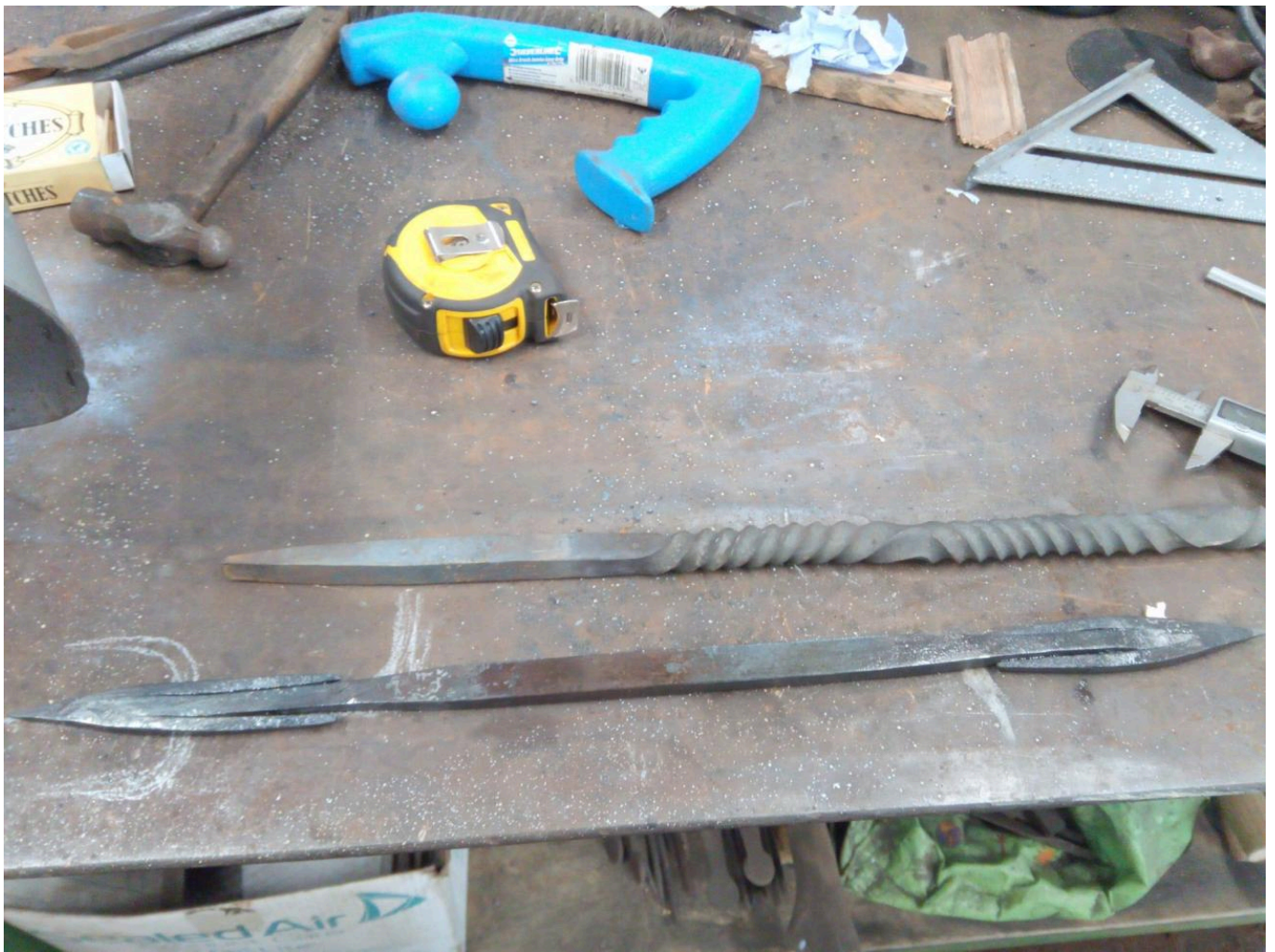
FIG 60A. A REPRODUCTION OF THE PRITTLEWELL STAND BY THE AUTHOR. THE UPPER SPIKE OF THIS OBJECT WAS CREATED USING THE METHOD SHOWN IN FIG 59. IMAGE SHOWS THE ADDITIONAL MATERIAL PREPARED FOR WELDING. COPYRIGHTS BY ROWAN TAYLOR.
