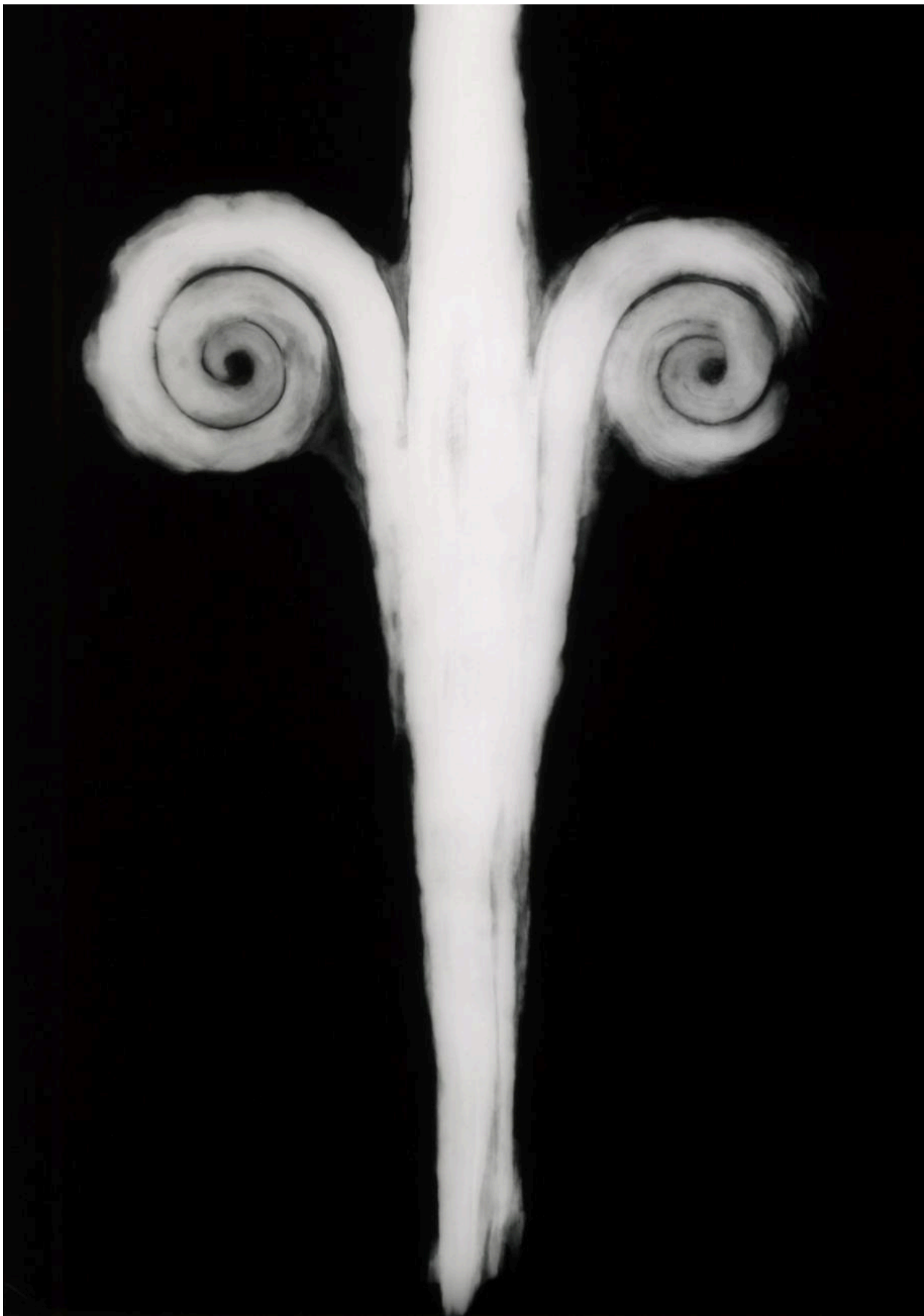
FIG 62A. A) FOR COMPARISON. B) THE GREEN LINES FOLLOW THE GRAIN OF THE SPIKE, WHICH BROADLY FOLLOWS PARALLEL TO THE EDGES OF THE TAPER. THIS IS A PART OF THE IRON AND SEPARATE FROM THE VOLUTE WELDS, WHICH WERE HIGHLIGHTED IN FIG 57.B. COPYRIGHTS BY THE TRUSTEES OF THE BRITISH MUSEUM. SHARED UNDER A CREATIVE COMMONS ATTRIBUTION-NONCOMMERCIAL-SHAREALIKE 4.0 INTERNATIONAL (CC BY-NC-SA 4.0) LICENCE.
