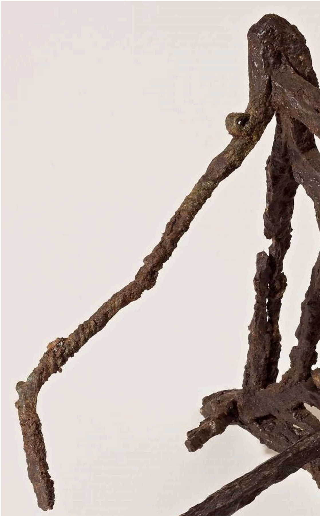
FIG 34. PHOTOGRAPHY OF STRUT R REVEALS COPPER-ALLOY CORROSION STILL EXTANT ON THE STRUCTURE. COPYRIGHTS BY THE TRUSTEES OF THE BRITISH MUSEUM. SHARED UNDER A CREATIVE COMMONS ATTRIBUTION-NONCOMMERCIAL-SHAREALIKE 4.0 INTERNATIONAL (CC BY-NC-SA 4.0) LICENCE.
