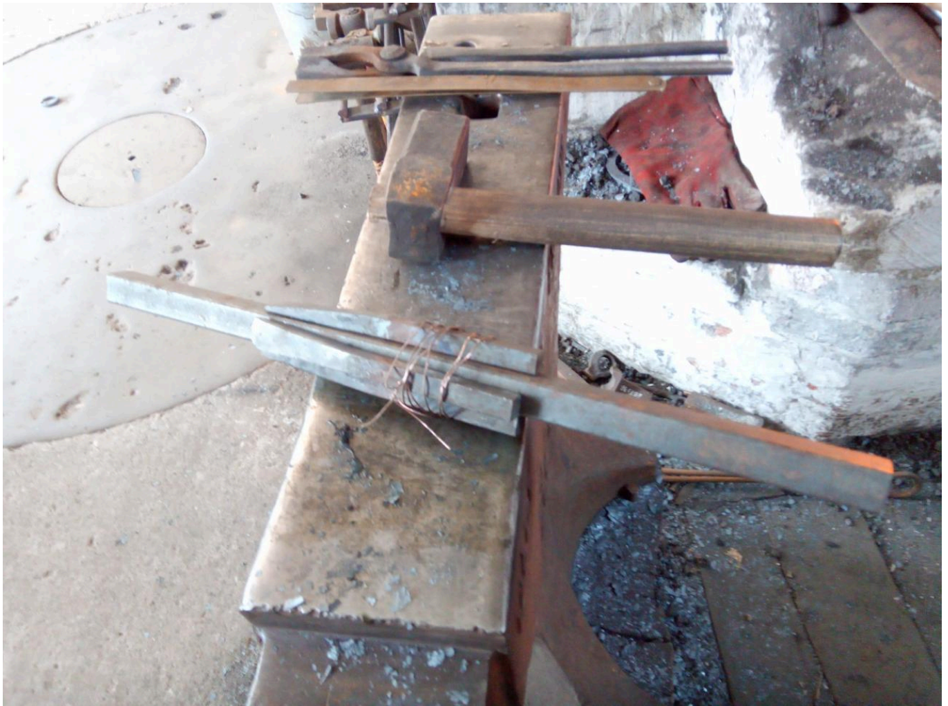
FIG 18.A. IN ORDER TO EXPLORE THE NOTION THAT THE POINT B SWELLING REPRESENTS THE FIREWELDED BASE OF THE UPPER-BASKET STRUTS, FOUR "STRUTS" WERE SCARFED AND PREPARED FOR WELDING TO A "SHAFT". HERE THEY ARE WIRED INTO POSITION. A MORE PERIOD-ACCURATE MANNER OF DOING THIS COULD HAVE BEEN TO COLLAR THEM WITH A SHORT LENGTH OF FLAT STOCK, WELD THEM INDIVIDUALLY, OR TIE THEM WITH DAMP CORDAGE/THONGING HIGHER UP THE SHAFT. COPYRIGHTS BY ROWAN TAYLOR.
