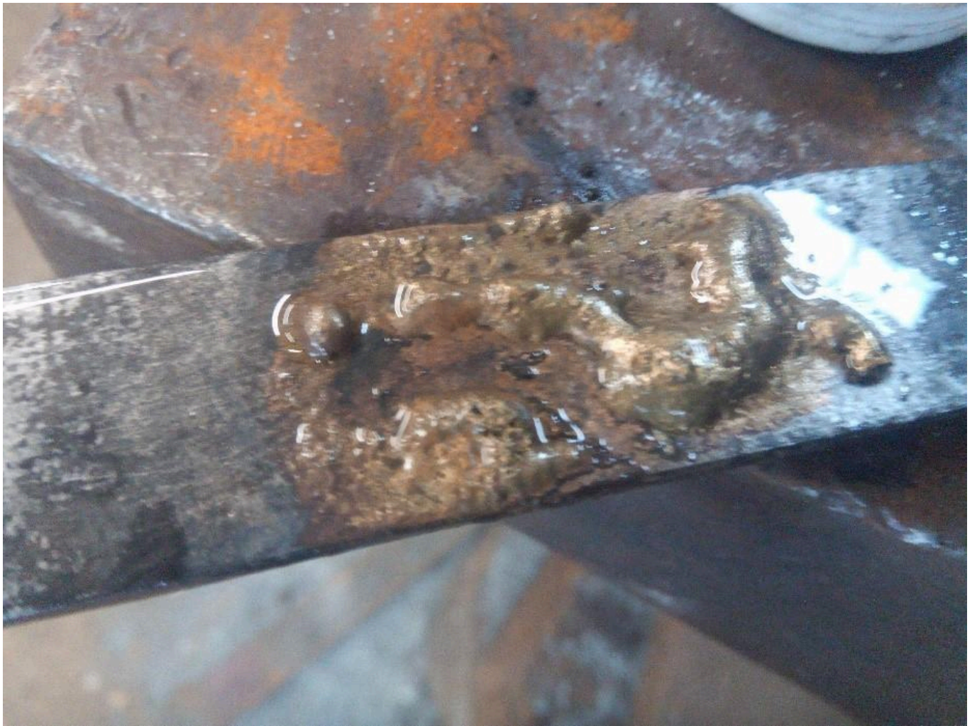
FIG 41. TEST CONDUCTED USING THEOPHILUS'S RECIPE. THE USE OF EXCESSIVE AMOUNTS OF COPPER-ALLOY (BRASS IN THIS CASE) RESULTS IN A GLOBULAR COATING. COPYRIGHTS BY ROWAN TAYLOR.
