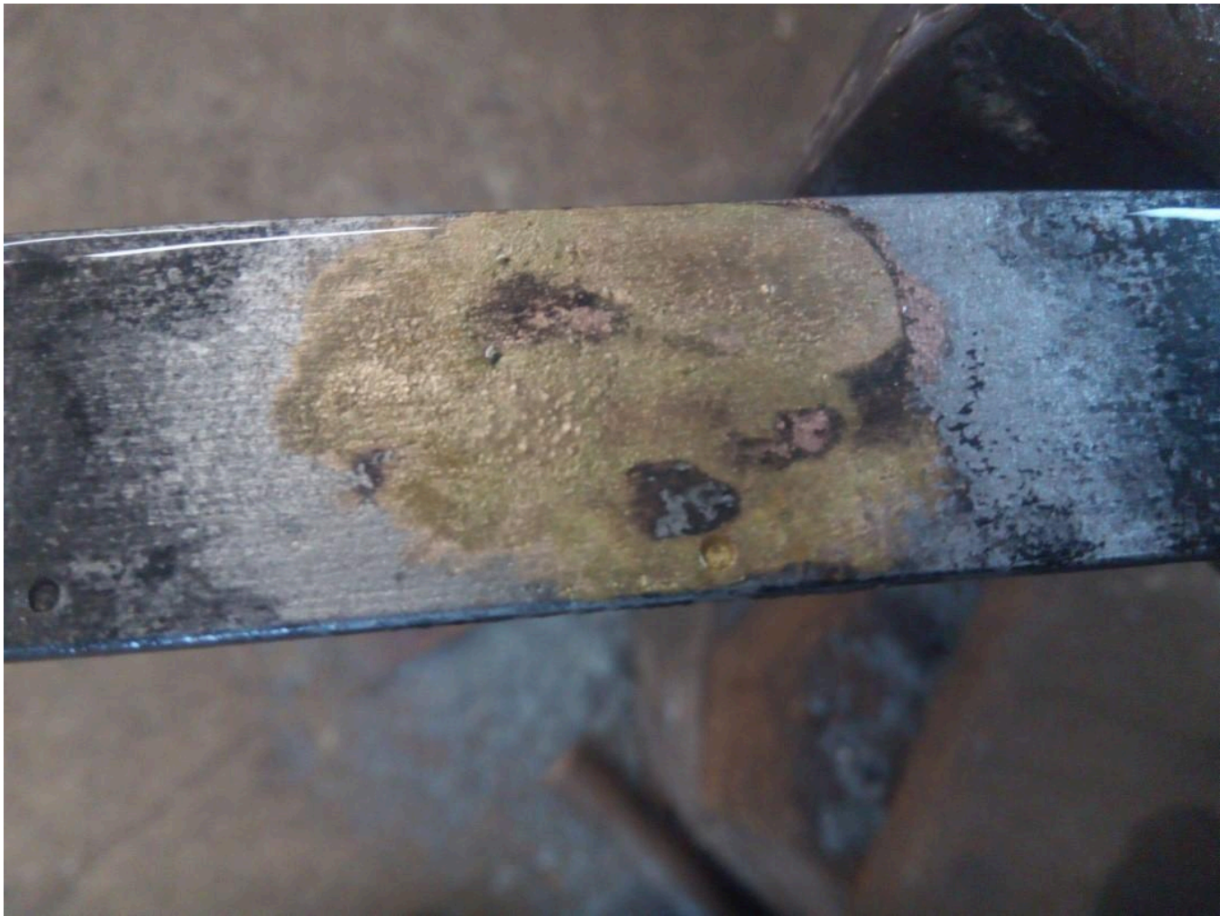
FIG 40. TEST CONDUCTED USING THEOPHILUS'S RECIPE. FOLLOWING THE LATTER'S INSTRUCTIONS RESULTS IN A THIN, EVEN PLATING OF COPPER-ALLOY. BRASS WAS USED FOR THIS TEST. SOME AREAS OF DE-ZINCIFICATION ARE VISIBLE AS A RESULT OF OVER-HEATING. SOME IMPURITIES AND POROSITY ARE ALSO VISIBLE. NOTE THE REMOVAL OF OXIDES AND FIRE-SCALE FROM THE STEEL BASE. COPYRIGHTS BY ROWAN TAYLOR.
