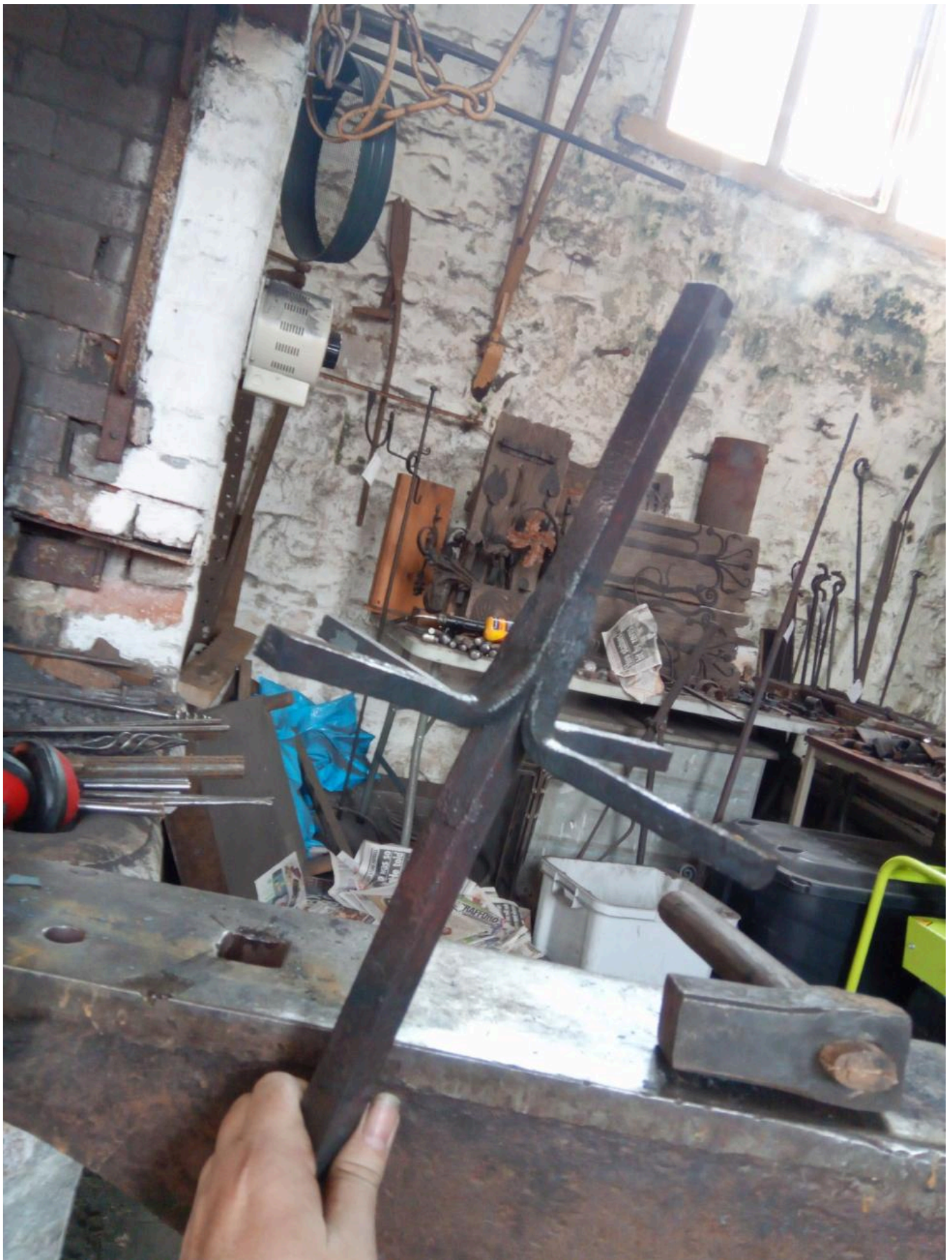
FIG 18C. THE "STRUTS" ARE UNFURLED UPWARDS. BASED ON THE POINT B SWELLING AND THE POSITION OF THE STEP BEING POSITIONED LOWER THAN THE TOE, IT IS LIKELY THAT THE STRUTS FACED DOWN THE SHAFT IN THIS MANNER AND WERE THEN BENT UPWARDS. COPYRIGHTS BY ROWAN TAYLOR.
