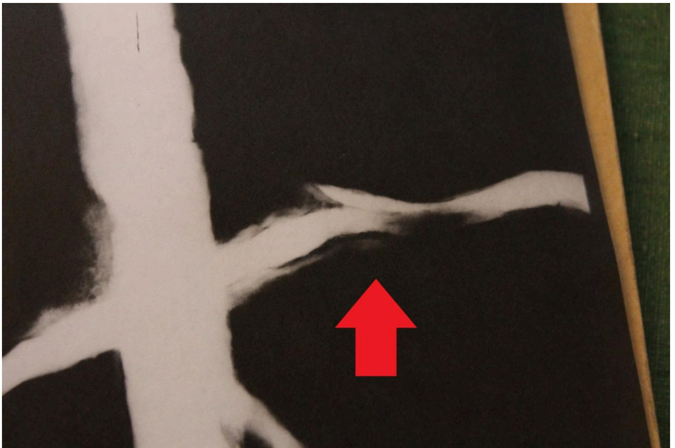
FIG 31A. X RADIOGRAPHY OF THE POINT A ELEMENT. THE RED ARROW HIGHLIGHTS THE PRESENCE OF A SCARF OR LAP WELD BY WHICH ONE OF THE STRUTS HAS BEEN ATTACHED TO THE ELEMENT. THE WELD IS BECOMING DETACHED, LIKELY DUE TO A COMBINATION OF CORROSION AND A SLIGHTLY COLD WELD RESULTING IN A COLD-SHUT. COPYRIGHTS BY THE TRUSTEES OF THE BRITISH MUSEUM. SHARED UNDER A CREATIVE COMMONS ATTRIBUTION-NONCOMMERCIAL-SHAREALIKE 4.0 INTERNATIONAL (CC BY-NC-SA 4.0) LICENCE.
