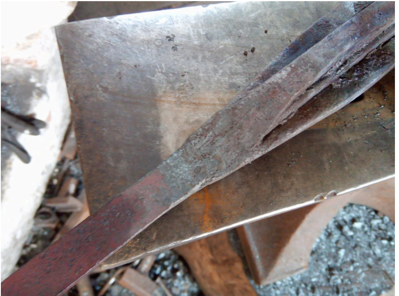
FIG 18B. THE FOUR "STRUTS" HAMMER WELDED INTO POSITION. COPYRIGHTS BY ROWAN TAYLOR.
