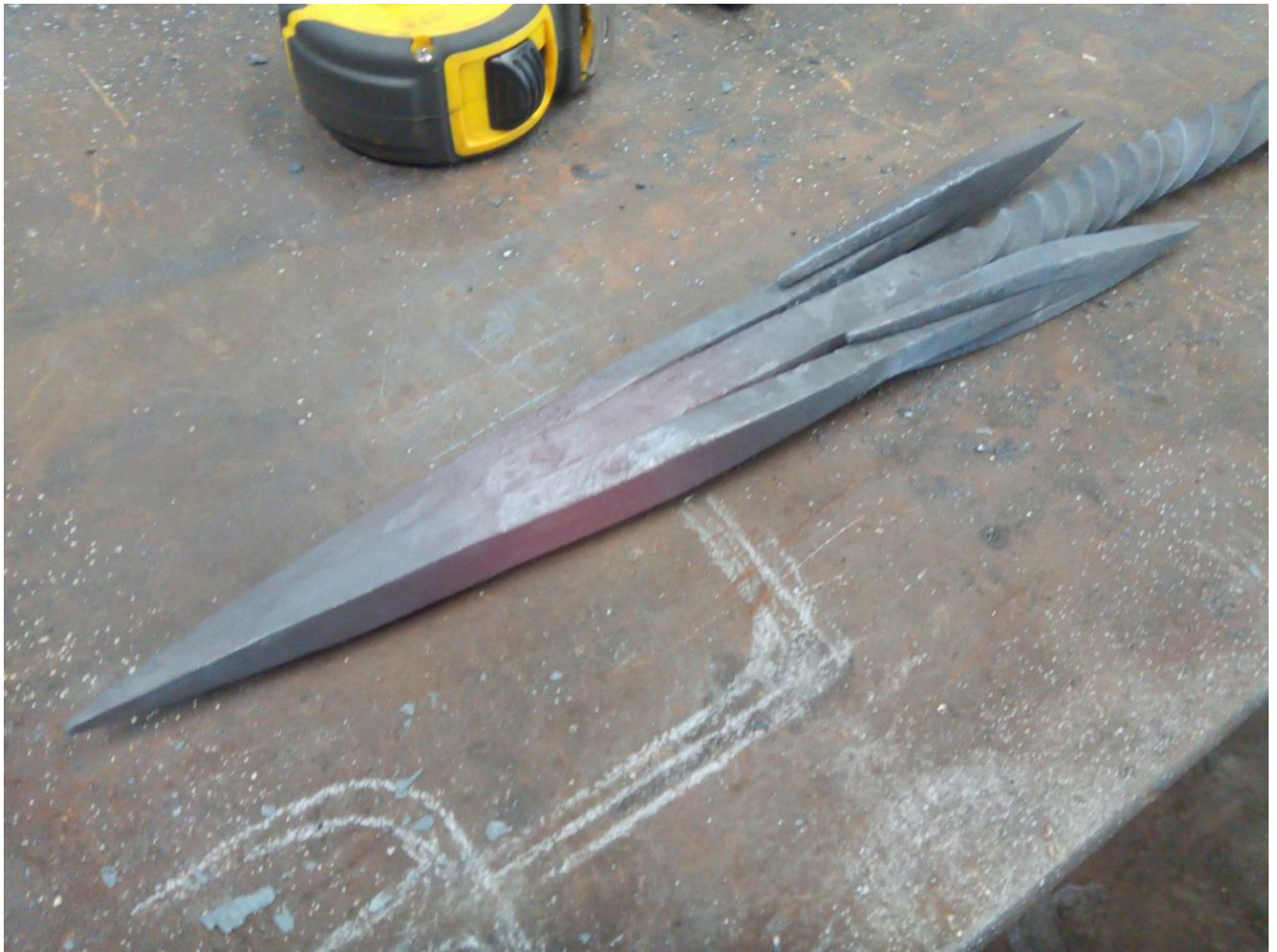
FIG 60B. A REPRODUCTION OF THE PRITTLEWELL STAND BY THE AUTHOR. THE UPPER SPIKE OF THIS OBJECT WAS CREATED USING THE METHOD SHOWN IN FIG 59. IMAGE SHOWS THE UPPER SPIKE WELDED PRIOR TO FORMING. COPYRIGHTS BY ROWAN TAYLOR.
