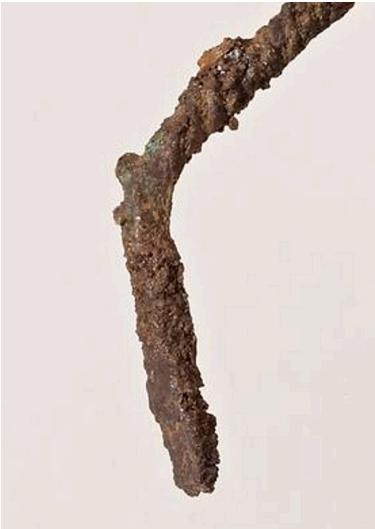
FIG 44B. PHOTOGRAPHY OF THE STRUT R LOWER "ELBOW" SHOWS THE REMAINS OF THE PRESUMED RING ALONG WITH COPPER-ALLOY OXIDES STILL CLEARLY PRESENT ON THE SURFACE. COPYRIGHTS BY THE TRUSTEES OF THE BRITISH MUSEUM. SHARED UNDER A CREATIVE COMMONS ATTRIBUTION-NONCOMMERCIAL-SHAREALIKE 4.0 INTERNATIONAL (CC BY-NC-SA 4.0) LICENCE.
