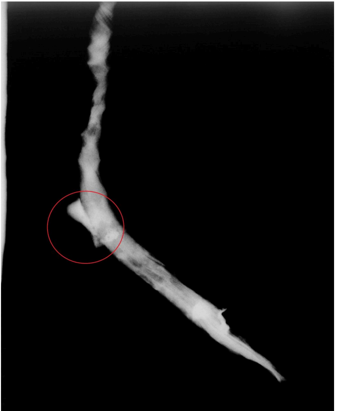
FIG 44A. X-RADIOGRAPHY OF STRUT R. THE "ELBOW" AT THE LOWER END OF THE STRUT PRESENTS THE REMAINS OF WHAT MAY BE A BRAZED RING ON ITS OUTER CORNER (RED CIRCLE). COPYRIGHTS BY THE TRUSTEES OF THE BRITISH MUSEUM. SHARED UNDER A CREATIVE COMMONS ATTRIBUTION-NONCOMMERCIAL-SHAREALIKE 4.0 INTERNATIONAL (CC BY-NC-SA 4.0) LICENCE.
