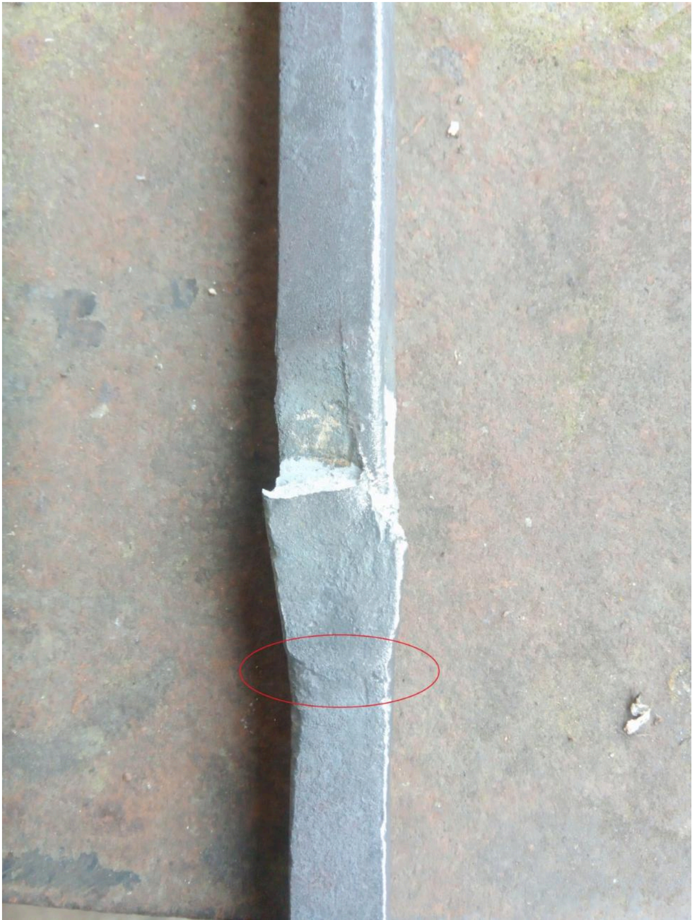
FIG 14B. AN EXPERIMENTAL RECREATION OF THE POINT B SWELLING (OUTLINED FURTHER-ON IN THIS DOCUMENT) HAS ALSO RESULTED IN THE PRESENCE OF A TOE AT THE BASE OF THE WELD. COPYRIGHTS BY ROWAN TAYLOR.
