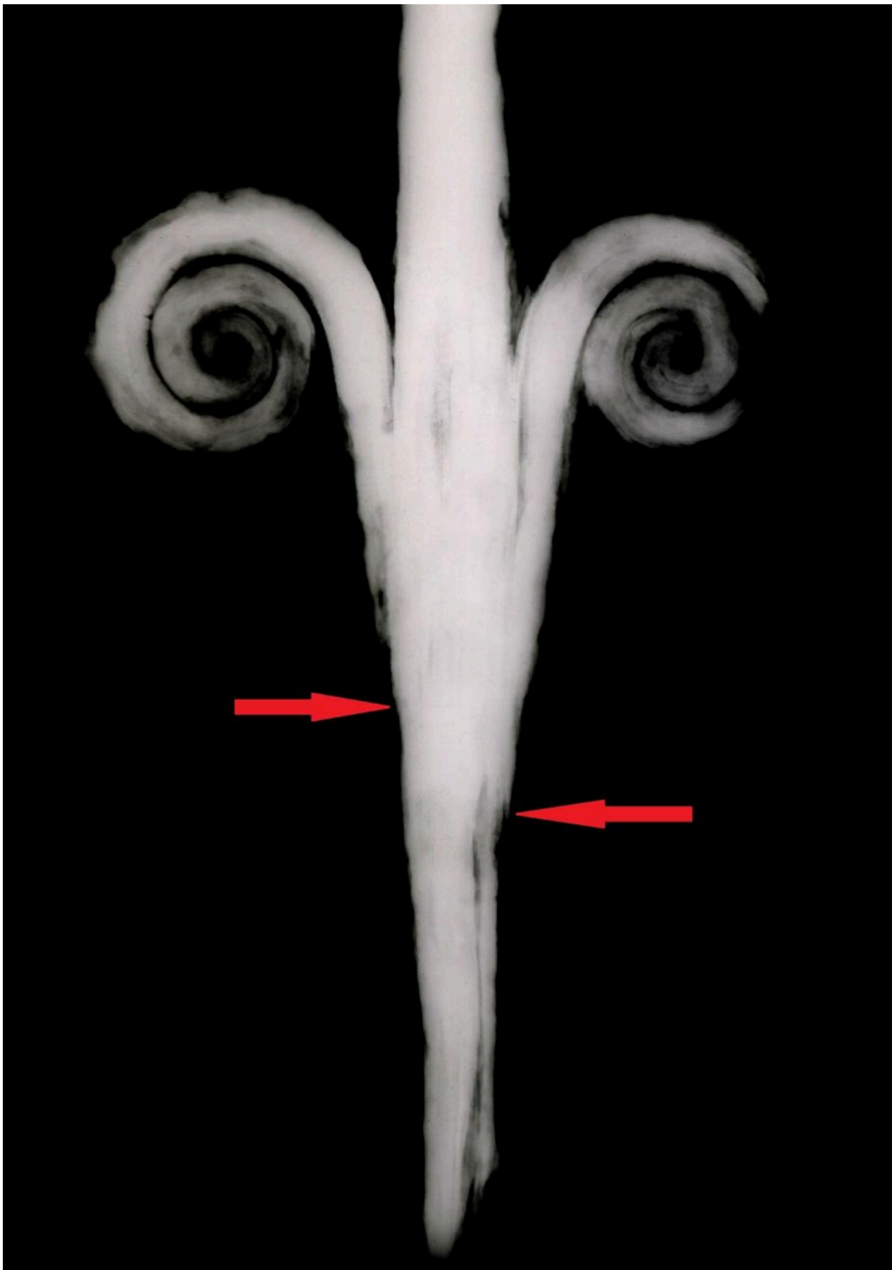
FIG 57A. THE SAME X-RADIOGRAPHY OF THE BASE OF THE STAND, WITH THE CONTRAST ENHANCED SO AS TO BETTER SHOW CONSTRUCTIONAL LINES WITHIN THE IRONWORK. THE RED-ARROWS SHOW THE TOES OF THE WELDS FOR EACH VOLUTE. COPYRIGHTS BY THE TRUSTEES OF THE BRITISH MUSEUM. SHARED UNDER A CREATIVE COMMONS ATTRIBUTION-NONCOMMERCIAL-SHAREALIKE 4.0 INTERNATIONAL (CC BY-NC-SA 4.0) LICENCE.
