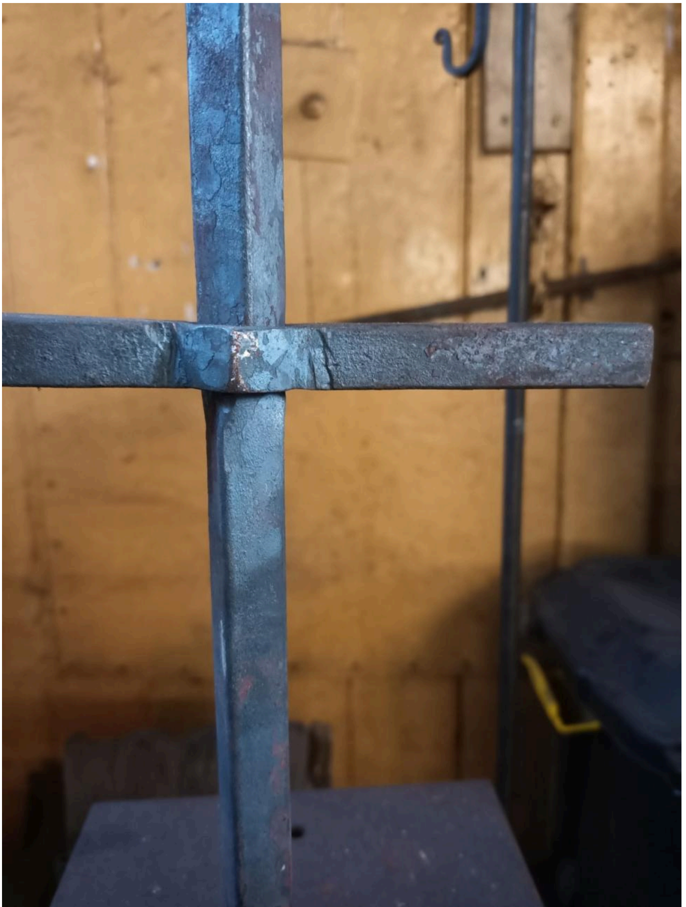
FIG 28B. PRACTICAL DEMONSTRATION OF A TWIST BEING USED TO FORM A STEP IN A SHAFT. THIS PRODUCES AN IMPEDANCE ON THE SHAFT SUFFICIENT TO THE RETENTION OF A PASS-THROUGH FIXING. ADDITIONALLY, THE SHAFT APPEARS EITHER BROADER ABOVE OR BELOW THE TWIST DEPENDING ON WHERE THE VIEWER STANDS. COPYRIGHTS BY ROWAN TAYLOR.
