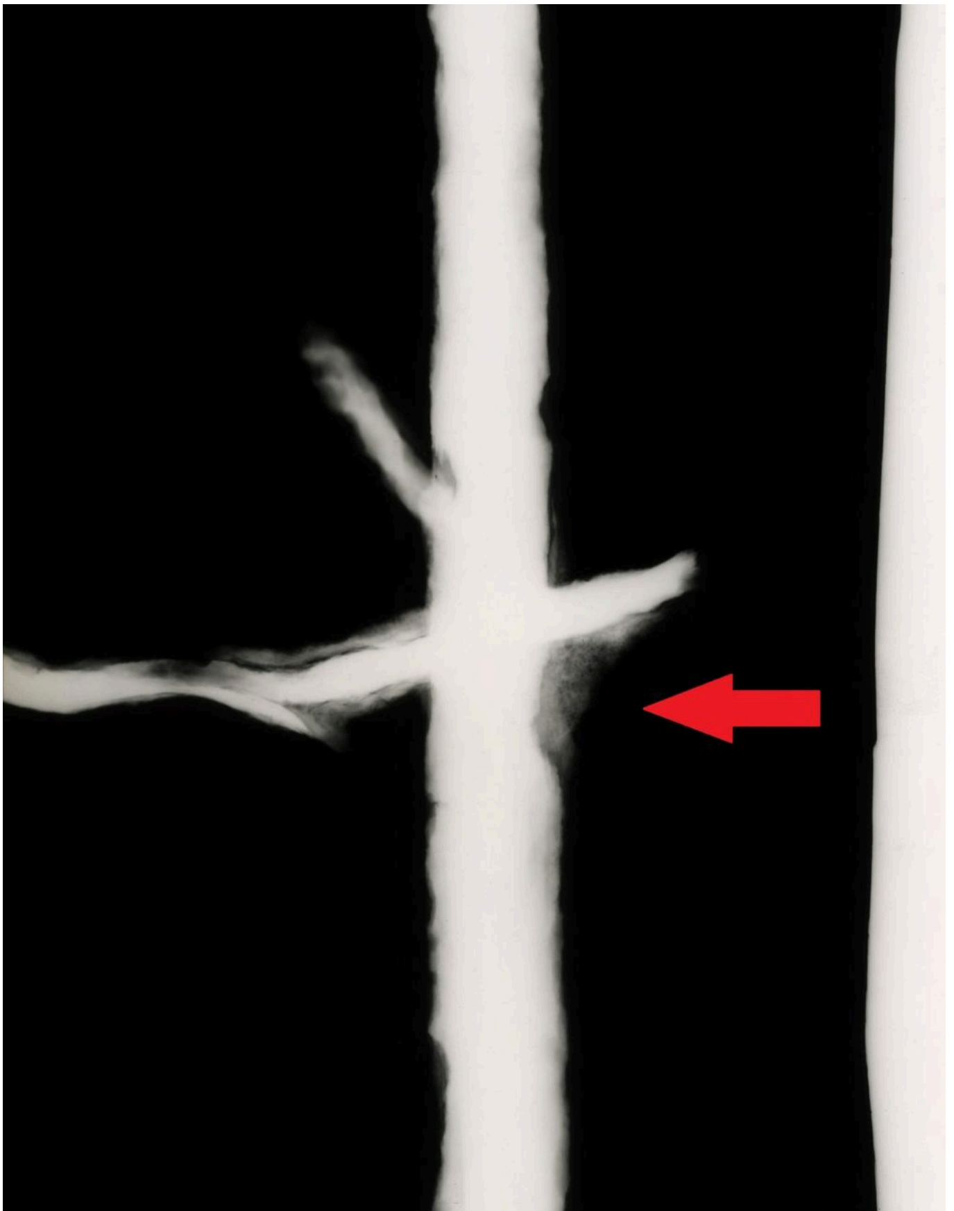
FIG 22. SIMILAR POSSIBLE FOOTING CORROSION (RED ARROW) IS VISIBLE BELOW THE PLATE AT POINT A. COPYRIGHTS BY THE TRUSTEES OF THE BRITISH MUSEUM. SHARED UNDER A CREATIVE COMMONS ATTRIBUTION-NONCOMMERCIAL-SHAREALIKE 4.0 INTERNATIONAL (CC BY-NC-SA 4.0) LICENCE.
