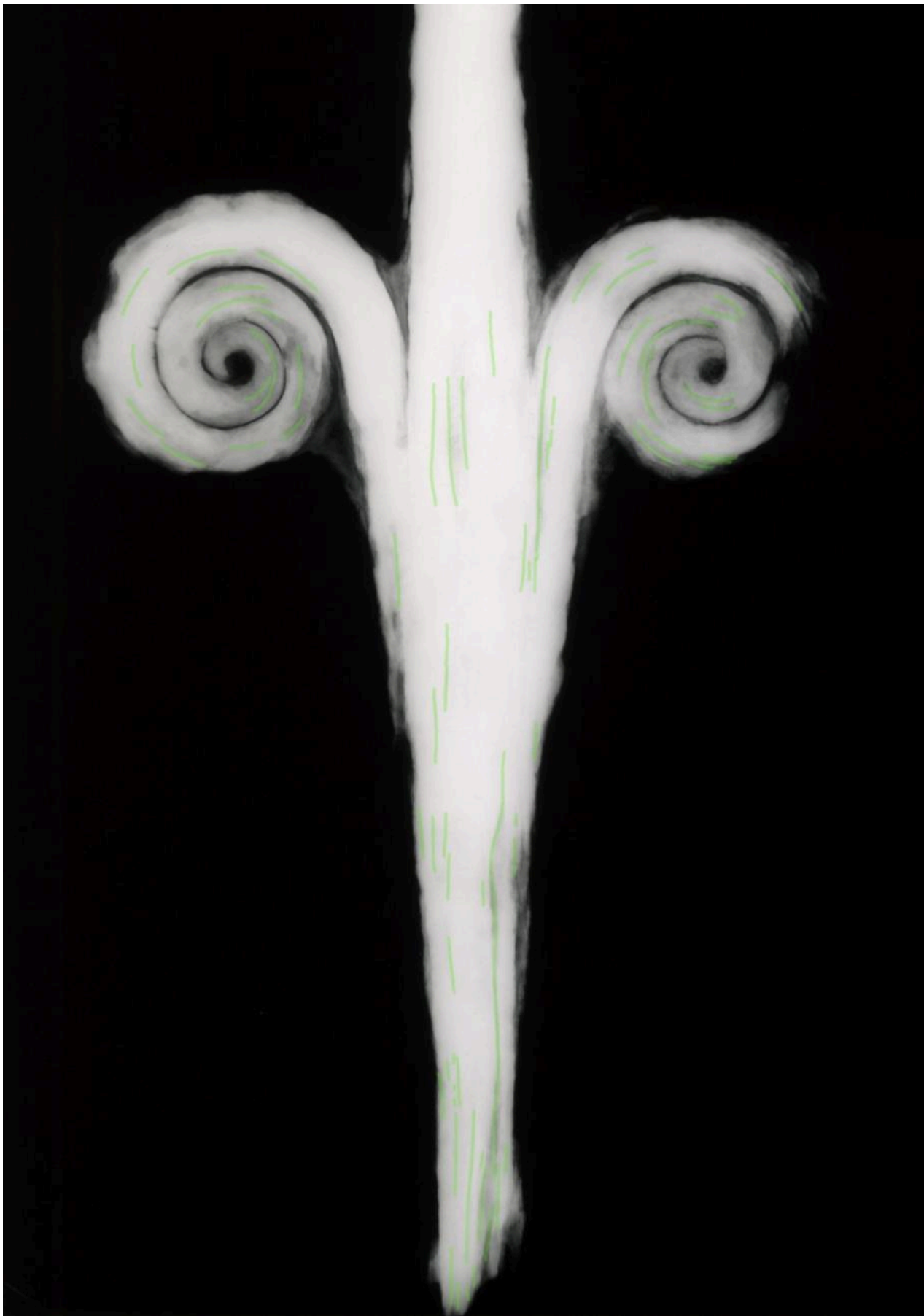
FIG 62B. A) FOR COMPARISON. B) THE GREEN LINES FOLLOW THE GRAIN OF THE SPIKE, WHICH BROADLY FOLLOWS PARALLEL TO THE EDGES OF THE TAPER. THIS IS A PART OF THE IRON AND SEPARATE FROM THE VOLUTE WELDS, WHICH WERE HIGHLIGHTED IN FIG 57.B. COPYRIGHTS BY THE TRUSTEES OF THE BRITISH MUSEUM. SHARED UNDER A CREATIVE COMMONS ATTRIBUTION-NONCOMMERCIAL-SHAREALIKE 4.0 INTERNATIONAL (CC BY-NC-SA 4.0) LICENCE.
