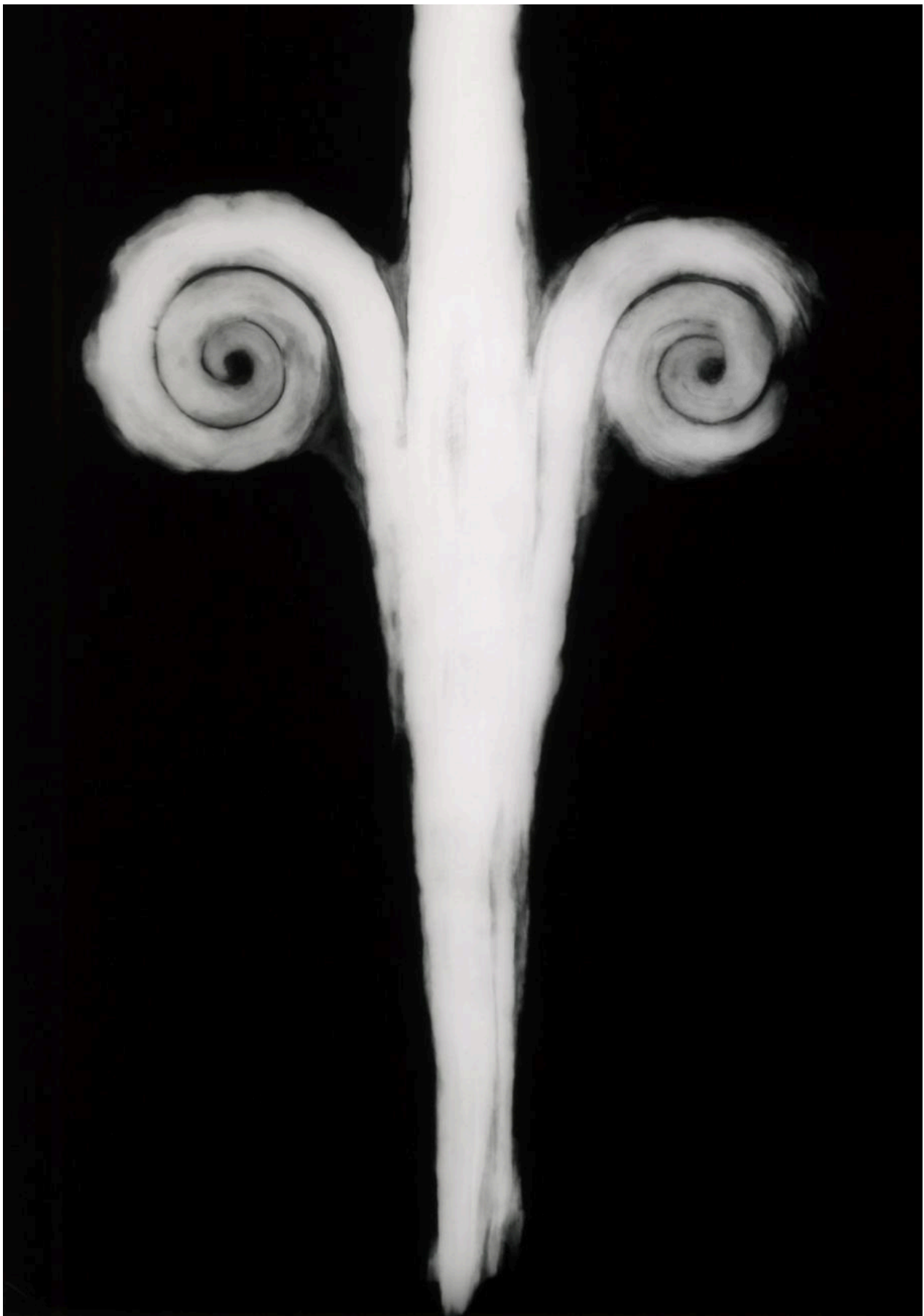
FIG 55. X-RADIOGRAPHY OF THE BASE OF THE STAND SHOWS THAT THE VOLUTES ARE CLOSED SCROLLS, FORMED FROM A THICK SECTION OF IRON, AS OPPOSED TO THE THIN, OPEN SCROLLS CURRENTLY REPRESENTED. COPYRIGHTS BY THE TRUSTEES OF THE BRITISH MUSEUM. SHARED UNDER A CREATIVE COMMONS ATTRIBUTION-NONCOMMERCIAL-SHAREALIKE 4.0 INTERNATIONAL (CC BY-NC-SA 4.0) LICENCE.
