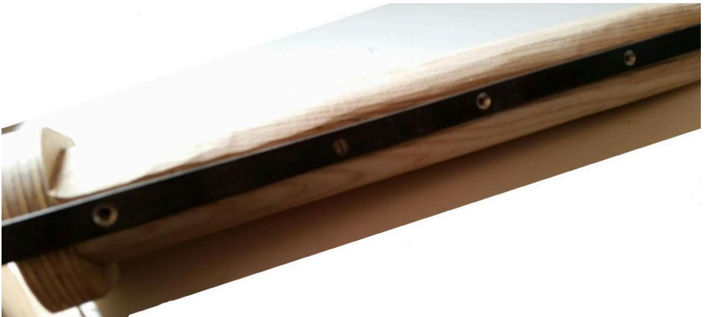
FIG 10. HOLES PUNCHED FOR THE NAILS TO SECURE THE THIGH SUPPORT TO THE PEG. COPYRIGHT: C. WALLER-COTTERHILL
