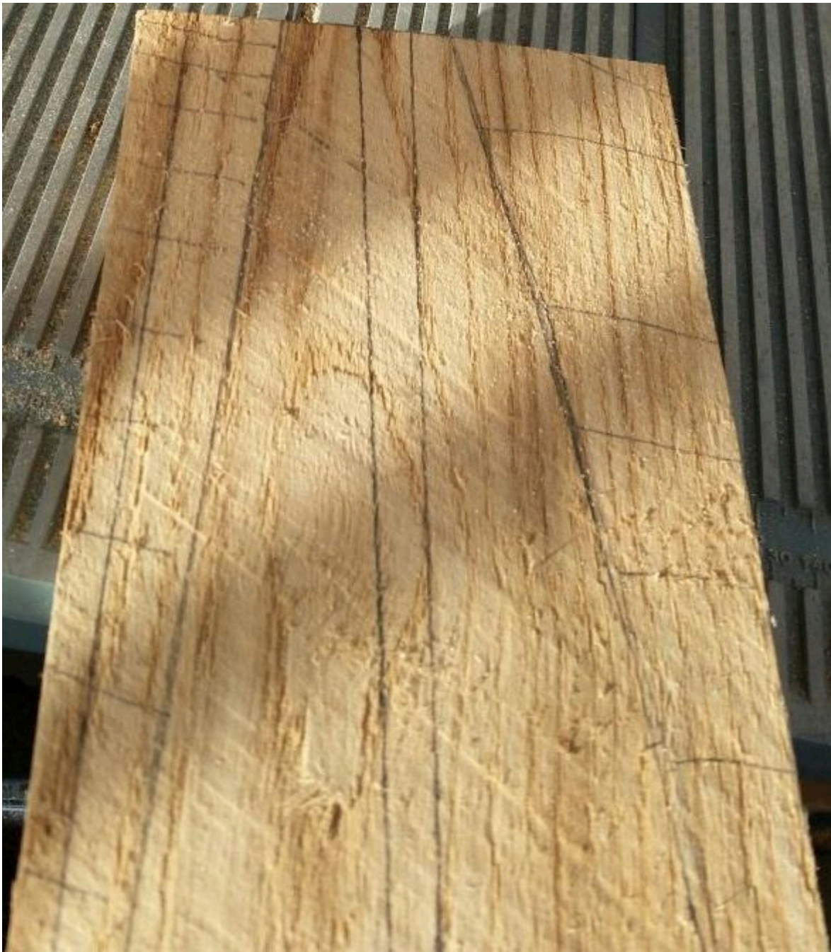
FIG 4. A RULER AND PENCIL WERE USED TO MARK OUT THE AREAS, WHICH WOULD BE CUT TO SIZE. COPYRIGHT: C. WALLER-COTTERHILL
