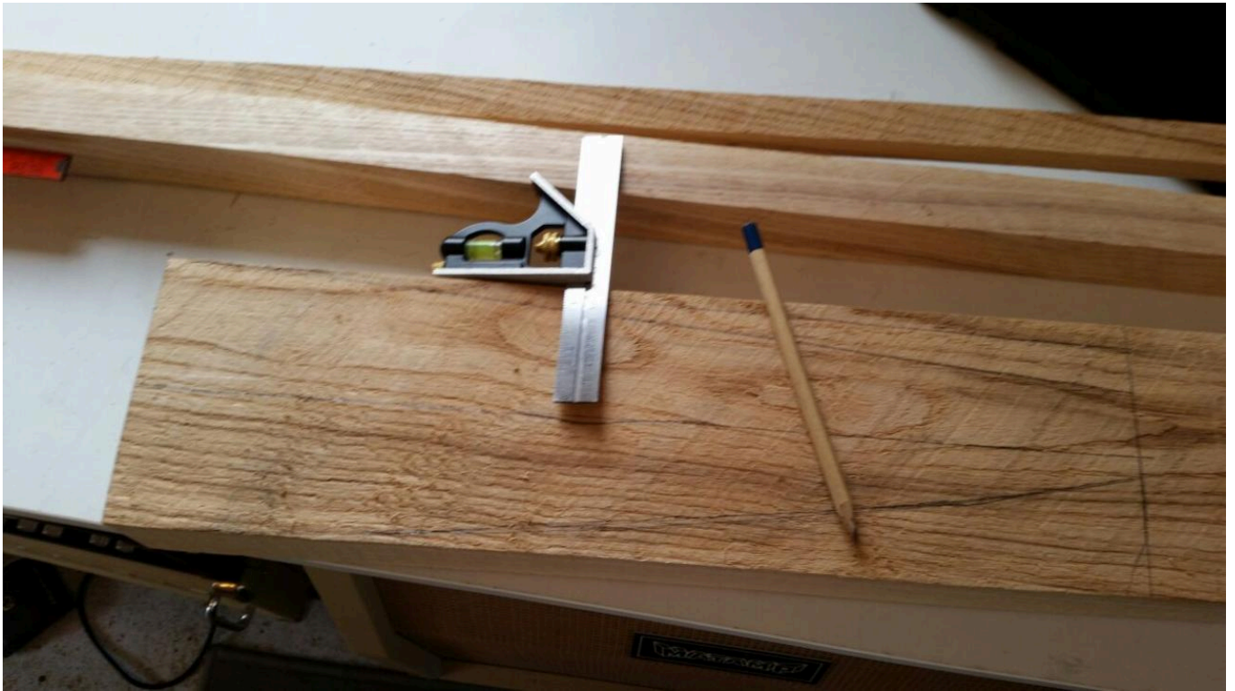
FIG 3. A RULER AND PENCIL WERE USED TO MARK OUT THE AREAS, WHICH WOULD BE CUT TO SIZE. COPYRIGHT: C. WALLER-COTTERHILL
