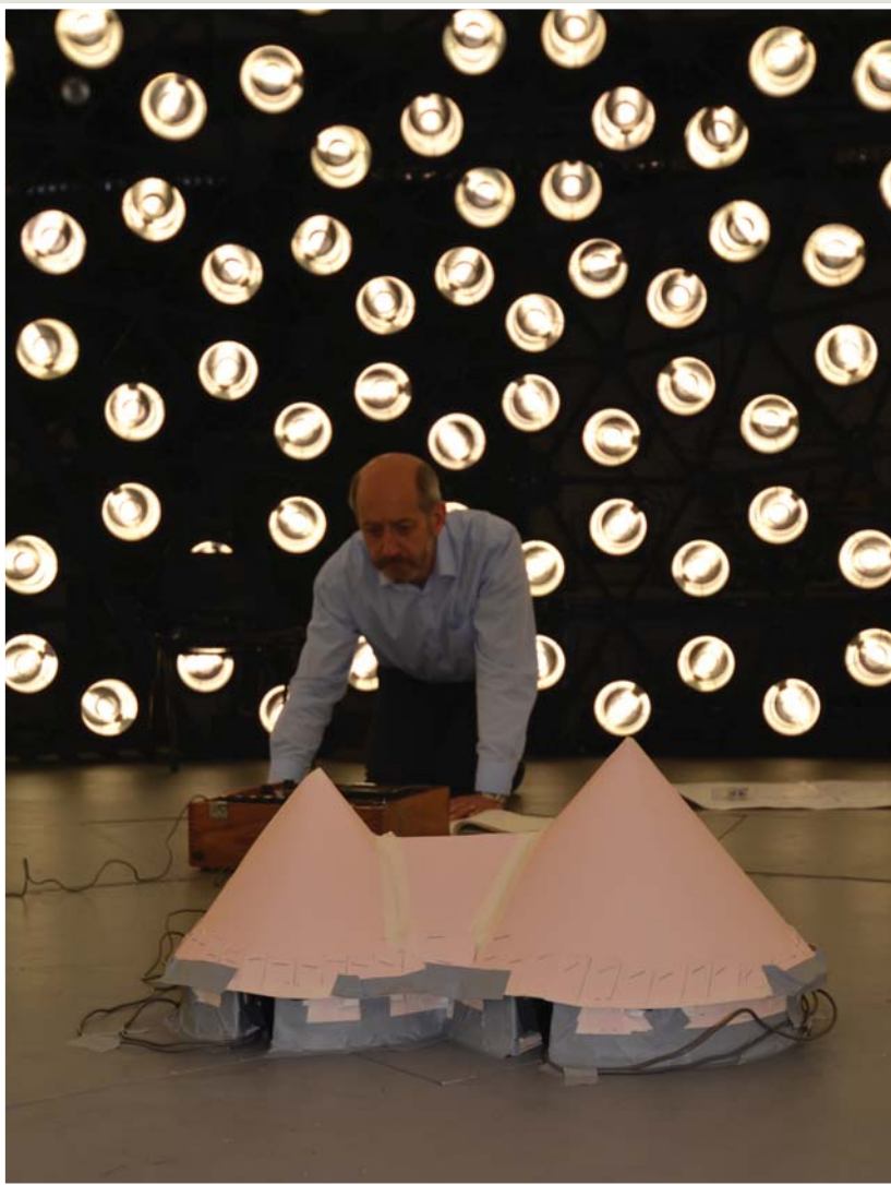
Fig 9. (Above) Testing the light levels that could be expected inside the Iron Age farmstead inside the artificial sky facility at Cardiff School of Architecture, 2012.
