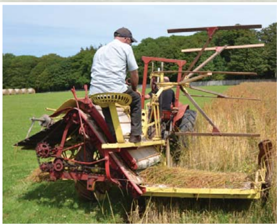
Fig 10. (Above) The 1940s reaper-binder harvesting the spelt crop in July 2014.
