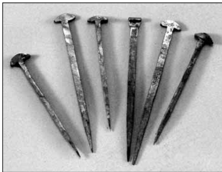
Fig. 9 Replicas of nails used in the roof construction of the building B7. ■
