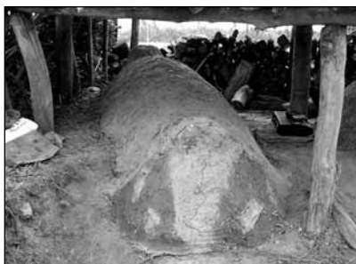
Fig. 23 Kiln closed after firing to create a reducing atmosphere. ■
