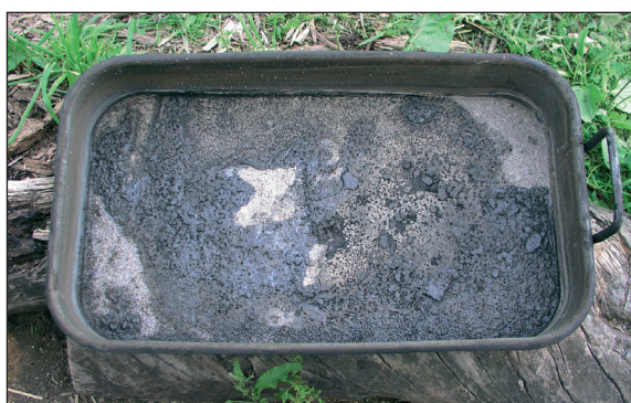
■ Fig. 10 After evaporation a thin layer of lye stays on the bottom.
