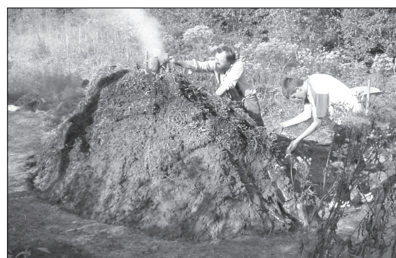
■ Fig. 2 Production of charcoal: a Building of a clamp – wood is stacked vertically in layers; b, c Covering of the clamp with turf and igniting it from the top. (photo M. Cvejn)
