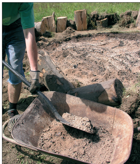
■ Fig. 6 Potash production: Beech ashes are collected after cooling down.
