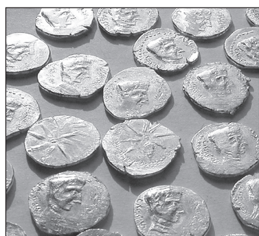
■ Fig. 15 Hot striking produced these pure silver coins
