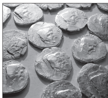
■ Fig. 14 Cold striking produced these pure silver coins.
