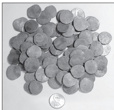
■ Fig. 7 Debased coin blanks after vinegar treatment.*
