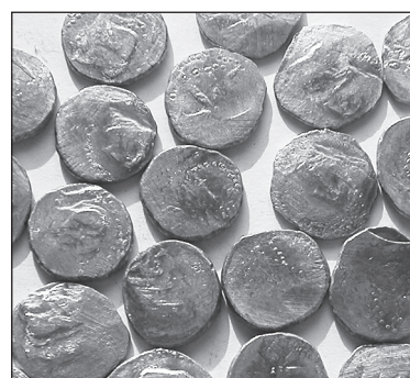
■ Fig. 16 Cold striking produced these debased silver coins.
