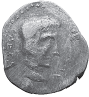
■ Fig. 24 Hot-struck debased coin after prolonged vinegar soak.
