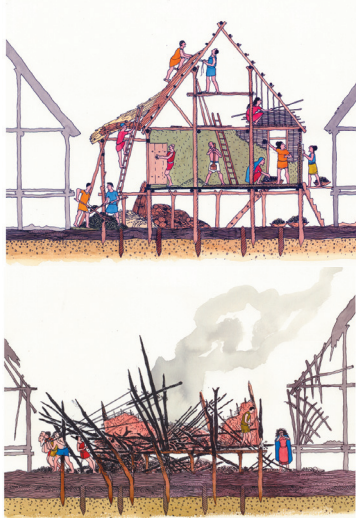
■ Fig. 4 Construction and destruction of houses in phase II
