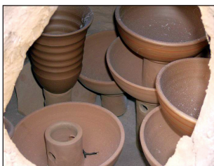
■ Fig. 13 Use of stilts in the small kiln (5th firing test, May 2009)
