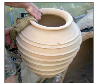
■ Fig. 14 Pot being removed during ‘hot’ opening of the big kiln (6th firing test, July 2009)
