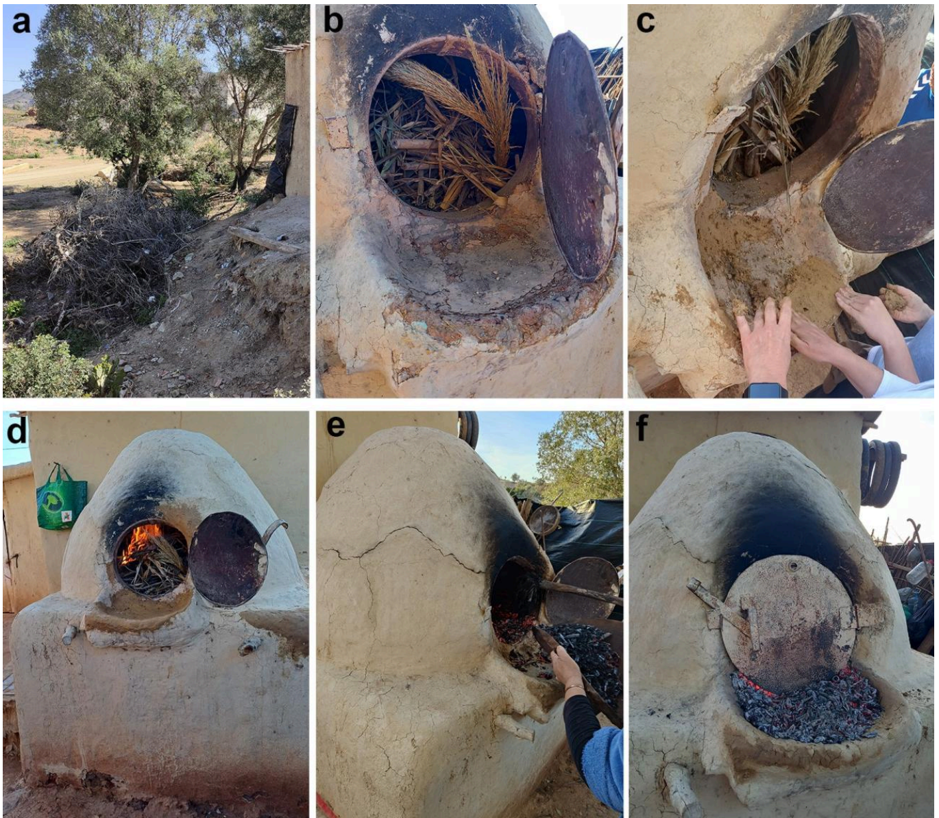
FIG 7. STORAGE (A) AND ADDITION OF FUEL (B). QUICK REPAIR OF THE OVEN (C) BEFORE IT IS PUT INTO USE (D). REDUCTION OF THE FUEL TO EMBERS AND ITS EXTRACTION IN THE LEDGE (E AND F). PHOTOS BY THE AUTHORS.
