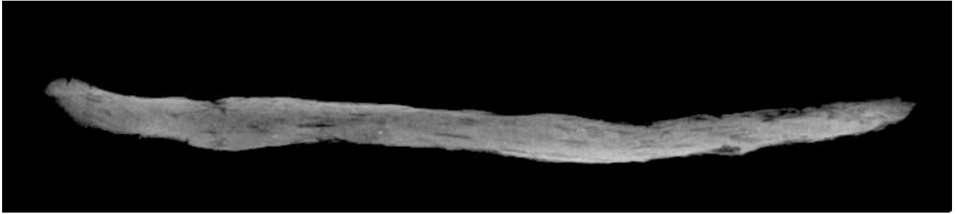
FIG 15. SIMPLE TABLET (METHOD 1.4). CLAY WITH THE STRAW TEMPER. MADE BY MANUALLY FORMING A CLAY COIL AND THEN PRESSING THIS DOWN WITH THE PALM OF ONE'S HAND INTO A FLAT TABLET SHAPE. SIDE X-RAY VIEW. PHOTO BY INA BERG.
