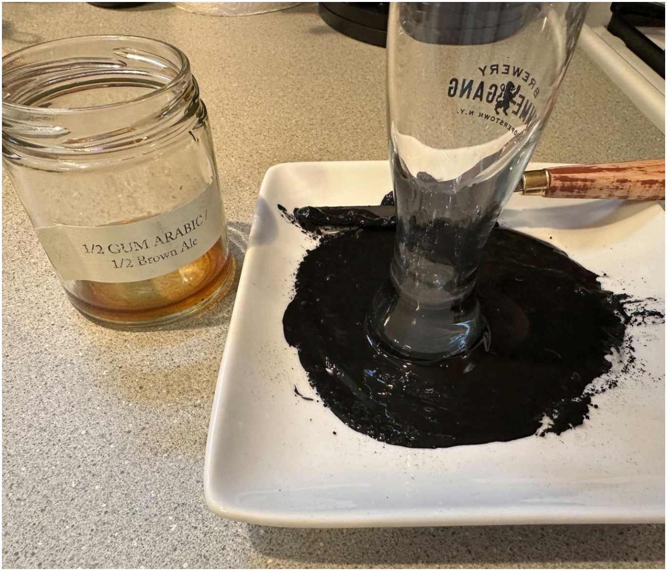
FIG 7. MULLING THE BLACK COATING USING A SIMULATED MULLER. PHOTO BY LAUREN MUNNEY.
