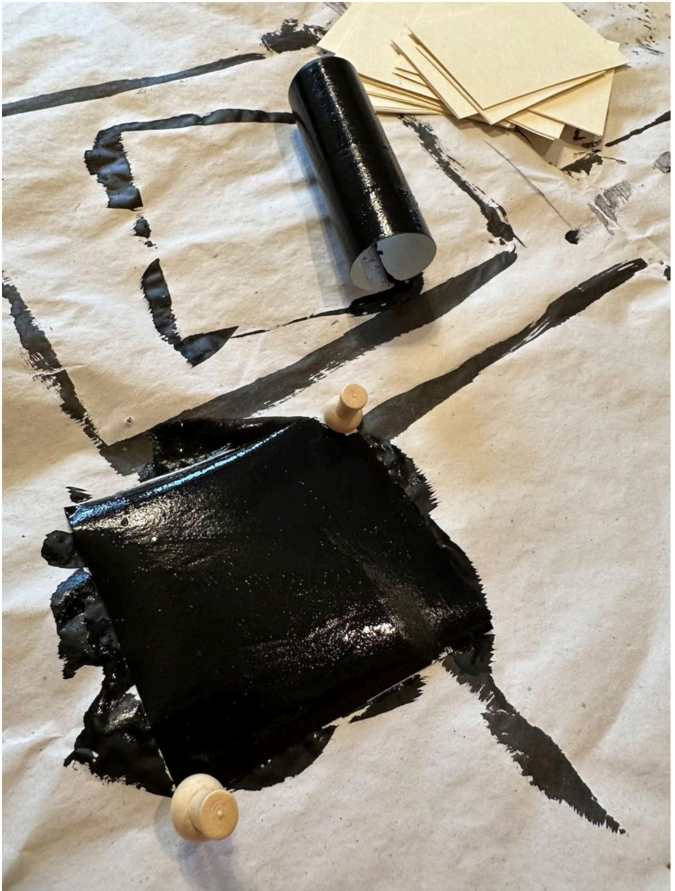
FIG 8. COATING THE PAPER, USING THE LOOSE METHOD (ABOVE) AND THE PINNING METHOD (BELOW). PHOTO BY LAUREN MUNNEY.
