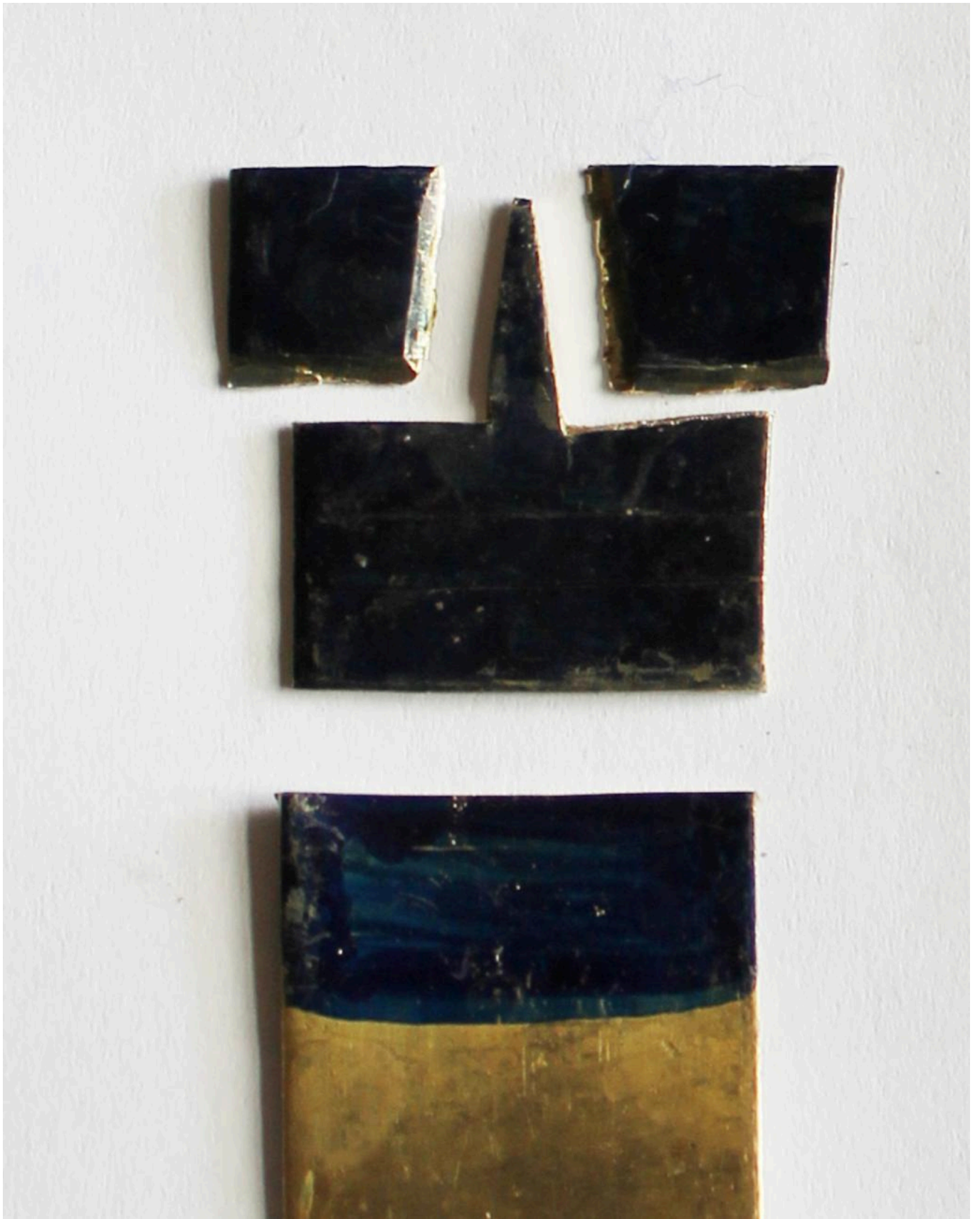
FIG 6. BLANK CUT FROM PARENT BAR. PHOTO BY DAVID SIM
