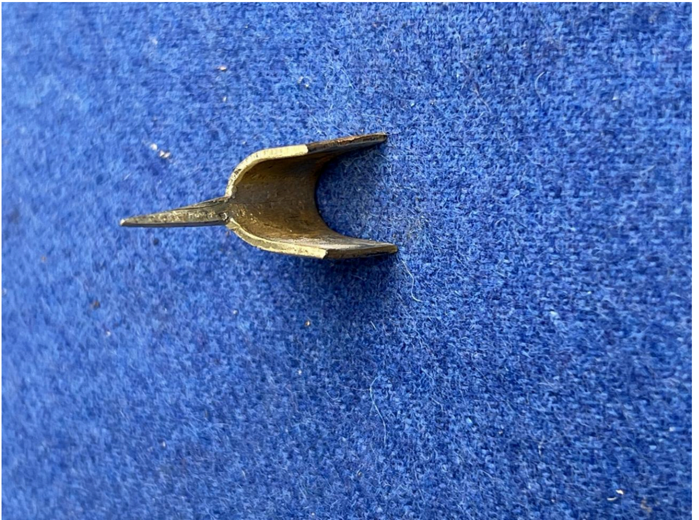
FIG 7. BLANK BENT TO U SHAPE (ENLARGED VIEW). PHOTO BY DAVID SIM
