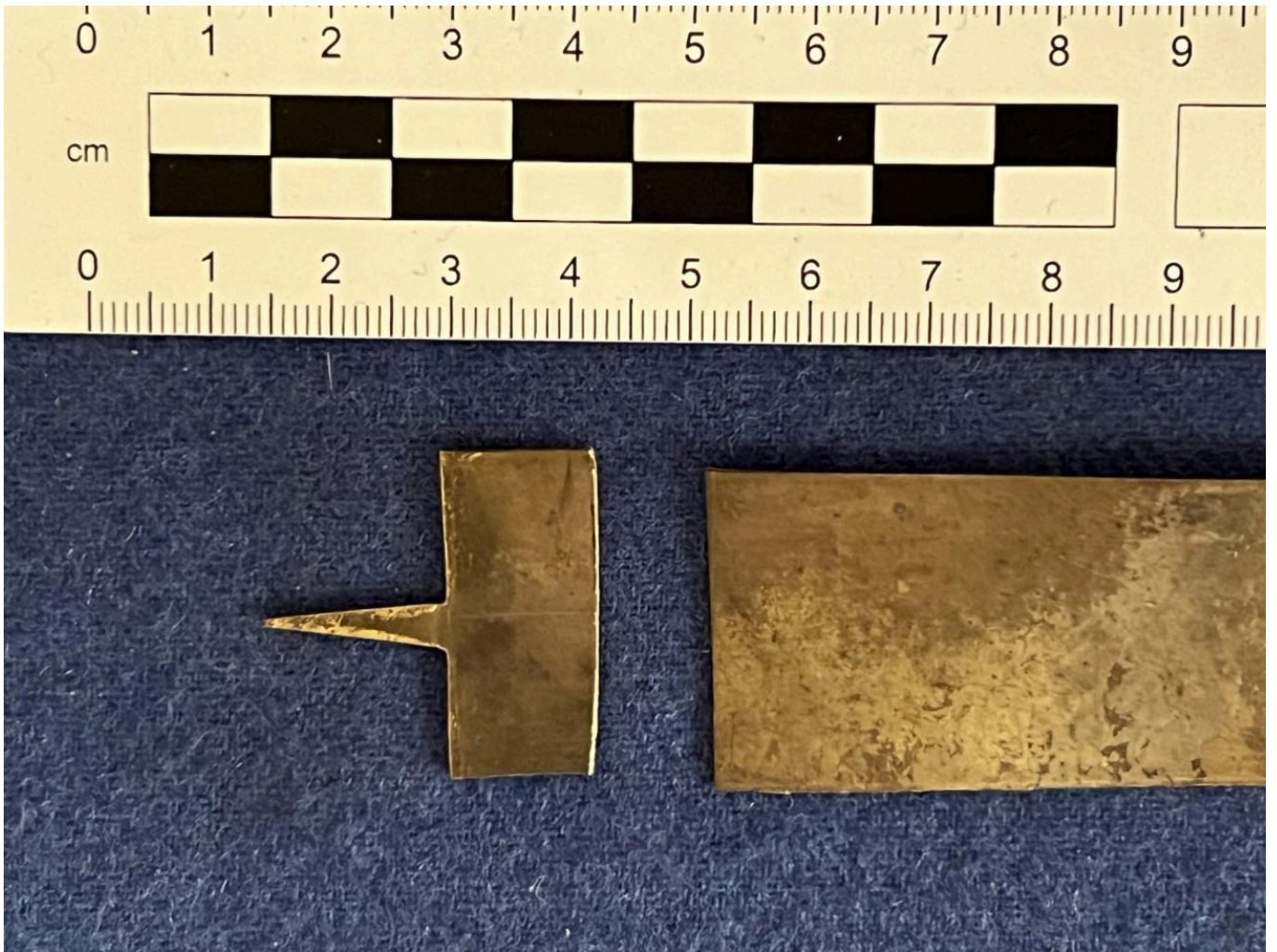
FIG 12. TEMPLATE FOR MARKING OUT NIB. PHOTO BY DAVID SIM
