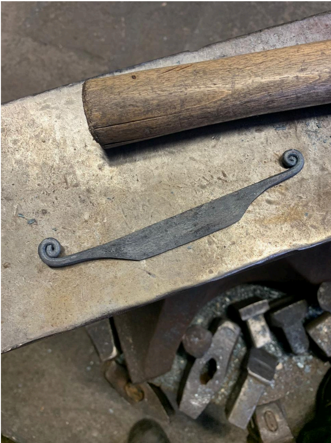
FIG 9. THE IRON FIBULA IS FORGED AGAINST THE ANVIL HORN AND CORNER BY THE BLACKSMITH MASTER TIIA LAHTI IN THE WINTER OF 2024. PHOTO'S BY TIIA LAHTI.
