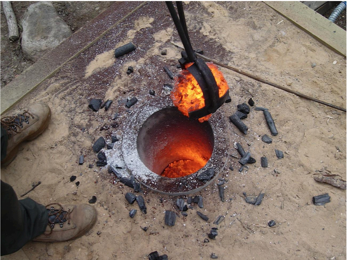
FIG 6. IRON HEMATITE ORE THAT HAS SMELTED INTO A METALLIC FORM, I.E. "BLOOM" RISES FROM THE FURNACE. PHOTO BY JOUNI JÄPPINEN
