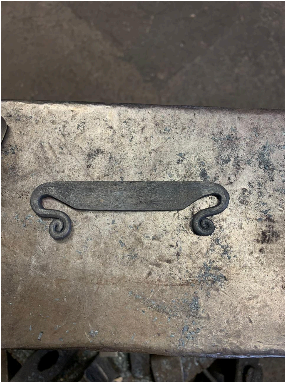
FIG 10. THE IRON FIBULA IS FORGED AGAINST THE ANVIL HORN AND CORNER BY THE BLACKSMITH MASTER TIIA LAHTI IN THE WINTER OF 2024. PHOTO'S BY TIIA LAHTI.
