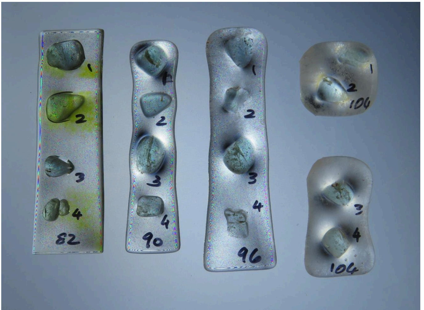
FIG 17. THE GLASS THROUGH THE POLARISING FILM. THE WHITE HALOES SHOW THE STRESS POINTS. PHOTO BY SUE HEASER.
