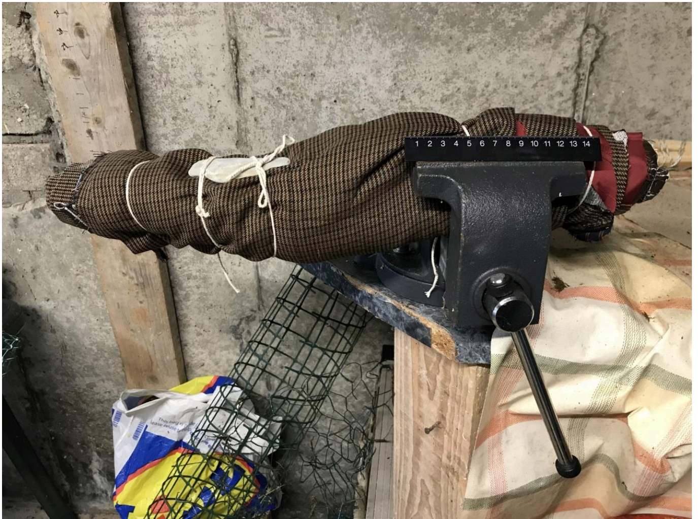
FIG 10. THE PROXY FOREARM HELD IN VICE TO MIMIC THE HUMAN GESTURE HOLDING IT AS PROTECTION. A TRIAL STONE IS ATTACHED. PHOTO BY STEPHEN LALOR.
