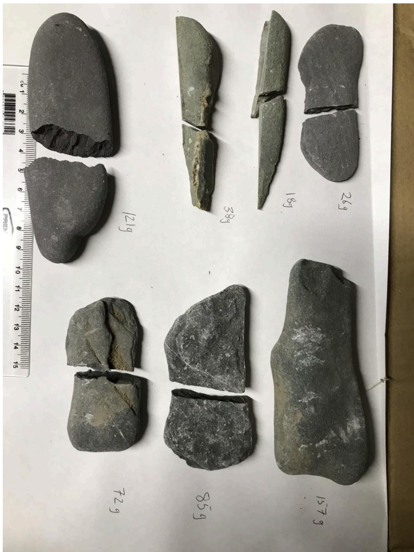
FIG 14. THE PROXY WRIST-GUARDS AFTER BEING STRUCK BY THE STONE-KNIFE. THEY SHATTERED EASILY EXCEPT FOR THE 157G WHICH RESISTED THE BLOWS. PHOTO BY STEPHEN LALOR.
