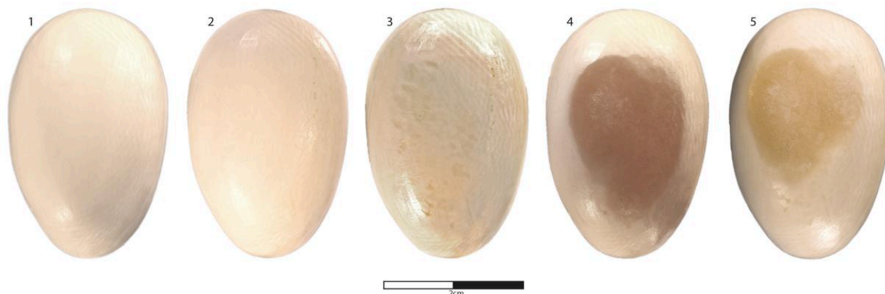
FIG 12. EXPERIMENTAL OBJECT N°1 MADE FROM AFRICAN ELEPHANT IVORY THAT RESEMBLES THE ARTEFACT FROM HOHLE FELS N° 100/2254, TOP VIEW ON THE PROXIMAL END. 1) FINAL OBJECT READY TO BE USED, 2) AFTER ACTION N°1 (PESTLE ON A FLAT PLATE), 3) AFTER ACTION N°2 (POUNDING ON A FLAT PLATE), 4) AFTER ACTION N° 3 (STRIKING/HITTING ON THE PROXIMAL SURFACE), 5) AFTER ACTION N° 4 (HAMMERING ON ONE POINT ON THE PROXIMAL SURFACE). PHOTOS BY A. FATZ, SHEP TÜBINGEN.
