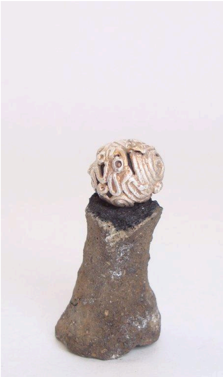
FIG 25. EXAMPLE OF AN EXPERIMENTAL BELL CAST IN SILVER.
