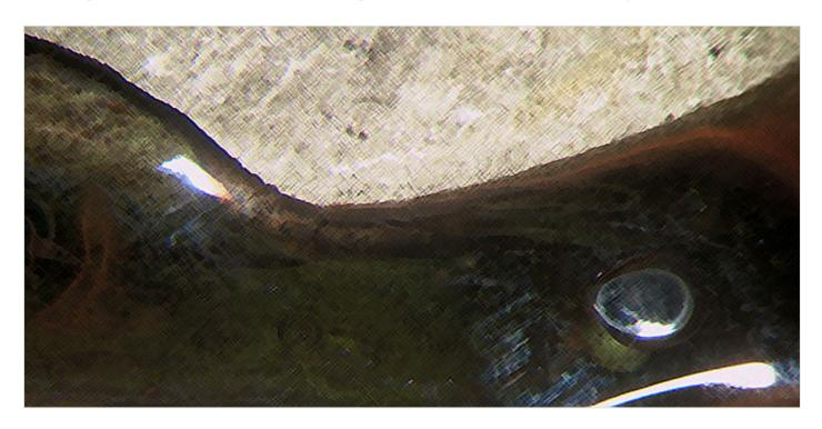
An historal technique of goldplating, described in 18th century literature, was reproduced. This cold-plating technique uses salts of gold, produced by dissolving gold in aqua regia. these salts are then rubbed onto a silver surfaces. Test prove that with this technique a thin goldlayer can be created on silver, though due to the small thickness it can not stand much wear.
