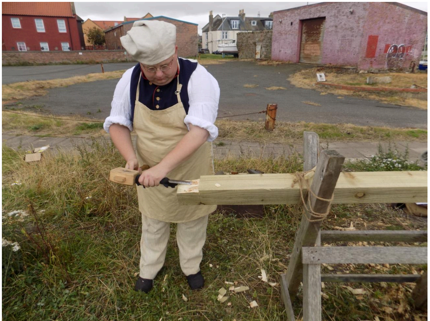
FIG 21. CUTTING JOINTS IN THE SLEEPERS. IT TOOK ONE INDIVIDUAL 40 MINUTES TO PRODUCE ONE SLEEPER WORKING ON THEIR OWN USING HAND TOOLS. AS WITH RAILS, IT IS LIKELY THEY WERE PREPARED OFF-SITE. PHOTO BY ANTHONY DAWSON.
