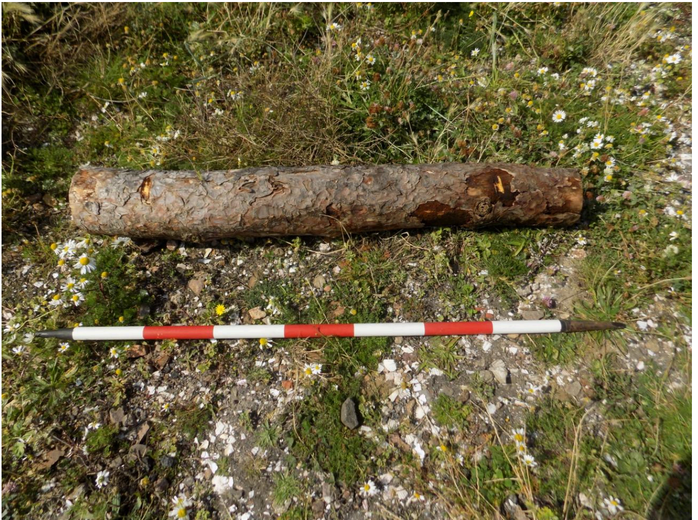
FIG 10. SLEEPER CUT TO LENGTH, BEFORE FURTHER PROCESSING TO CREATE A SHOULDER AND REBATE TO TAKE THE RAIL. PHOTO BY ANTHONY DAWSON.
