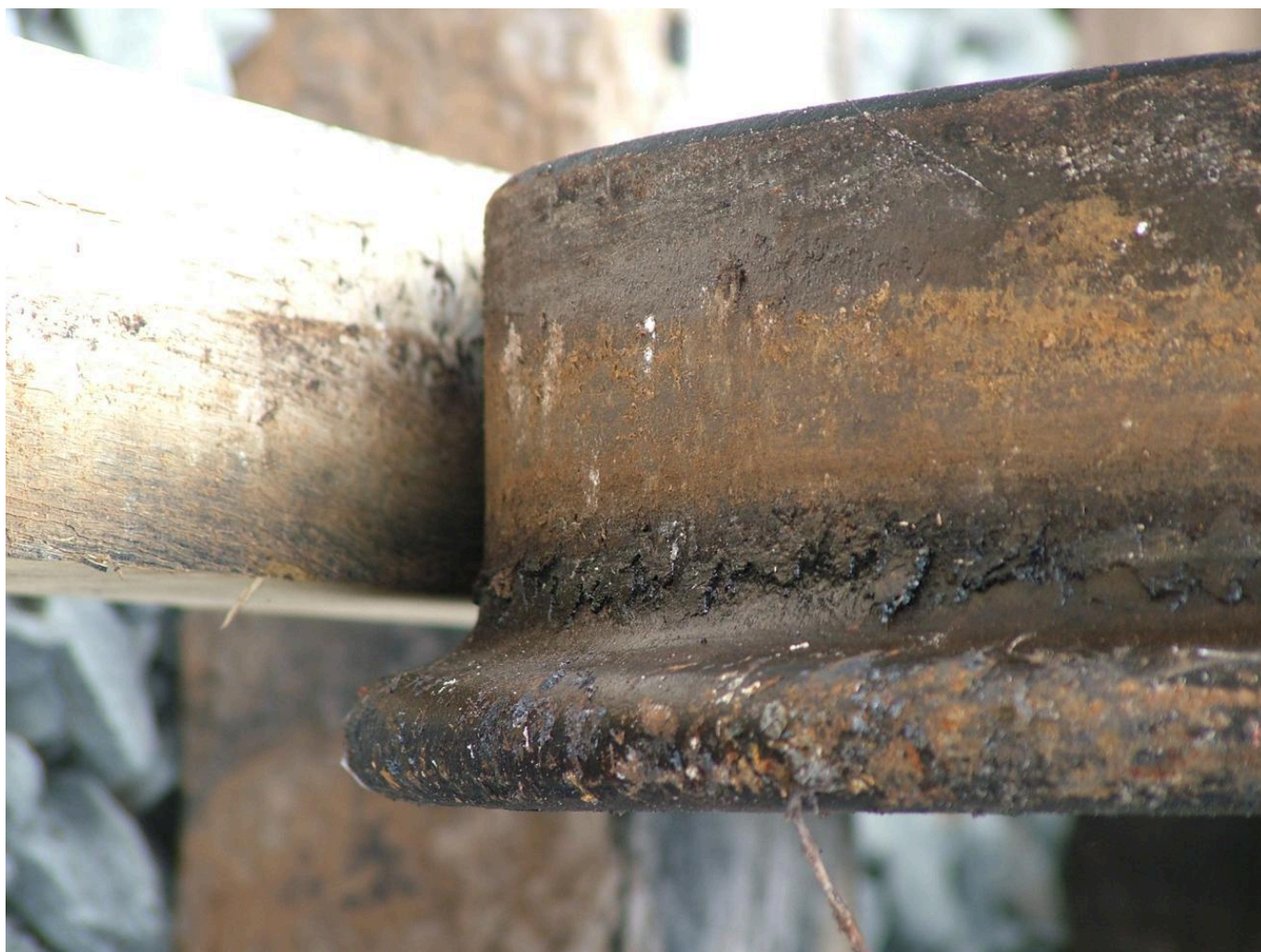
FIG 7. THE RELATIVELY POOR INTERFACE BETWEEN A CONED, CAST-IRON WHEEL ON THE REPLICA 'CHALDRON' TYPE WAGGON AND THE WOODEN RAIL. THE WHEEL IS TRYING TO CRUSH THE WOOD TO MIRROR THE SHAPE OF ITS TREAD. PHOTO BY PAUL JARMAN, BEAMISH MUSEUM.
