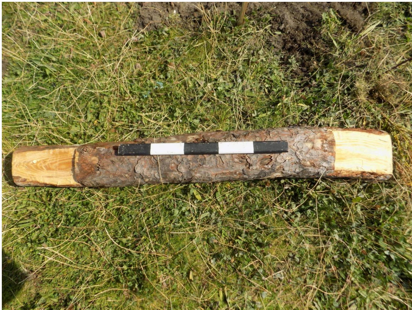
FIG 12. COMPLETED SLEEPER, DEMONSTRATING THE MINIMUM AMOUNT OF PROCESSING REQUIRED TO PREPARE ONE. IN TOTAL ONE INDIVIDUAL TOOK 60 MINUTES TO PRODUCE A SINGLE SLEEPER. PHOTO BY ANTHONY DAWSON.
