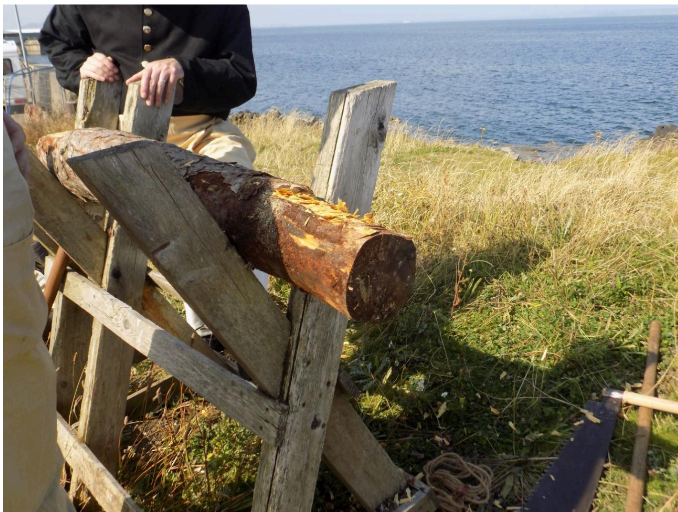
FIG 11. CUTTING SHOULDERS AND REBATES ON THE SLEEPER WAS BY SAW TO MARK OUT THE SHOULDER, AND THEN USING HAND AXES AND A BOX PLAIN TO CREATE A LEVEL SURFACE ONTO WHICH THE RAIL WOULD SIT. PHOTO BY ANTHONY DAWSON.
