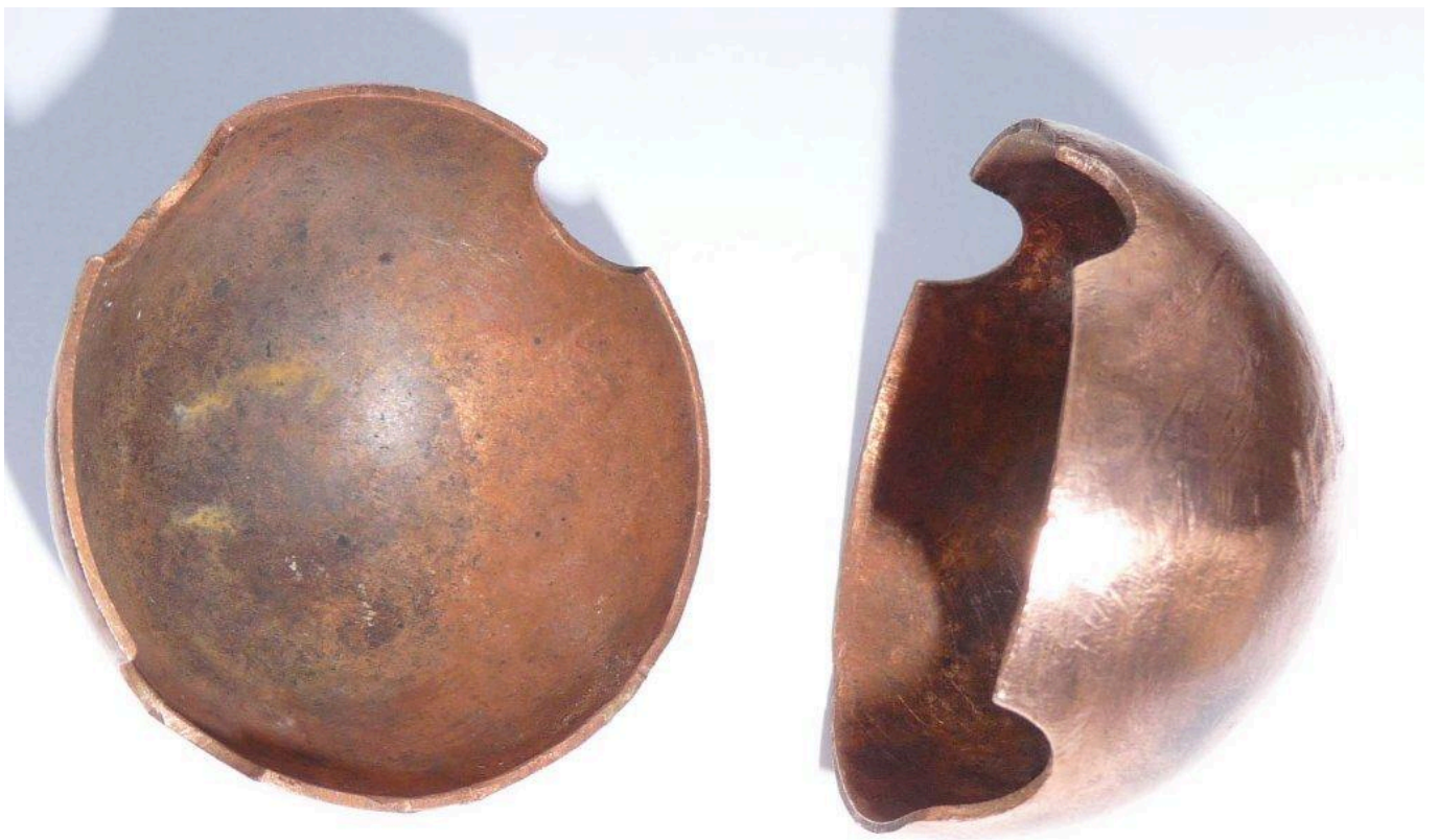
FIG 10. CASTING PRODUCED FROM METAL MOULD.
