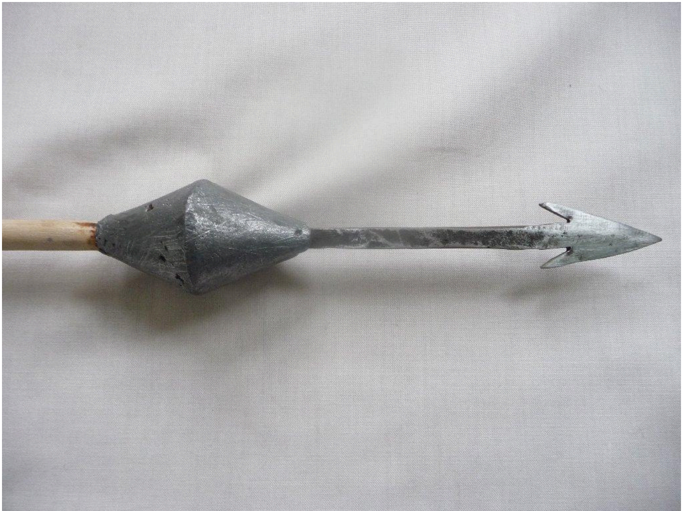
FIG 10. CASTING PRODUCED FROM METAL MOULD.
