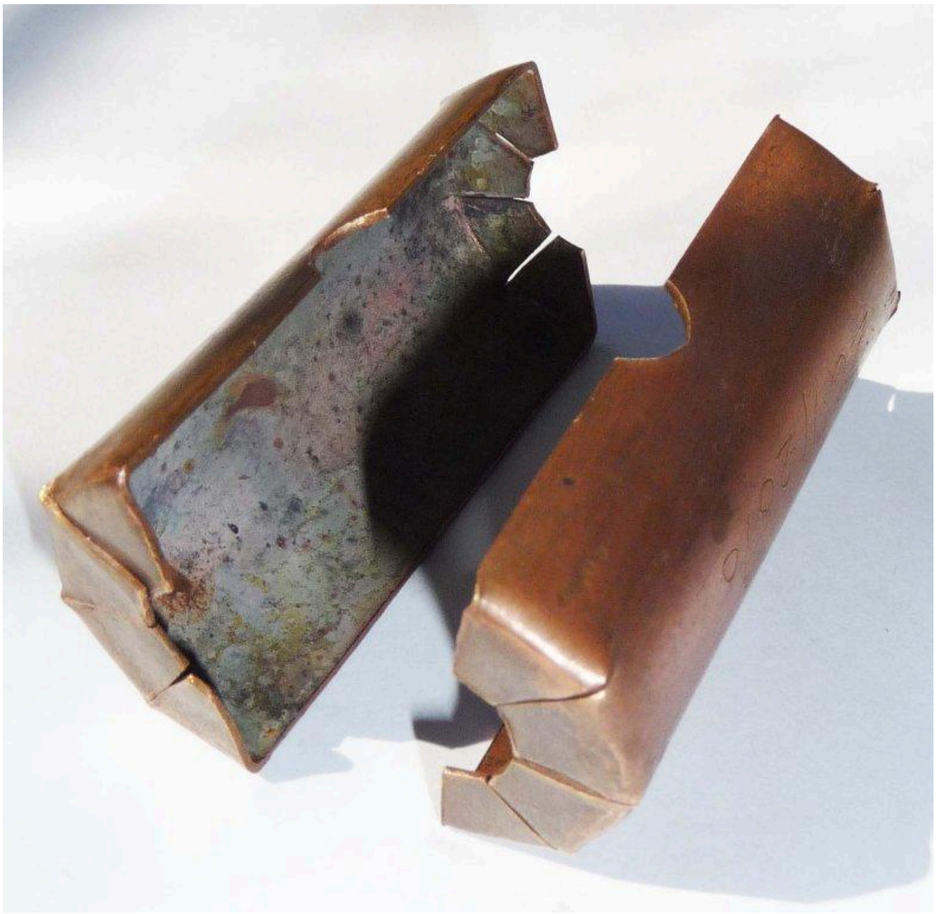
FIG 13. TWO HALVES OF A CYLINDRICAL COPPER MOULD.
