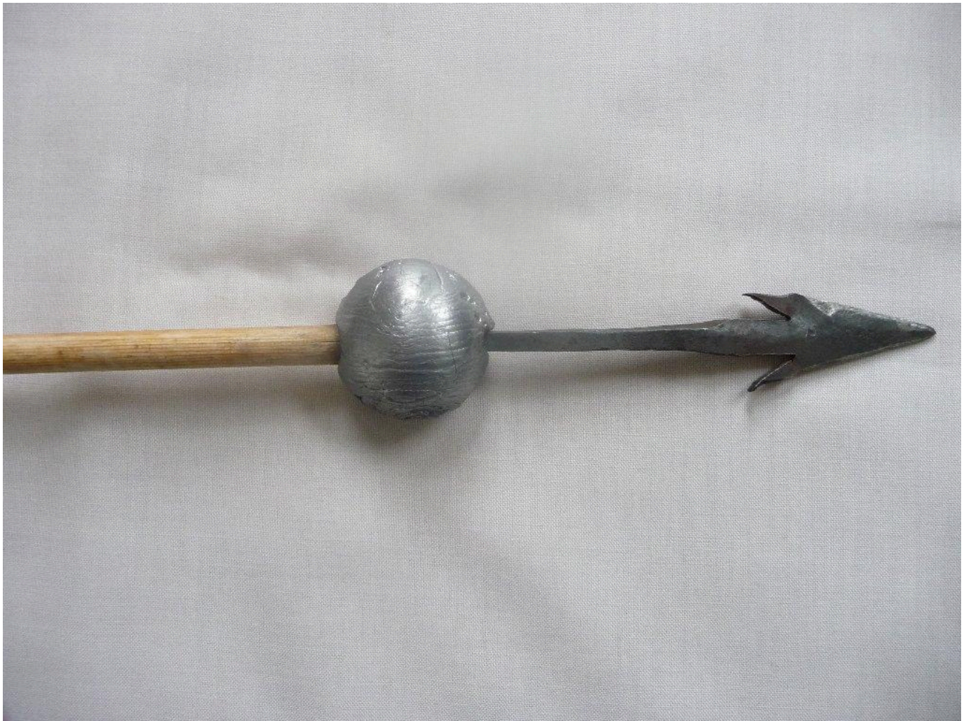
FIG 12. CASTING PRODUCED FROM METAL MOULD.
