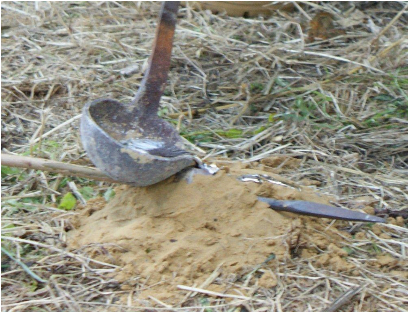
FIG 16. THE METHOD OF CASTING BY BURYING IN SAND.
