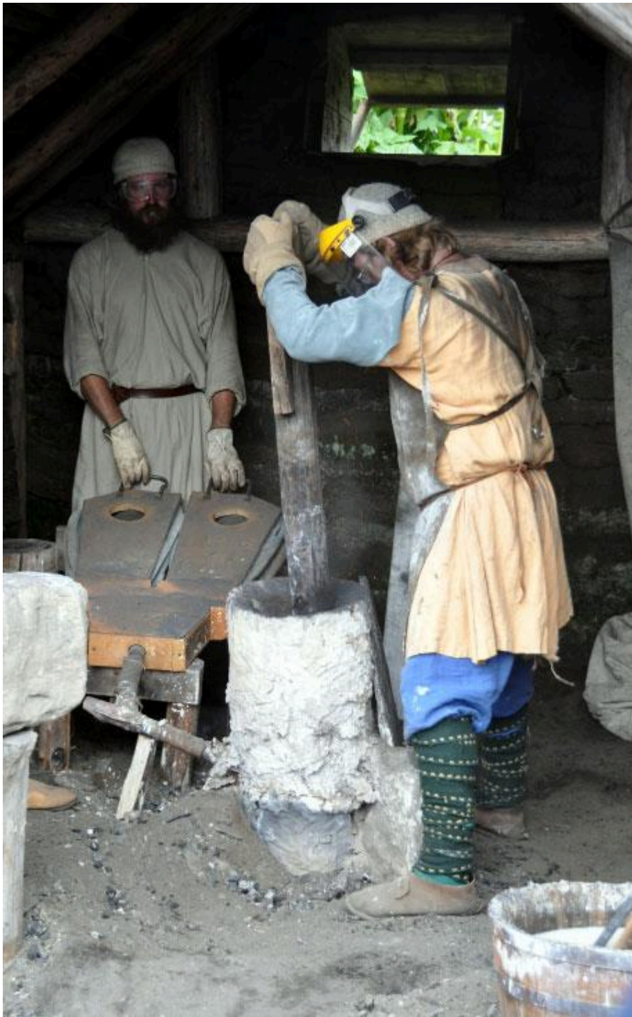
FIG 7. USING THE 'THUMPER' TO COMPACT AND LOOSEN THE BLOOM WHILE IN PLACE INSIDE THE FURNACE.
