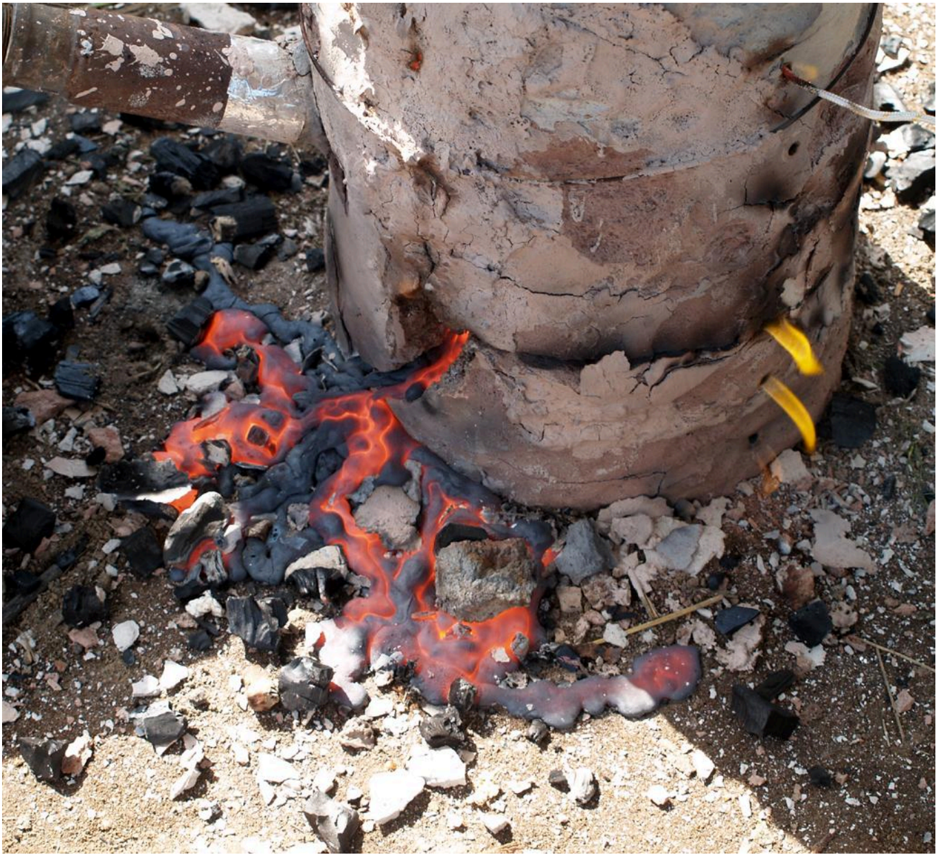
FIG 5. A FURNACE SELF TAPING EXCESS LIQUID SLAG (INCONTINENT).
