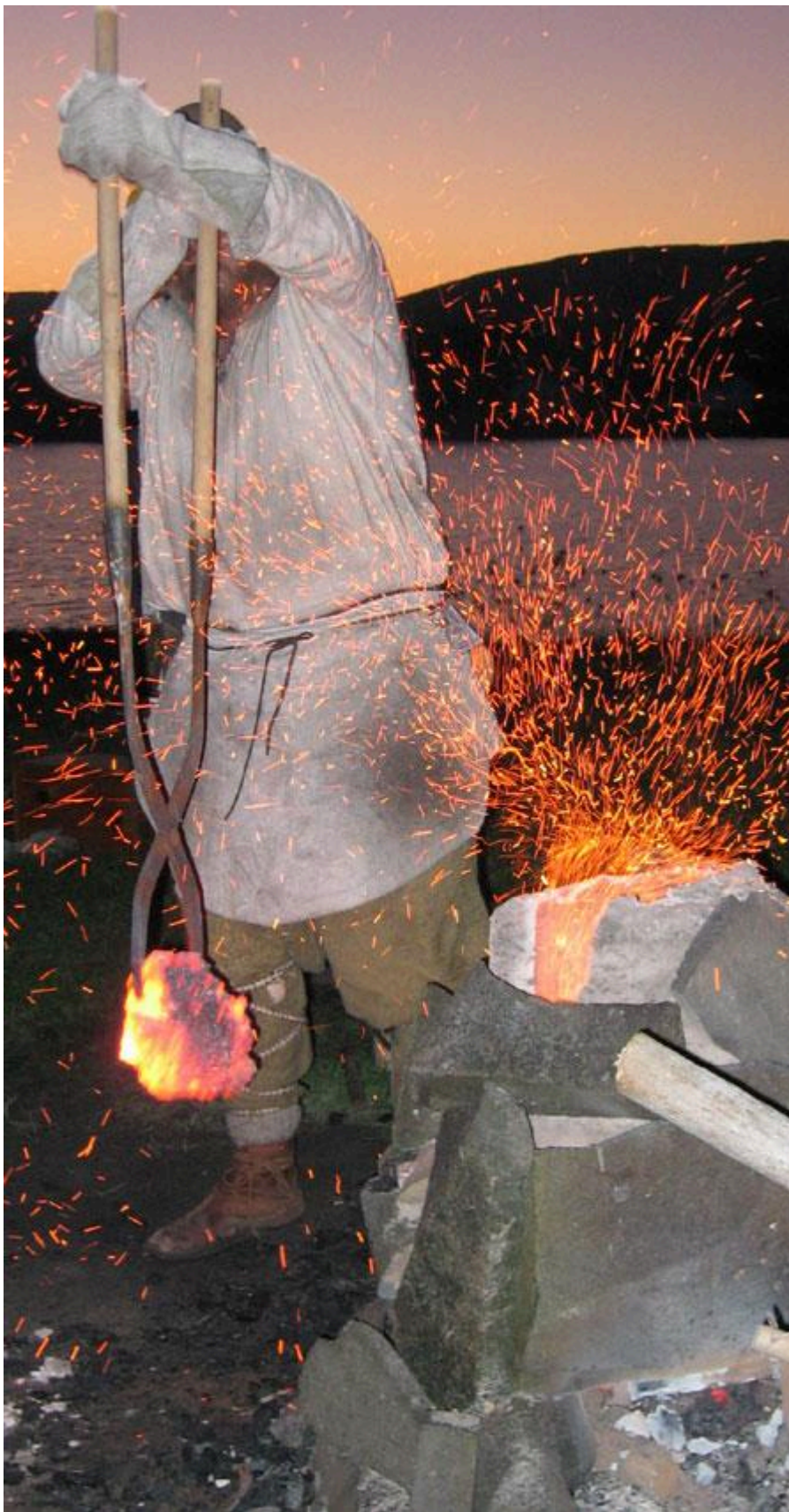
FIG 9. PULLING THE BLOOM! CANIRON 5, AUGUST 2005
