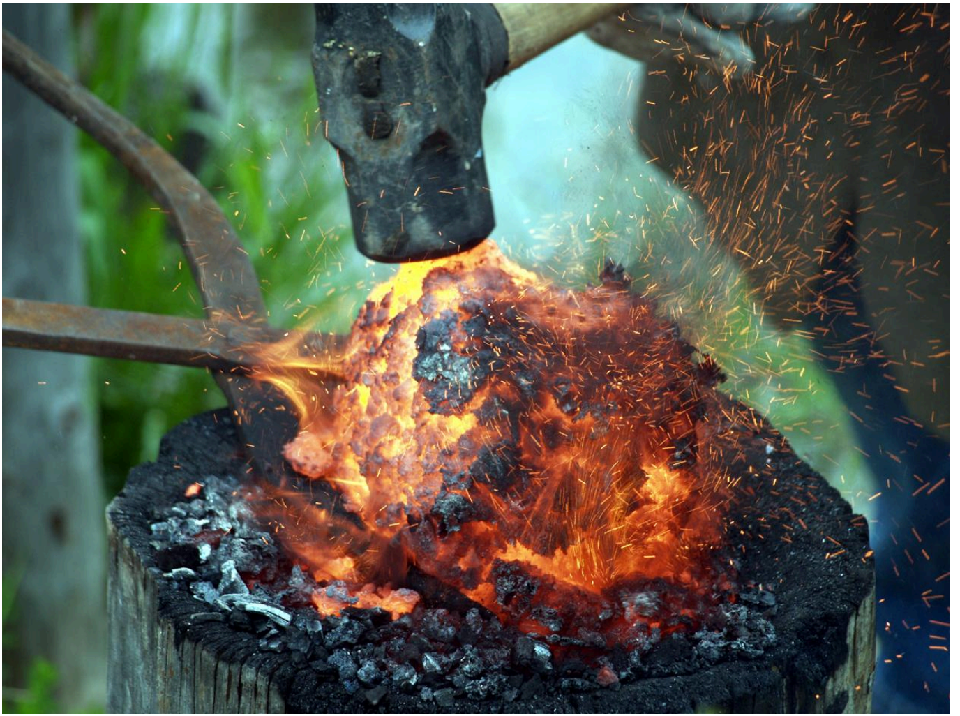
FIG 6. A HOT BLOOM, RIGHT AFTER EXTRACTION.
