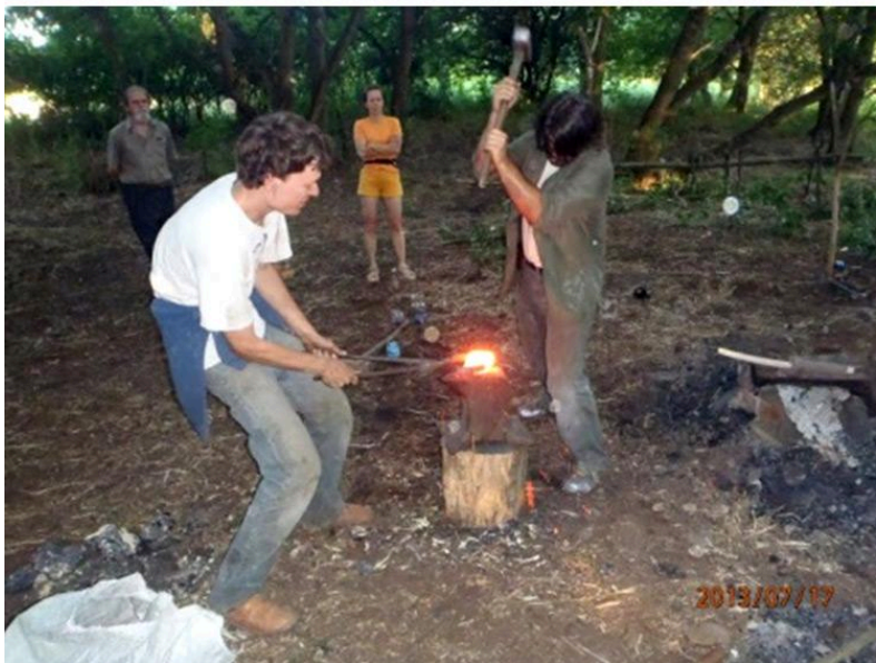
FIG 6. FORGING PATTERN-WELDED RODS FROM IRON BLOOMS.
