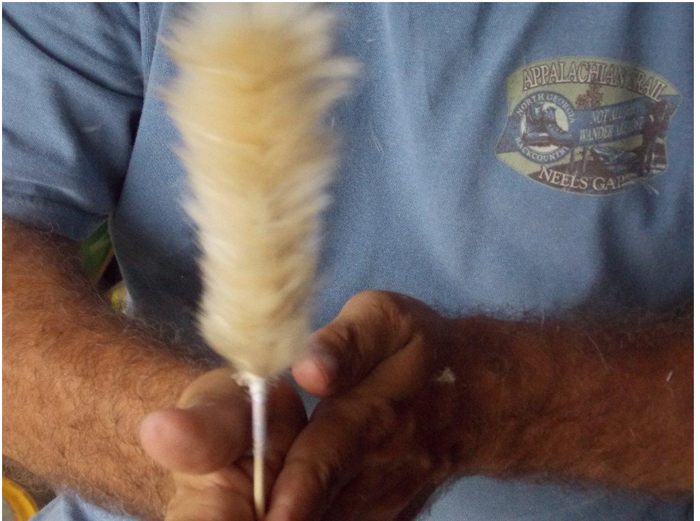
FIG 23. SPIN THE DART TO REMOVE EXTRA FILAMENT THAT DID NOT GET CAUGHT UNDER THE STRING.
