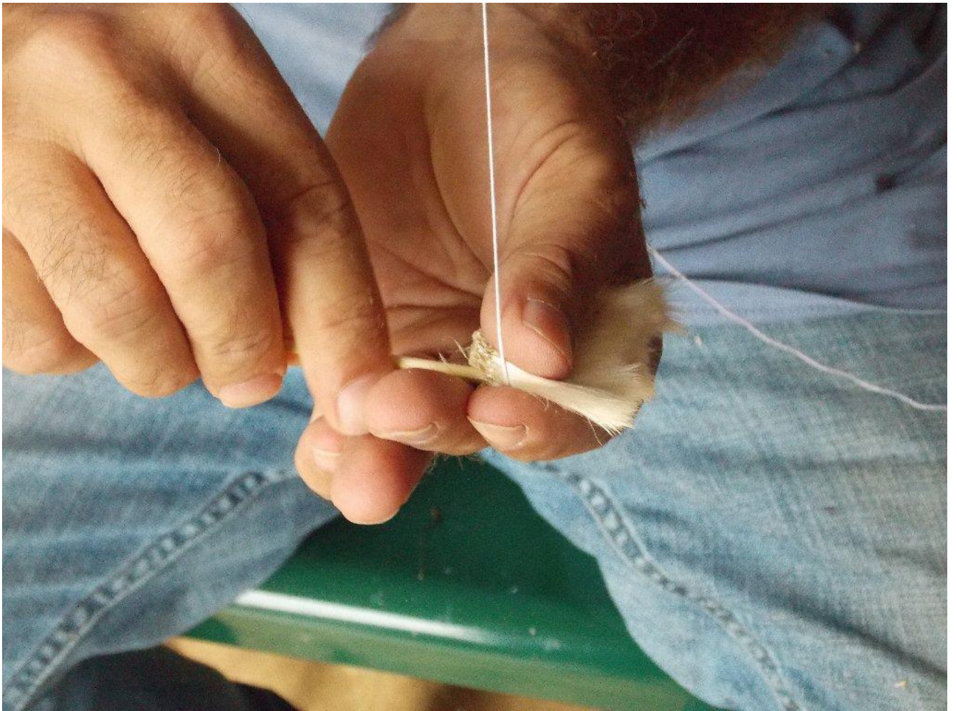
FIG 19. BEGINNING TO ROLL THE DART. ROLL AWAY FROM YOU AND SLOWLY PUSH TO THE RIGHT OF THE PHOTO.
