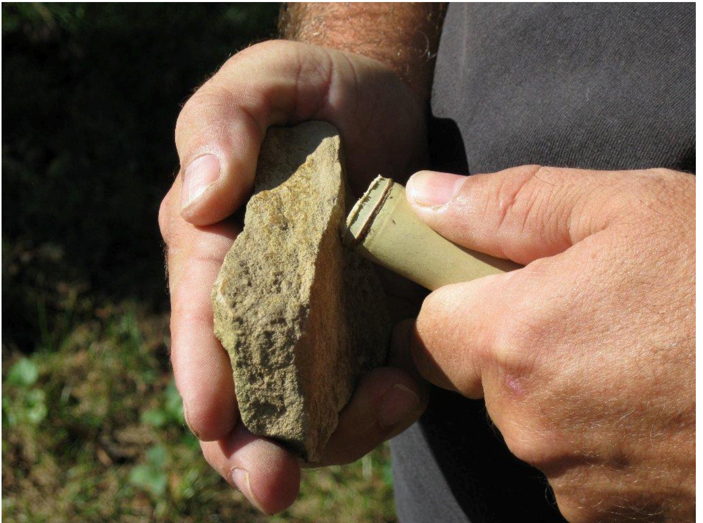
FIG 8. USING SANDSTONE TO SMOOTH THE MOUTHPIECE.
