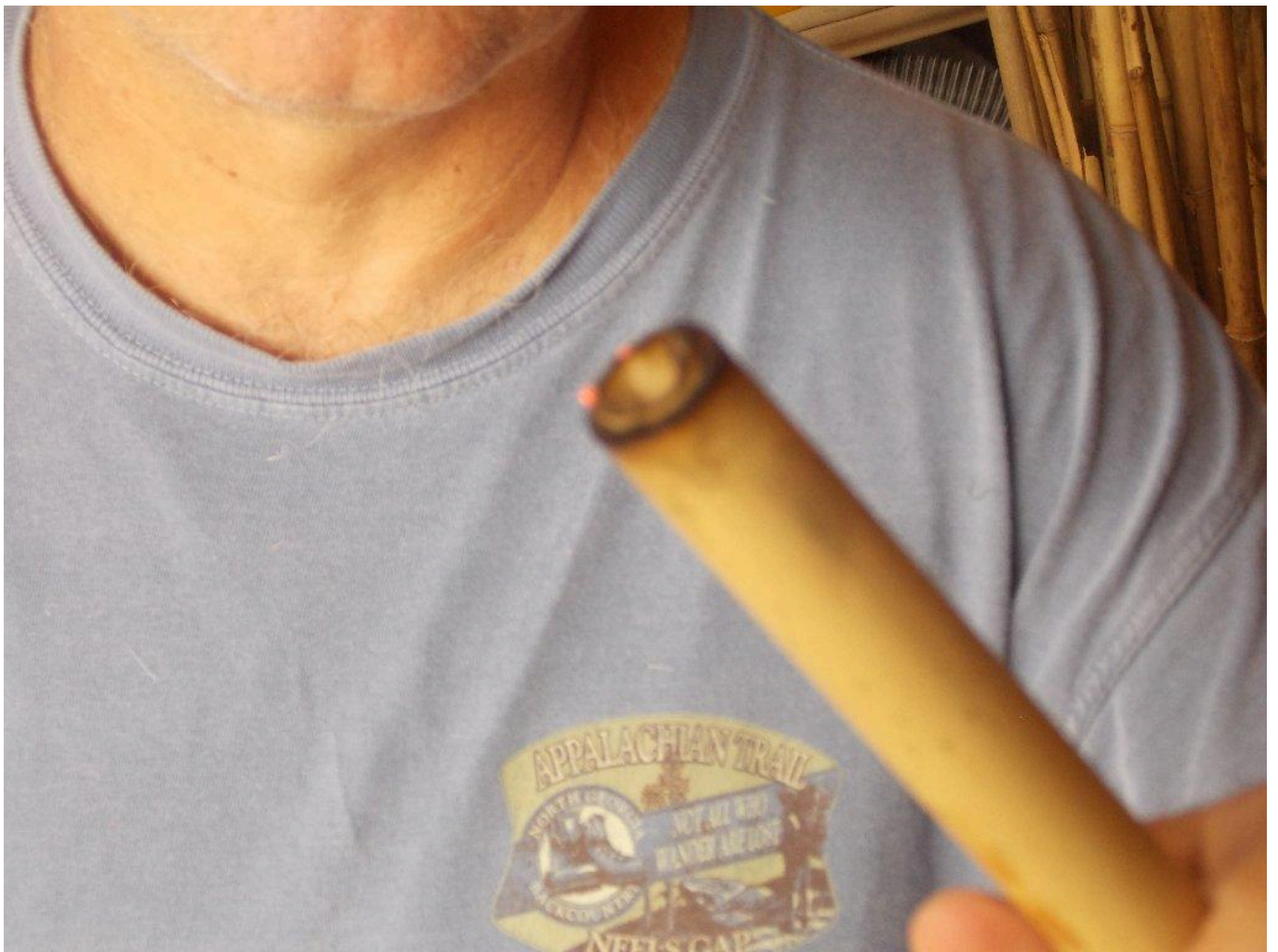
FIG 26. BURNING THE EXCESS FIBERS IN A TUBE. BY PLACING YOUR HAND OVER THE TUBE YOU CUT OFF THE OXYGEN AND STOP THE WHOLE DART FROM BURNING.
