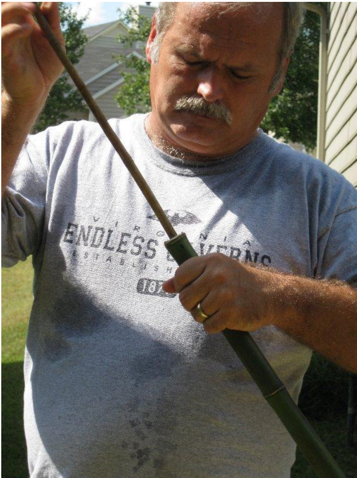
FIG 7. USING A SMALLER DIAMETER PIECE OF CANE TO REAM OUT THE BLOWGUN. BY ADDING A SLURRY OF SAND AND WATER YOU CAN SAND THE INTERIOR OF THE BLOWGUN.
