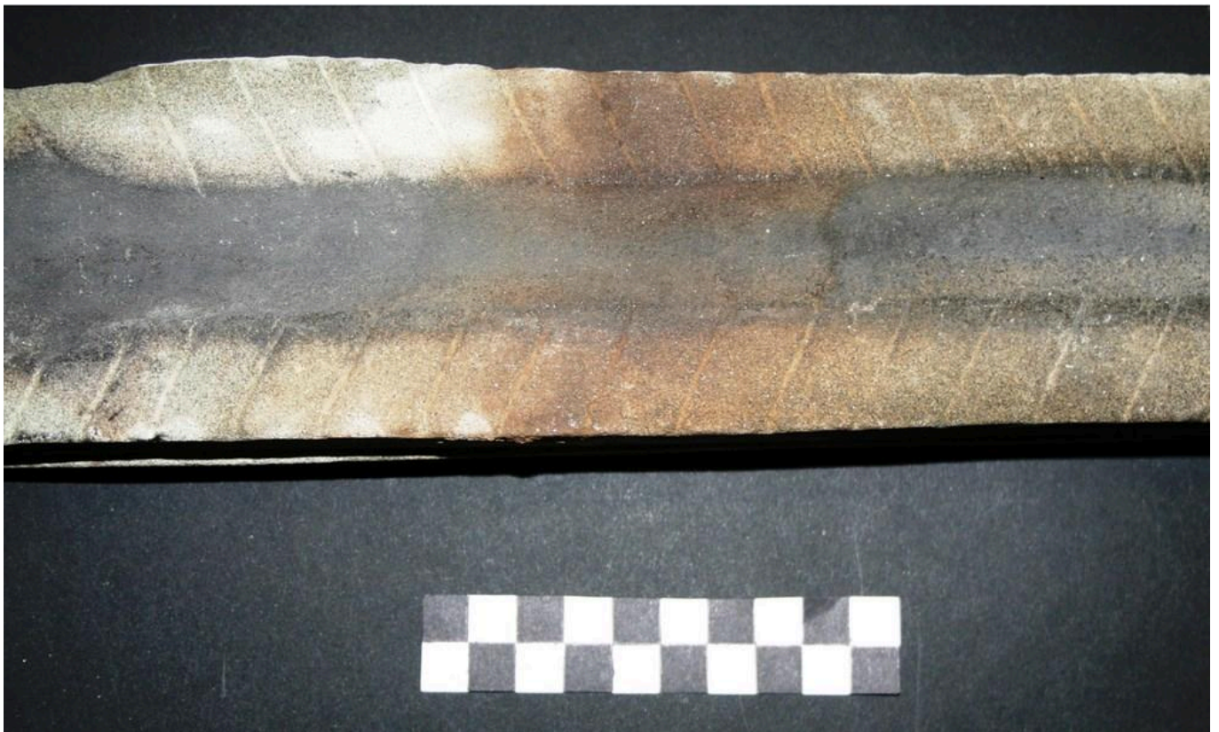
FIG 4B. PROBLEMS WITH EXPERIMENTAL STONE MOULDS: DETERIORATION FROM FREQUENT UTILIZATION.
