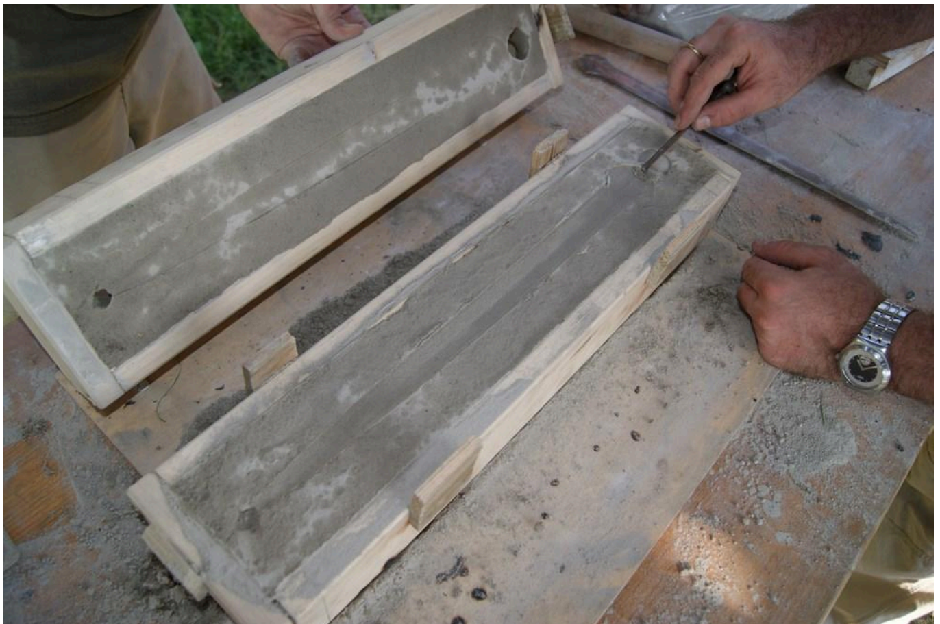
FIG 5D. OPERATIONAL CHAIN FOR THE REALIZATION OF A SAND MOULD: RE-OPENING OF THE TWO BOXES AFTER HAVING FILLED THE UPPER BOX.
