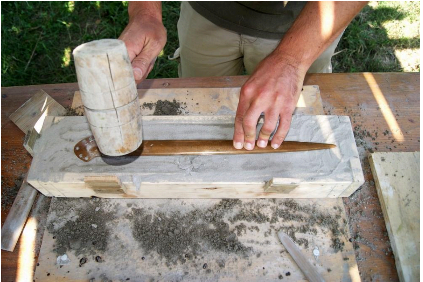
FIG 5C. OPERATIONAL CHAIN FOR THE REALIZATION OF A SAND MOULD: PUSHING THE SWORD MODEL INTO THE SAND TO OBTAIN THE SHAPE.
