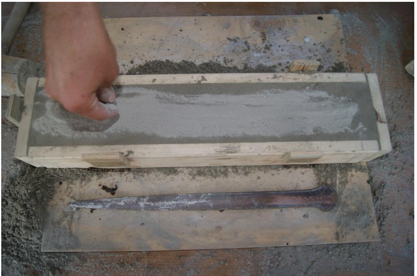
FIG 5B. OPERATIONAL CHAIN FOR THE REALIZATION OF A SAND MOULD: COVERING WET SAND WITH A THIN LAYER OF DRY SAND ORDER TO ALLOW THE REOPENING OF THE TWO BOXES.
