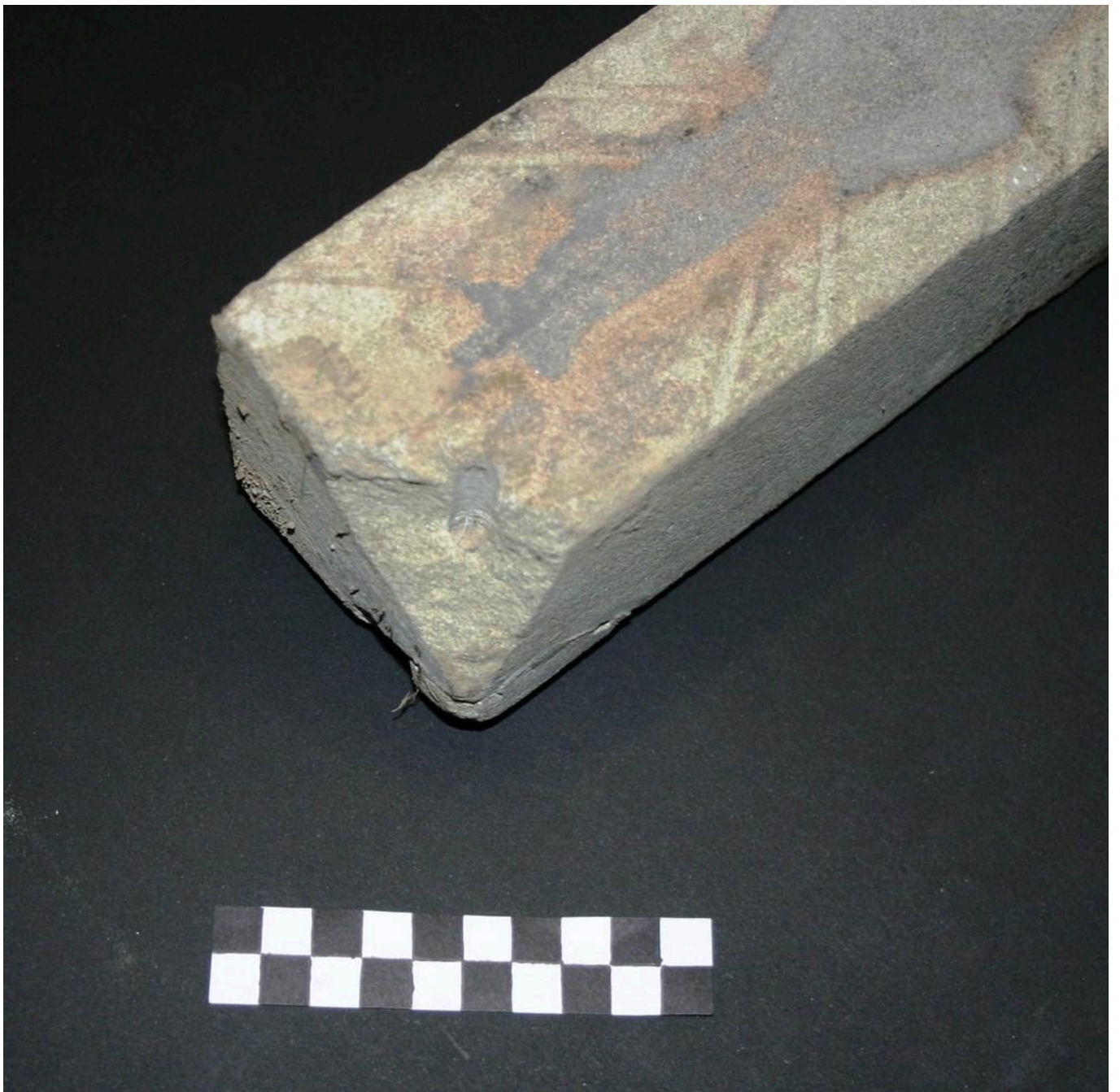
FIG 4A. PROBLEMS WITH EXPERIMENTAL STONE MOULDS: DETERIORATION FROM FREQUENT UTILIZATION.
