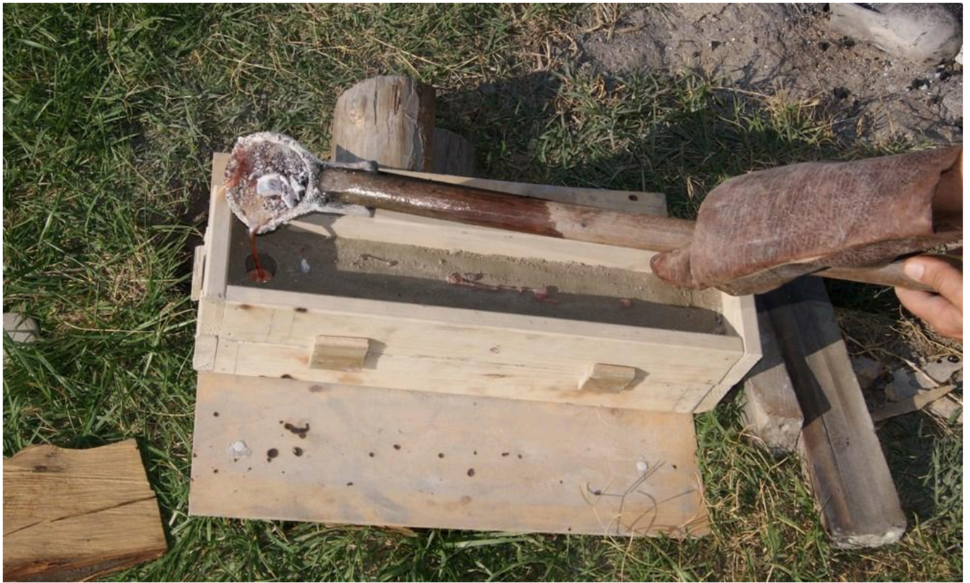
FIG 5E. OPERATIONAL CHAIN FOR THE REALIZATION OF A SAND MOULD: BRONZE CASTING.
