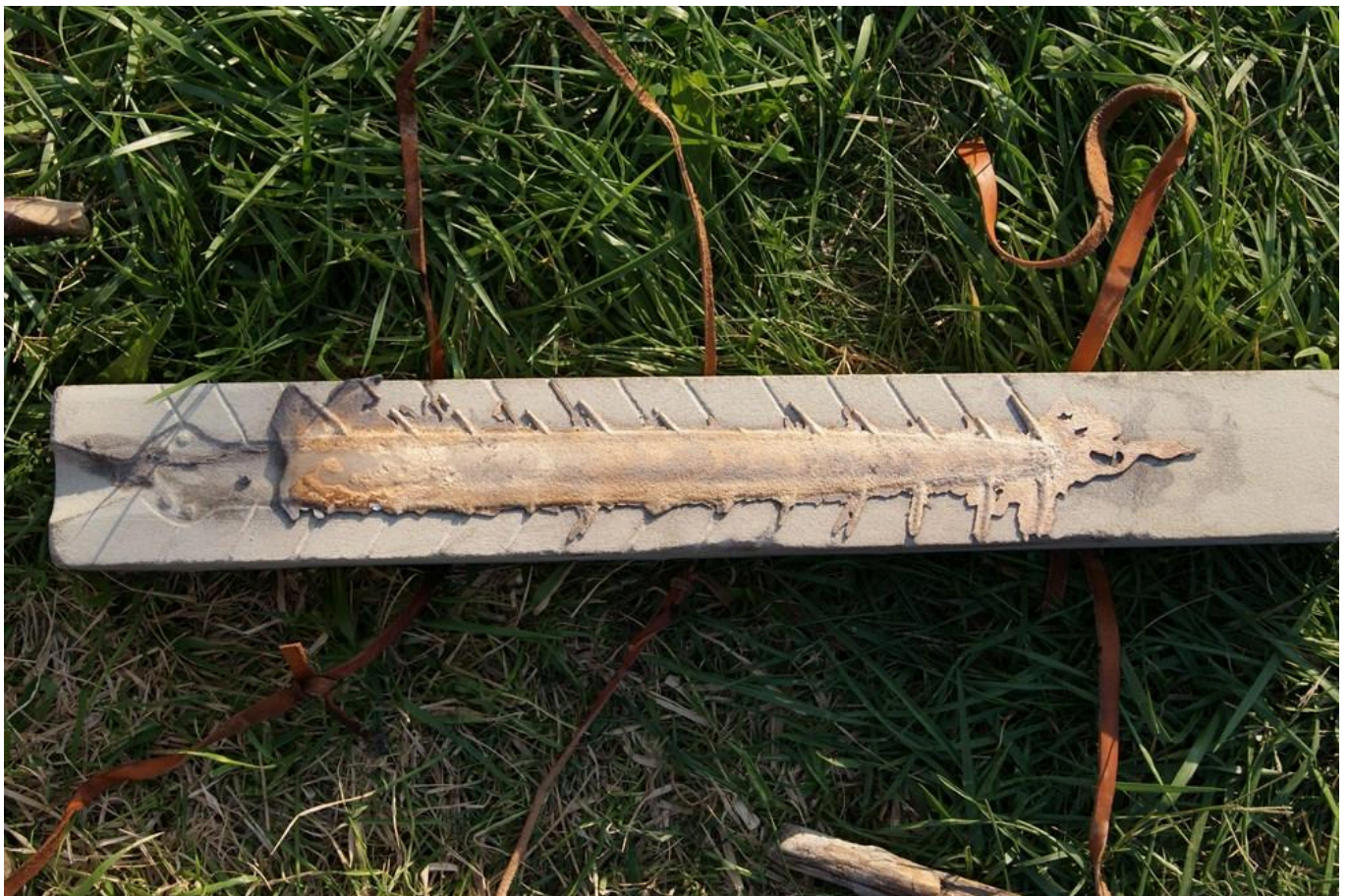
FIG 4C. PROBLEMS WITH EXPERIMENTAL STONE MOULDS: DEFORMATION OF THE STONE CAUSED BY THE HIGH TEMPERATURE AND THE FREQUENT UTILIZATION.
