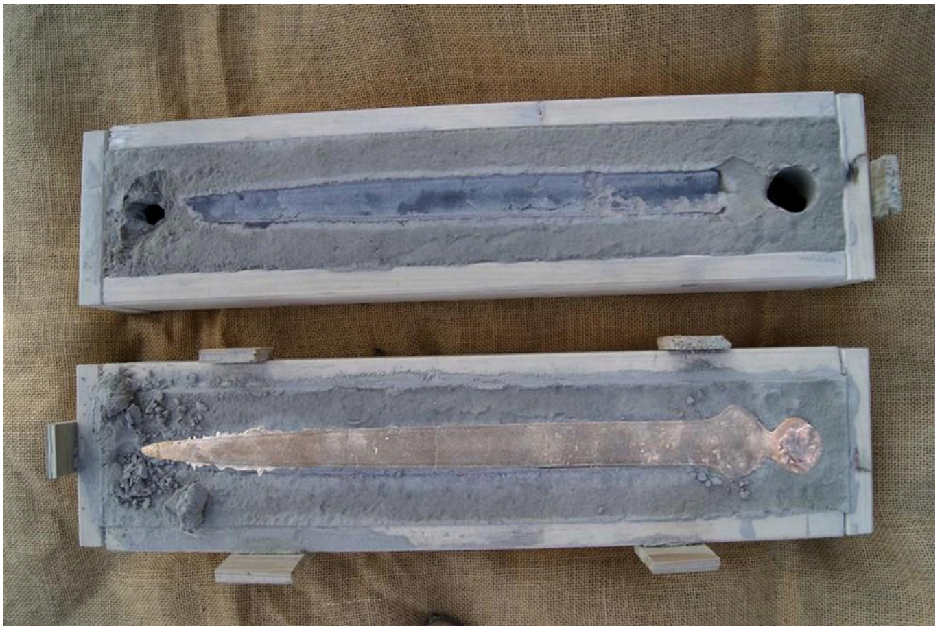
FIG 5F. OPERATIONAL CHAIN FOR THE REALIZATION OF A SAND MOULD: OPENING OF THE MOULDS.
