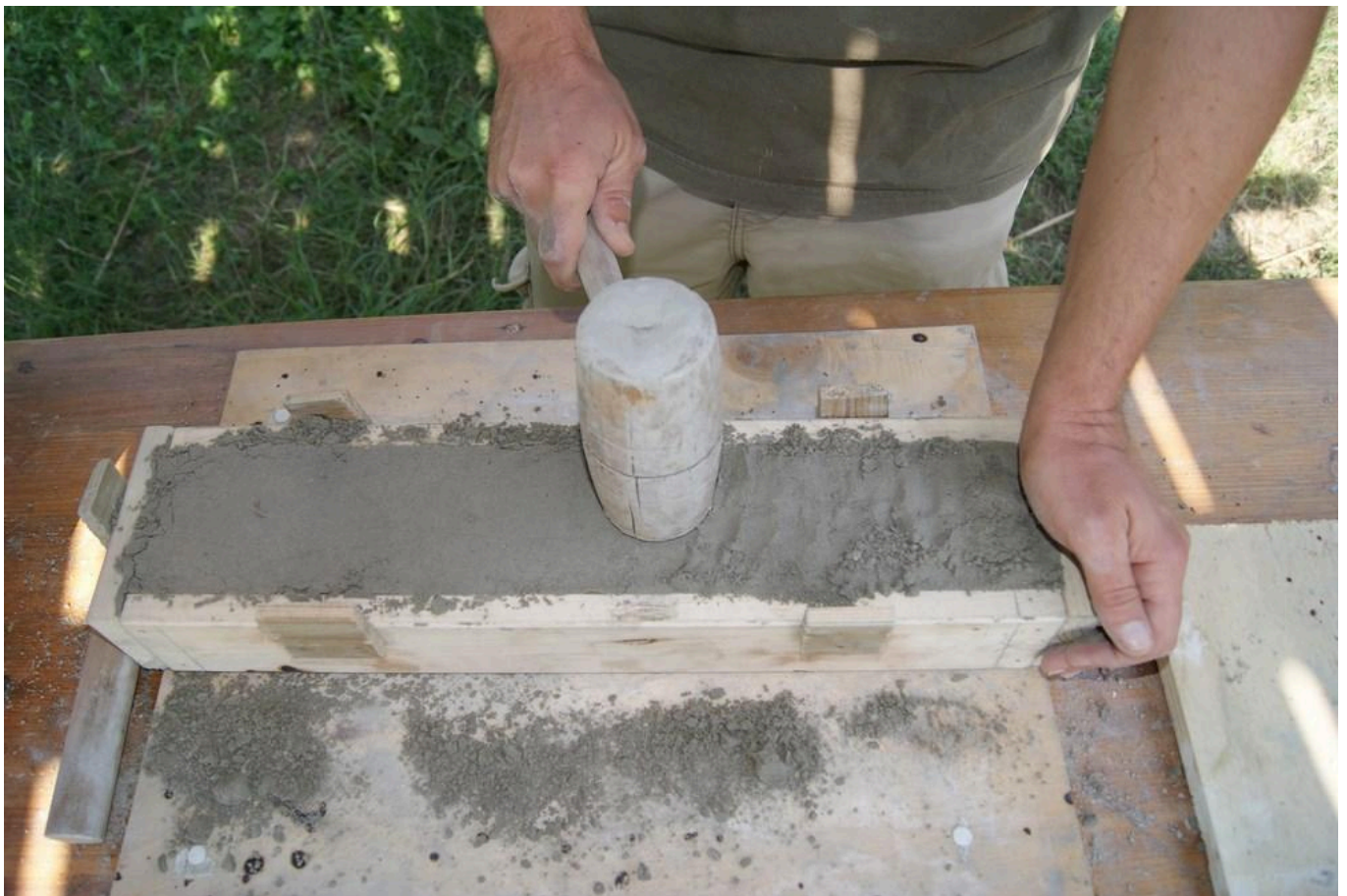
FIG 5A. OPERATIONAL CHAIN FOR THE REALIZATION OF A SAND MOULD: FILLING ONE OF THE TWO WOODEN BOXES WITH CALCAREOUS FINE SAND AND PRESSING IT WITH A HAMMER.
