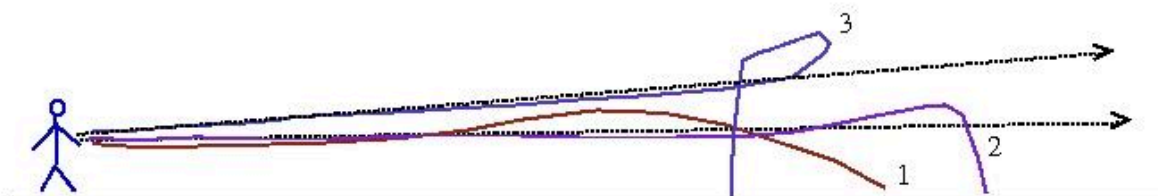
FIG 17. THE DIFFERENT TYPICAL TRAJECTORIES OBSERVED DURING THE TESTS: (1) INACCURATE S SHAPED TRAJECTORY BY THROWING THE OBJECT HORIZONTALLY, WITHOUT INCIDENCE OR DIHEDRAL ANGLE TOWARD THE GROUND: (2) OPTIMAL LOW TRAJECTORY BY THROWING NEAR VERTICAL PLANE: (3) OPTIMAL HIGHER TRAJECTORY BY THROWING WITH A 45^\circ ANGLE FROM THE VERTICAL.
