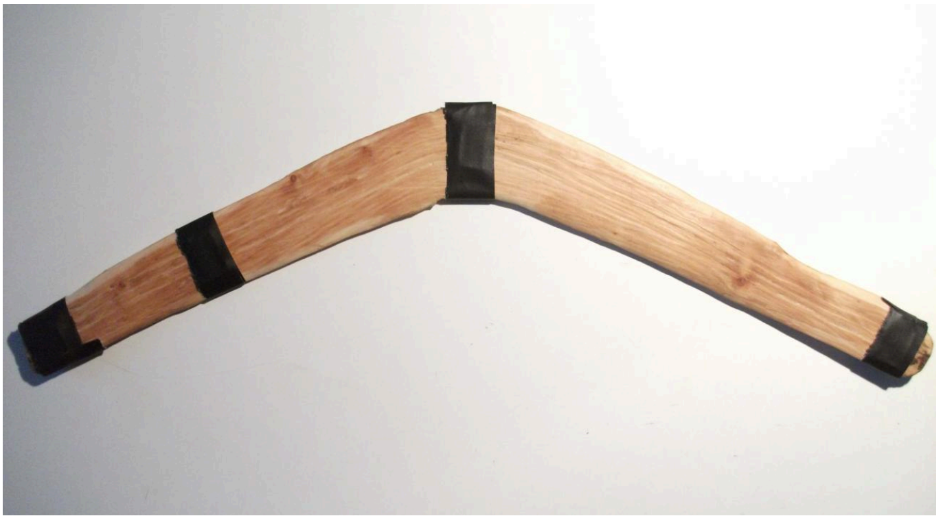
FIG 18. REPLICA WEIGHTED WITH LEAD FIXED BY ADHESIVE TAPE (PREPARED FOR FOUR STRIP TEST)
