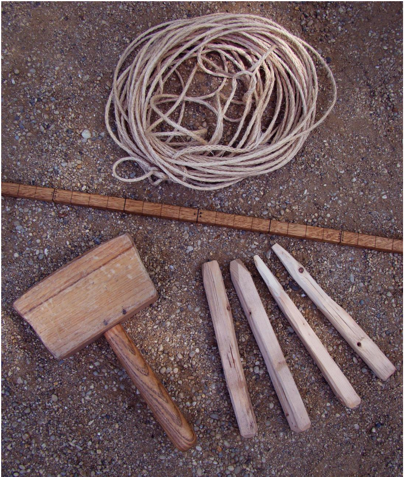
FIG 6. DURING THE PRACTICAL WORK IN ASPARN, THE HYPOTHESIS WAS ESTABLISHED THAT THE GROUND PLAN OF LONGHOUSES IN THE LINEAR POTTERY CULTURE MIGHT HAVE BEEN SET OUT WITH THE HELP OF TAUT CORDS, WOODEN PEGS AND A YARDSTICK AT THE CONSTRUCTION SITE.
