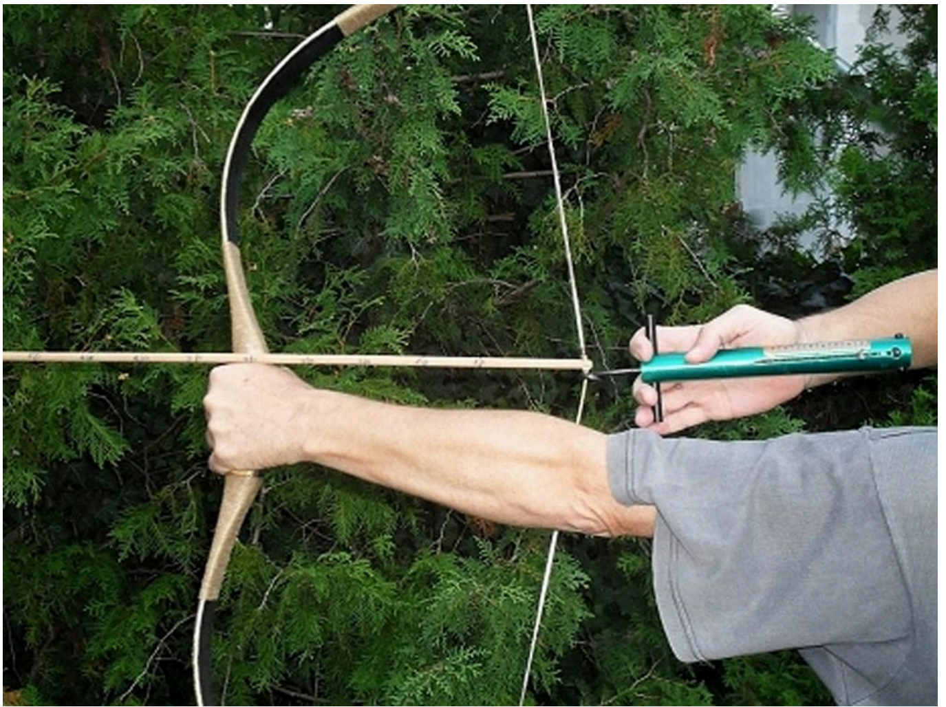
FIG 2. MEASURING THE POWER OF A BOW WITH MANUAL POWER METER.
