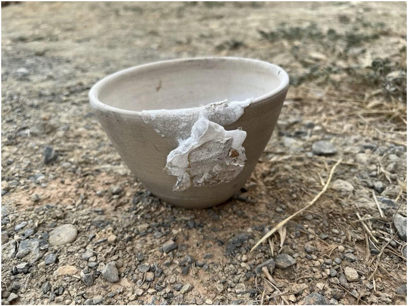
FIG 18. GLASMA AND KILN BATT MIXTURE WHICH WAS DISPLACED DURING THE FIRING PROCESS. PHOTO BY SARAH MITCHELL.
