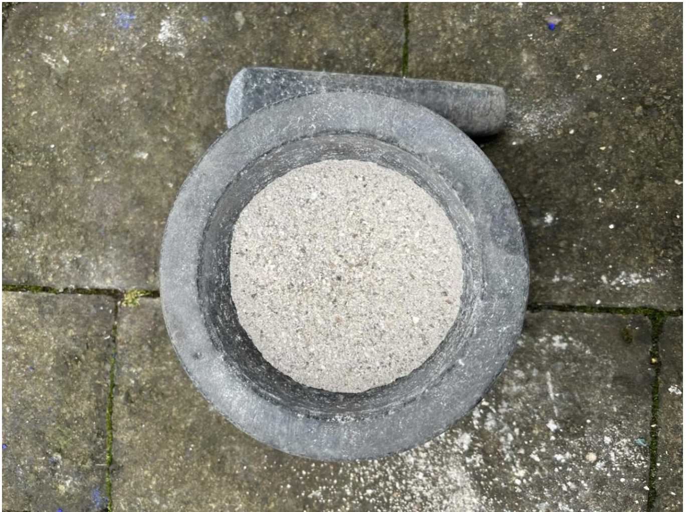
FIG 13. OYSTER SHELL FRAGMENTS DURING PROCESSING IN A PESTLE AND MORTAR. PHOTO BY SARAH MITCHELL.
