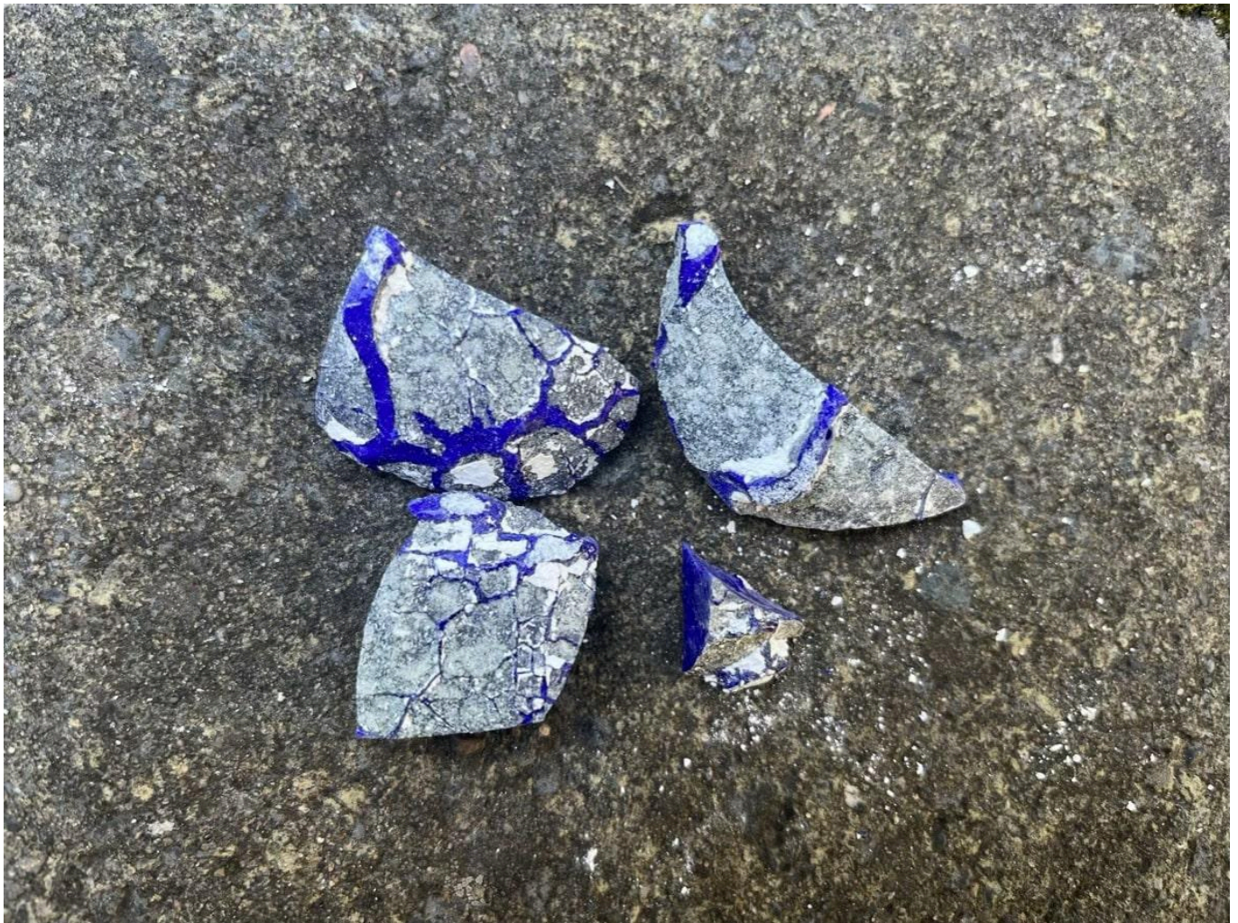
FIG 24. REMAINS OF GLASS FROM THE 1 MM LIME CRUCIBLE. A LAYER OF LIME RESIDUE CAN BE SEEN ON THE GLASS. PHOTO BY SARAH MITCHELL.
