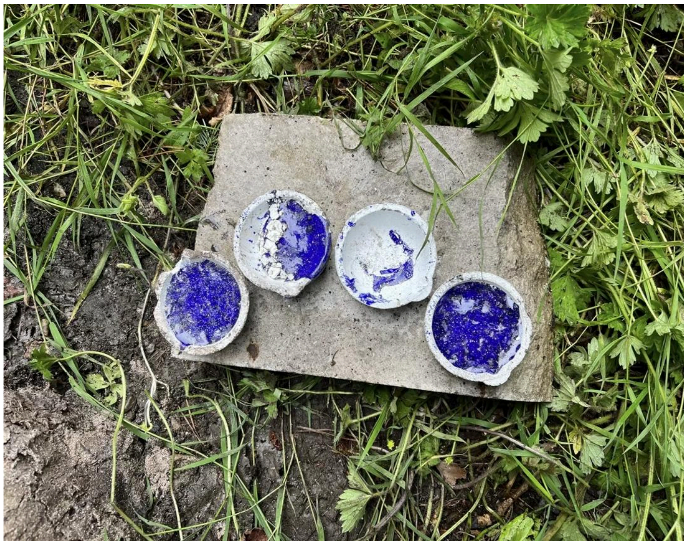
FIG 22. CRUCIBLES IMMEDIATELY AFTER FIRING, FROM LEFT TO RIGHT: OIL LINING; 1 MM THICK LIME LINING; 3 MM THICK LIME LINING; CONTROL. PHOTO BY SARAH MITCHELL.
