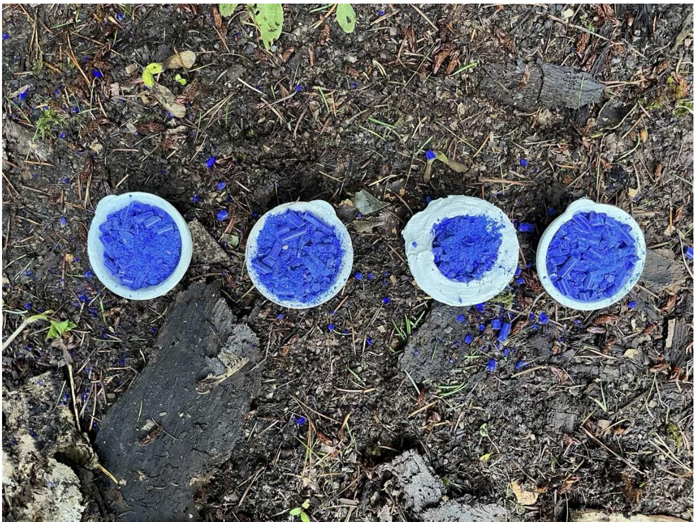
FIG 11. EACH CRUCIBLE PLACED IN THE FURNACE, FROM LEFT TO RIGHT: OIL LINING; LIME LINING, 1 MM THICK; LIME LINING, 3 MM THICK; CONTROL - NO LINING. PHOTO BY SARAH MITCHELL.
