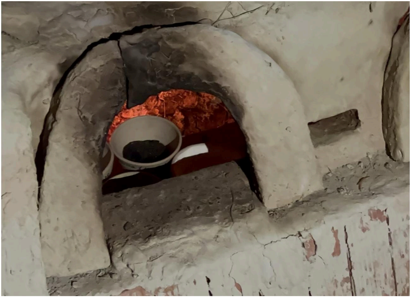
FIG 8. CRUCIBLES JUST AFTER BEING PLACED INSIDE THE FURNACE. PHOTO BY SARAH MITCHELL.
