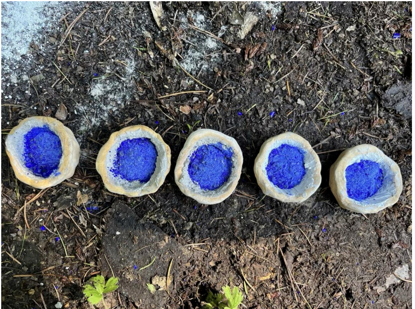
FIG 14. EACH CRUCIBLE PLACED IN THE FURNACE, FROM LEFT TO RIGHT: CRUCIBLES 5W, 6W AND 7W - SHELL LINING; 8W AND 9W - LIME LINING. PHOTO BY SARAH MITCHELL.
