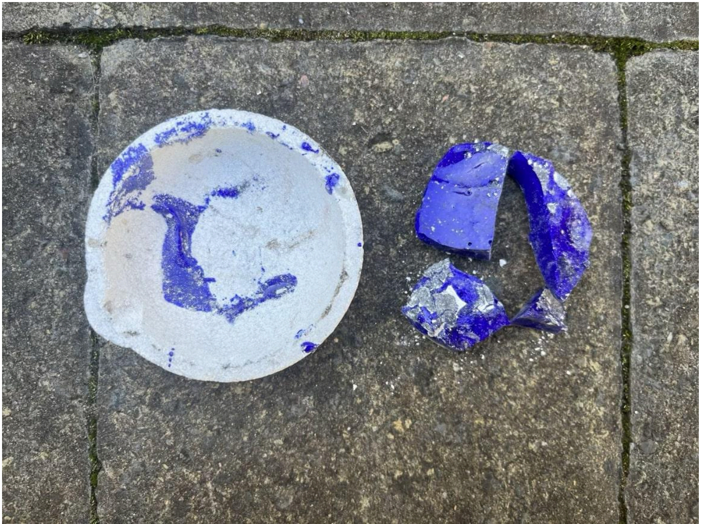
FIG 23. CRUCIBLE WHICH HAD A LIME LINING OF 1 MM THICKNESS. THE GLASS GRADUALLY SEPARATED FROM THE CRUCIBLE OVER SEVERAL DAYS. PHOTO BY SARAH MITCHELL.
