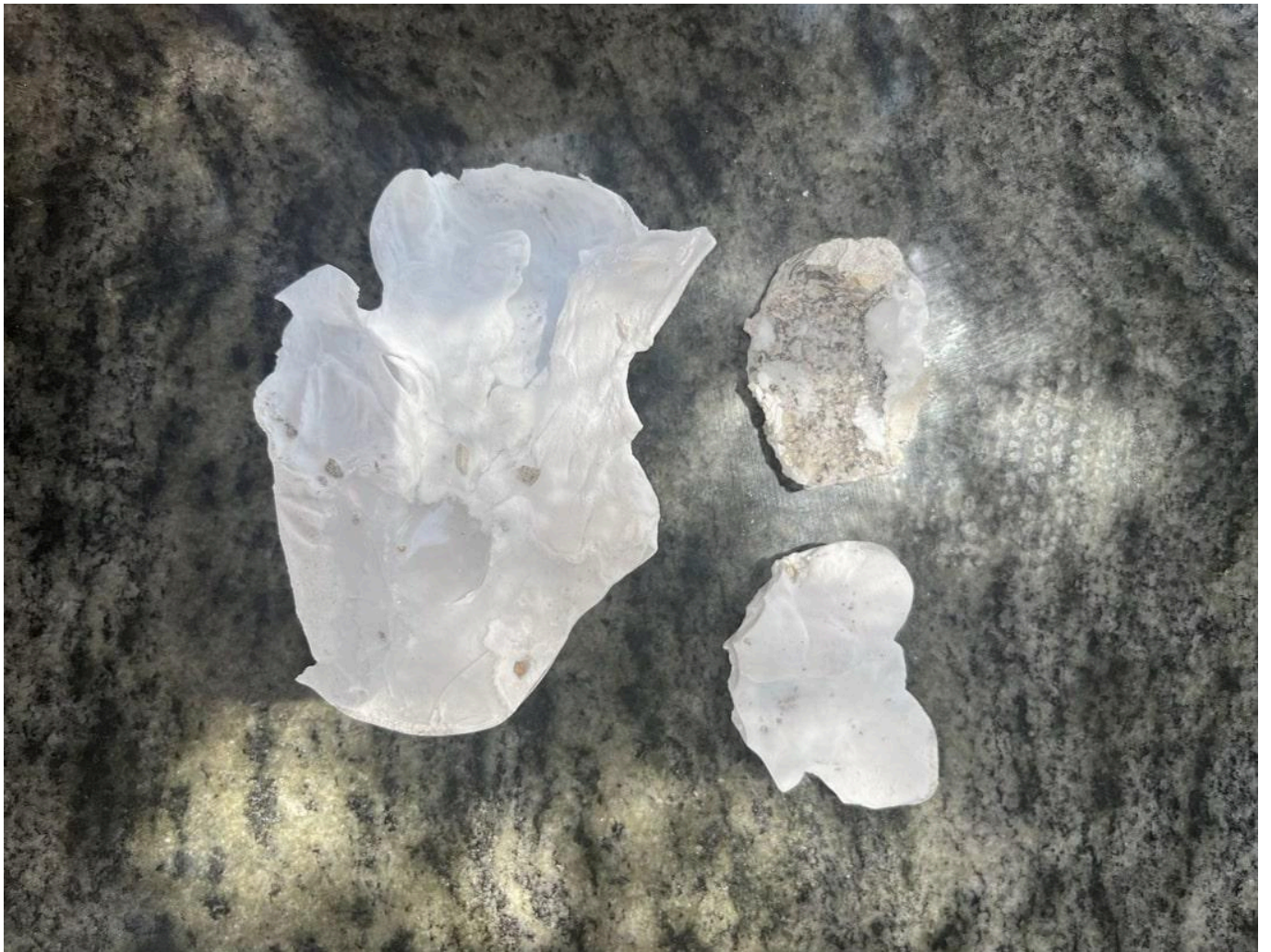
FIG 20. , GLASMA FULLY SEPARATED FROM THE CRUCIBLE. PHOTO BY SARAH MITCHELL.
