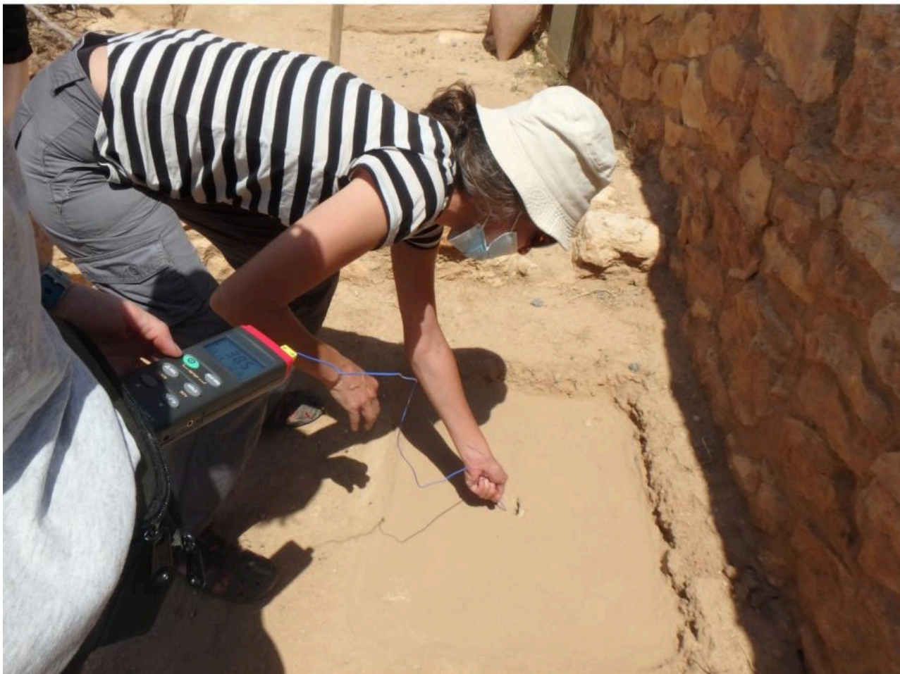
FIG 9. TEMPERATURE MEASUREMENTS. A. MEASURING TEMPERATURES IN HEARTH 1, WITH TWO TYPES OF DEVICES. B. PLACING THE DETECTOR OF A K-TYPE THERMOCOUPLE IN HEARTH 4.
