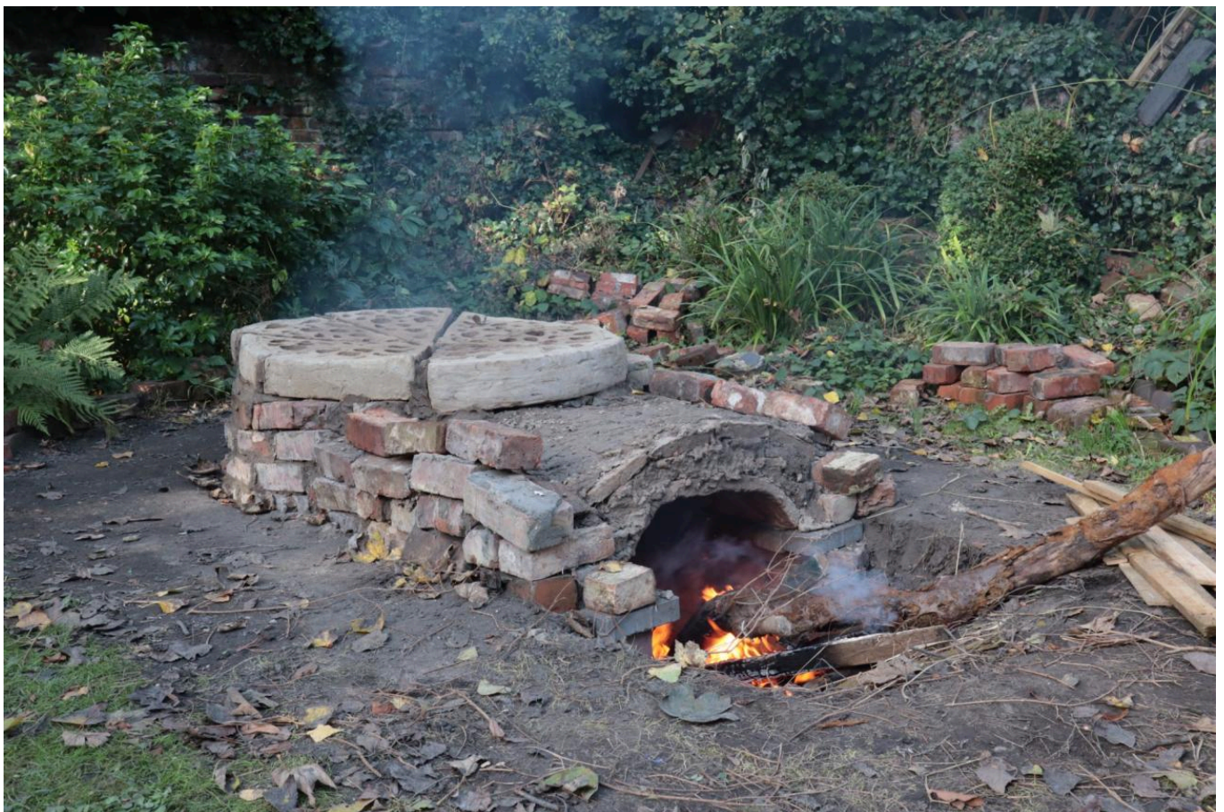
FIG 19. PRE-FIRING THE KILN UP TO 400°C. THE SMOKE COMING OUT OF THE PERFORATED FLOOR IS INDICATION OF GOOD DRAFT (TOMEI AND JIMÉNEZ RIVERO)
