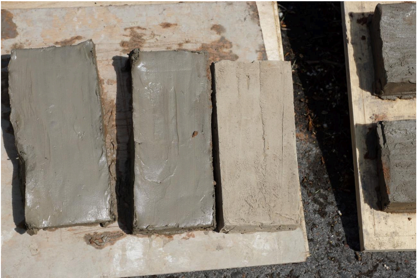
FIG 4. THE MUDBRICKS DRYING OUT UNDER THE SUN (TOMEI AND JIMÉNEZ RIVERO)
