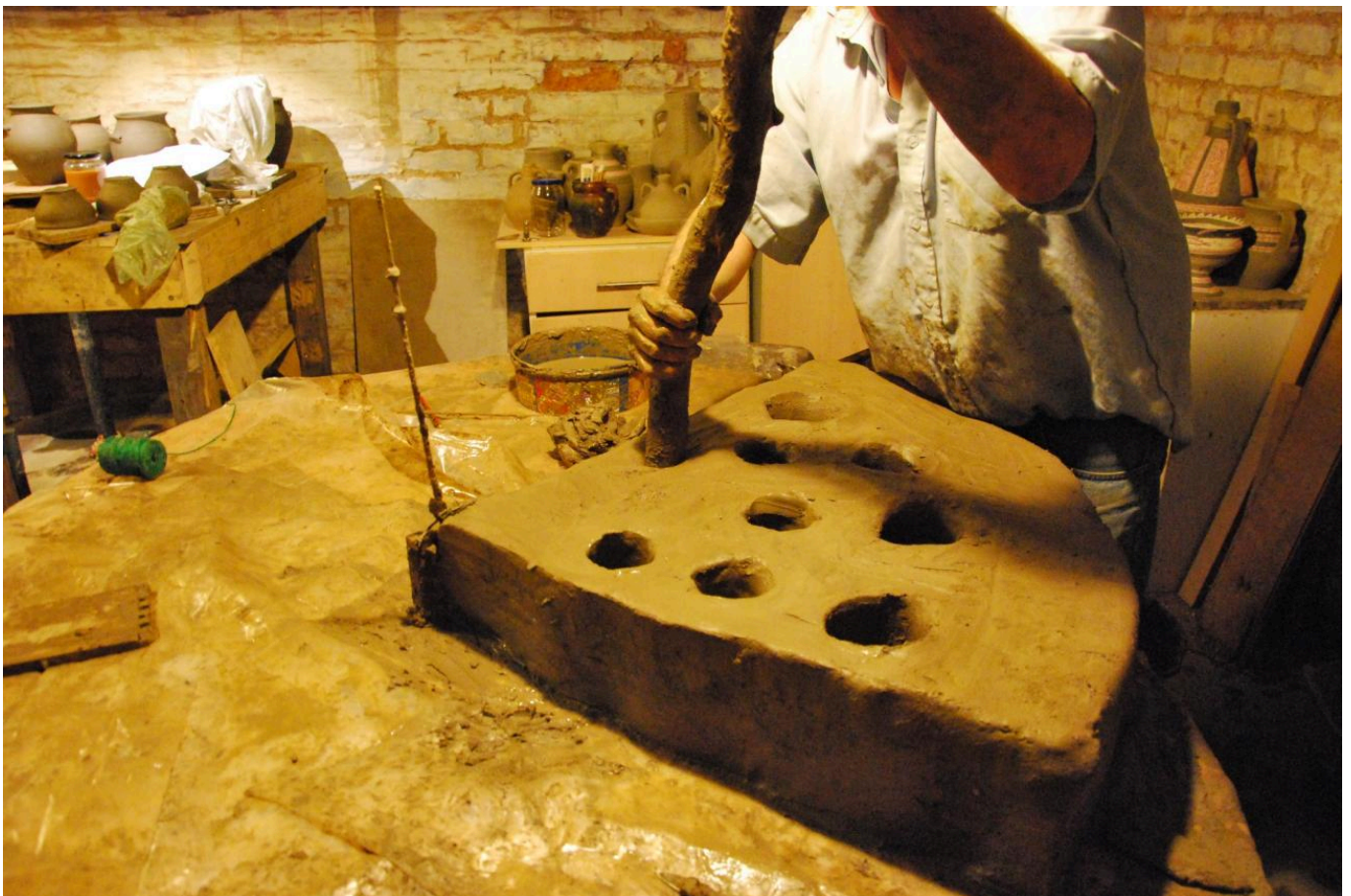
FIG 7. MAKING THE PERFORATED FLOOR. THE VENT HOLES ON EACH MODULE ARE MADE WITH A WOODEN ROD (TOMEI AND JIMÉNEZ RIVERO)
