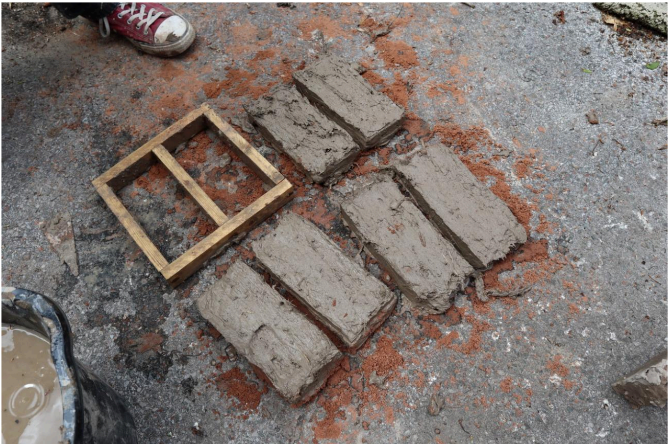
FIG 5. THE ADOBE BRICKS MADE OF CLAY TEMPERED WITH DRY STRAWS (TOMEI AND JIMÉNEZ RIVERO)
