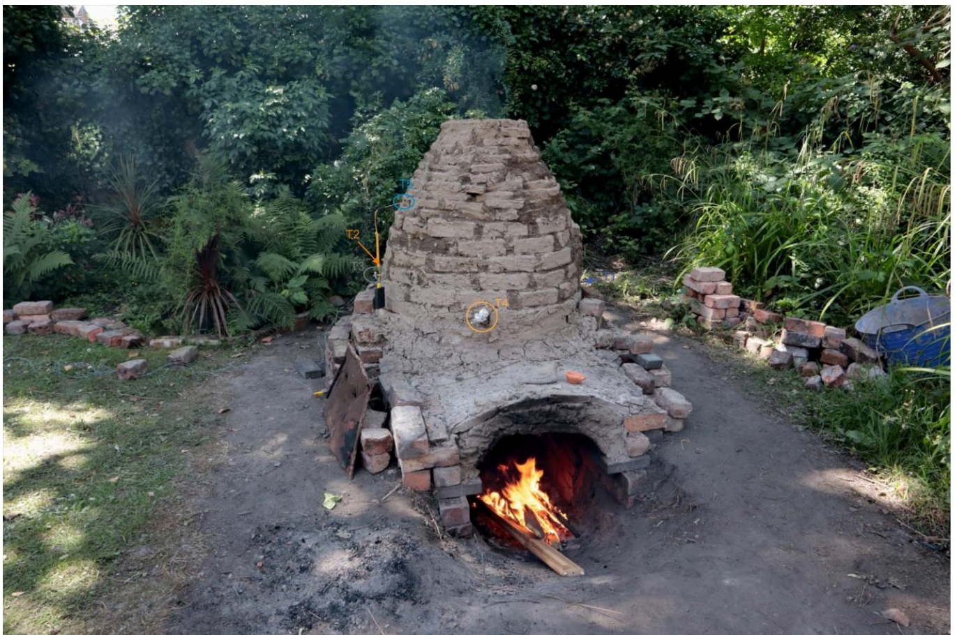
FIG 23. THE KILN DURING THE FIRST STAGES OF THE FIRING. FOUR THERMOCOUPLES MONITOR THE TEMPERATURE IN THE KILN (TOMEI AND JIMÉNEZ RIVERO)
