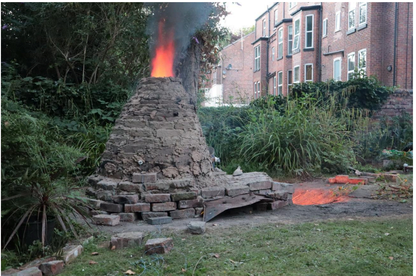
FIG 26. THE KILN WITH VIVID FLAMES AT 800-900°C (TOMEI AND JIMÉNEZ RIVERO)
