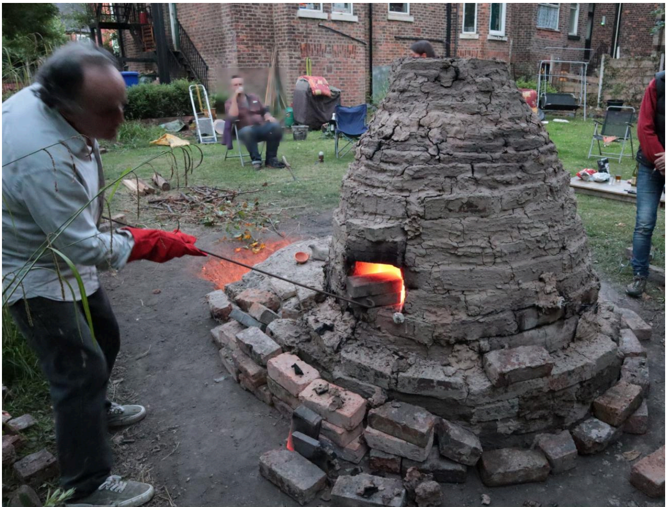
FIG 27. TAKING A SAMPLE FROM THE TEST WINDOW USING THE HOOKED TOOL (TOMEI AND JIMÉNEZ RIVERO)
