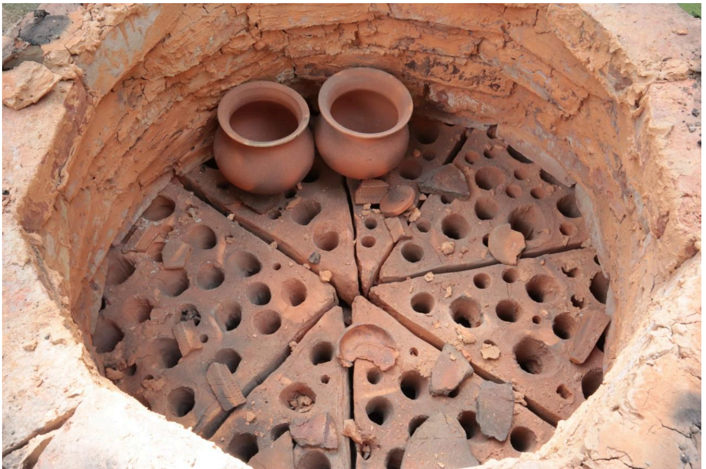
FIG 31. THE PERFORATED FLOOR AFTER THE FIRING (TOMEI AND JIMÉNEZ RIVERO)
