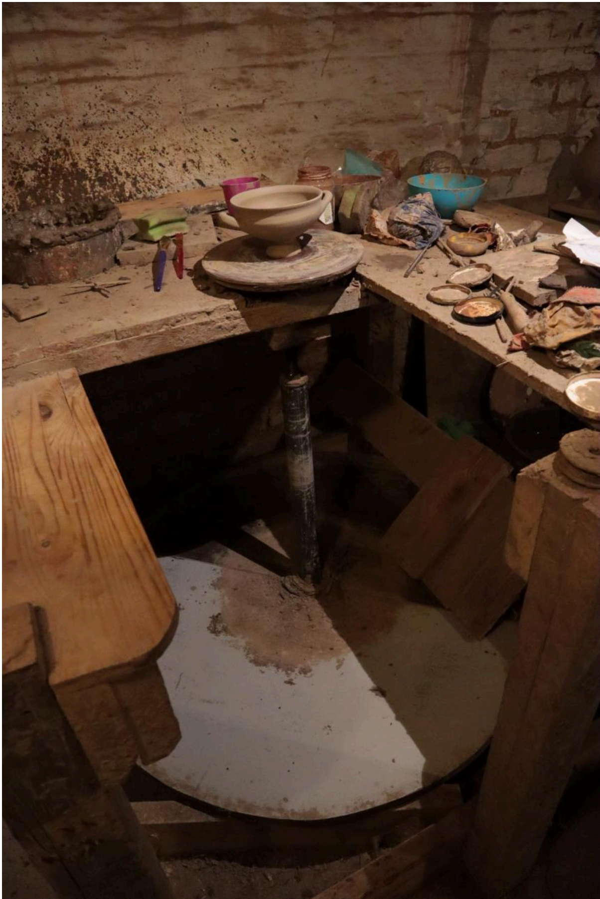
FIG 9. WHEEL-THROWING A IONIC CUP WITH A TRADITIONAL CASTILLAN KICK WHEEL (TOMEI AND JIMÉNEZ RIVERO)
