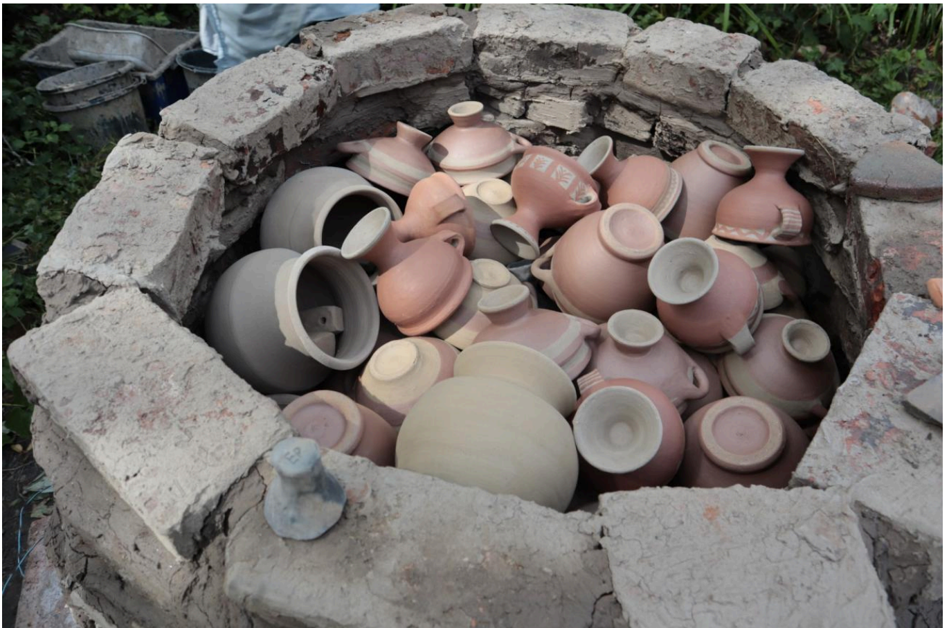
FIG 21. STACKING THE FIRING CHAMBER WITH THE COARSE WARES AT THE BASE AND THE FINE PAINTED VESSELS ABOVE THEM. LOOM WEIGHTS WORK AS KILN SPACERS (TOMEI AND JIMÉNEZ RIVERO)
