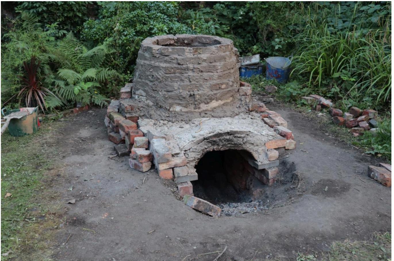
FIG 20. THE FIRING CHAMBER MADE OF VICTORIAN BRICKS AND CLAY CEMENT (TOMEI AND JIMÉNEZ RIVERO)
