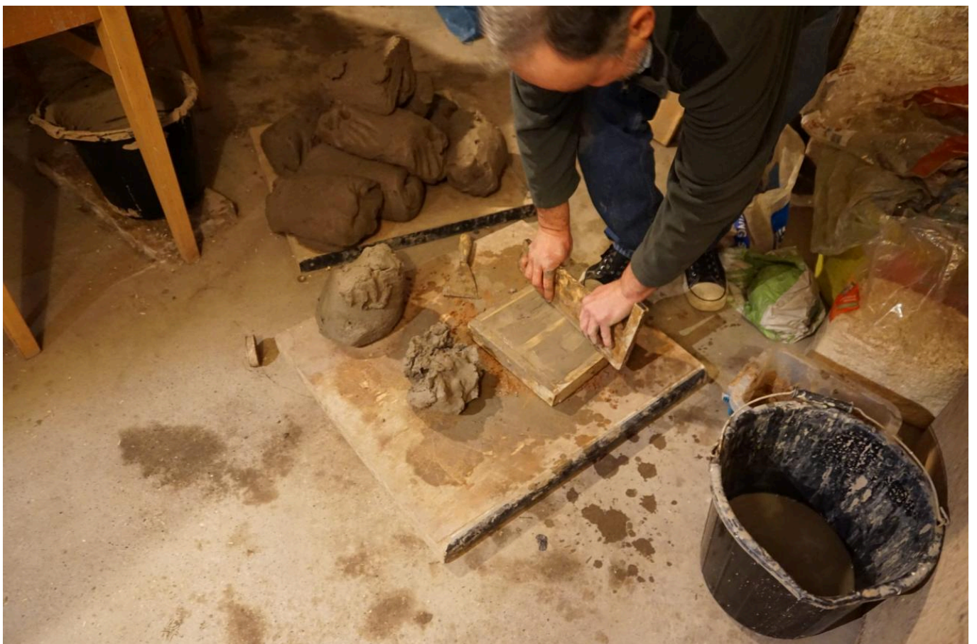
FIG 3. MAKING THE MUDBRICKS WITH A WOODEN FRAME (TOMEI AND JIMÉNEZ RIVERO)
