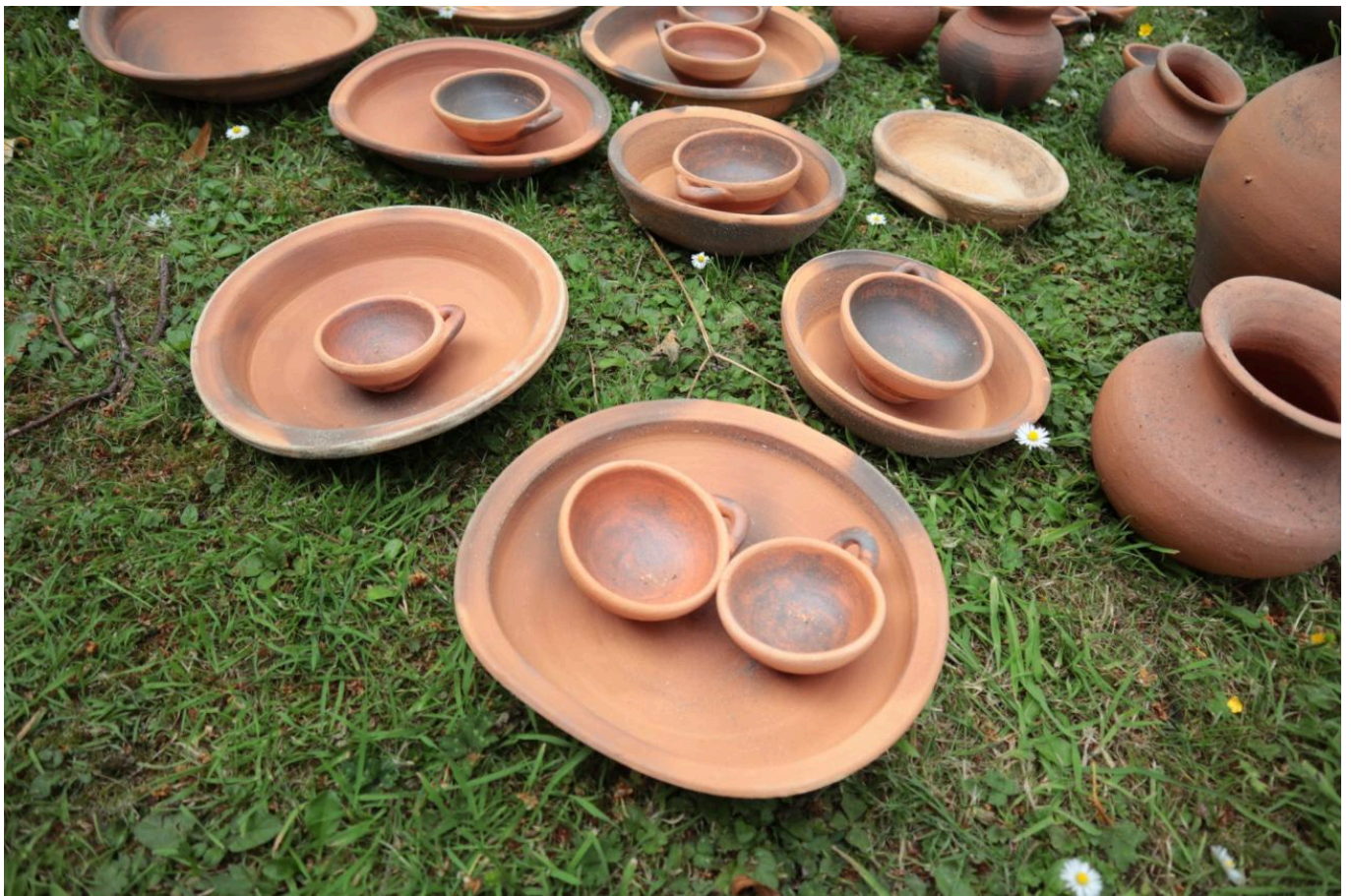
FIG 29. PANS WITH MINOR SIGNS OF MISFIRING (TOMEI AND JIMÉNEZ RIVERO)
