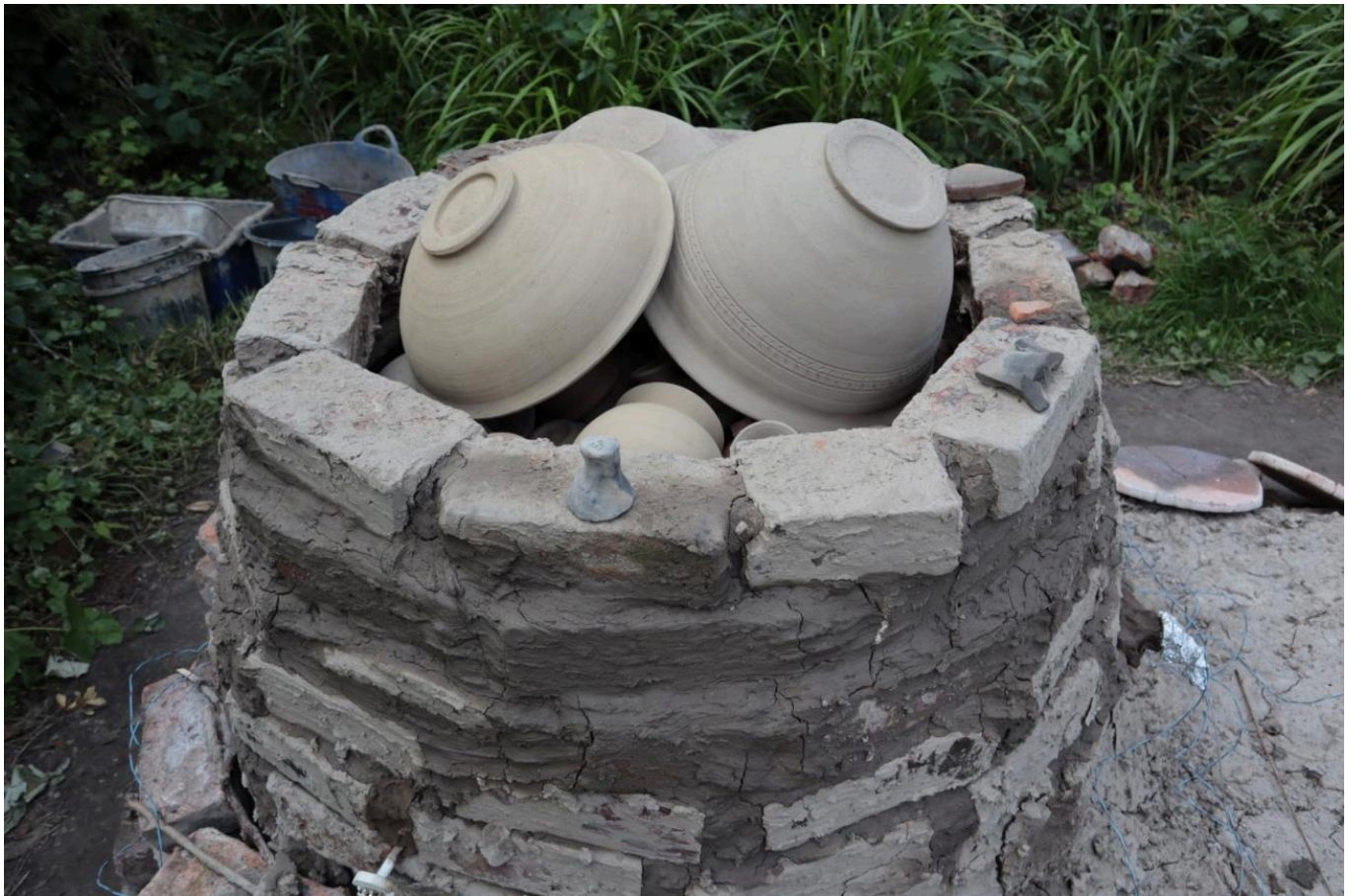
FIG 22. THE LARGE BASINS ARE PLACED UPSIDE DOWN ON THE TOP OF THE LOAD TO RETAIN HEAT (TOMEI AND JIMÉNEZ RIVERO)
