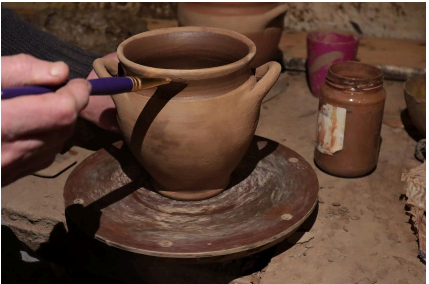
FIG 10. APPLYING THE SIGILLATA SLIP ON SEVERAL COATING BY BRUSHING (TOMEI AND JIMÉNEZ RIVERO)
