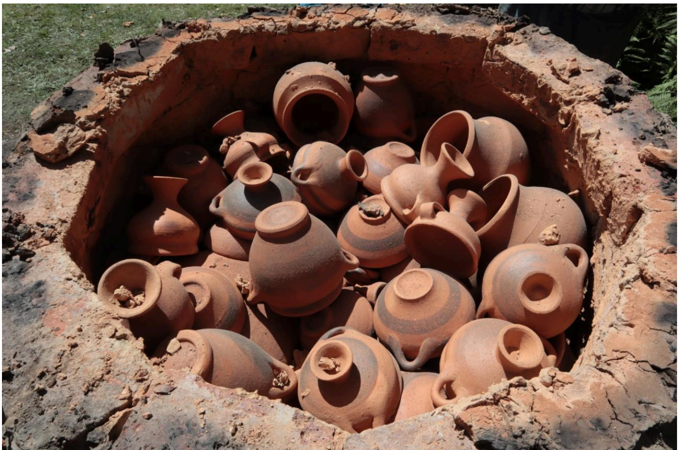
FIG 28. THE POTTERY LOAD AFTER OPENING THE TEMPORARY DOME (TOMEI AND JIMÉNEZ RIVERO)
