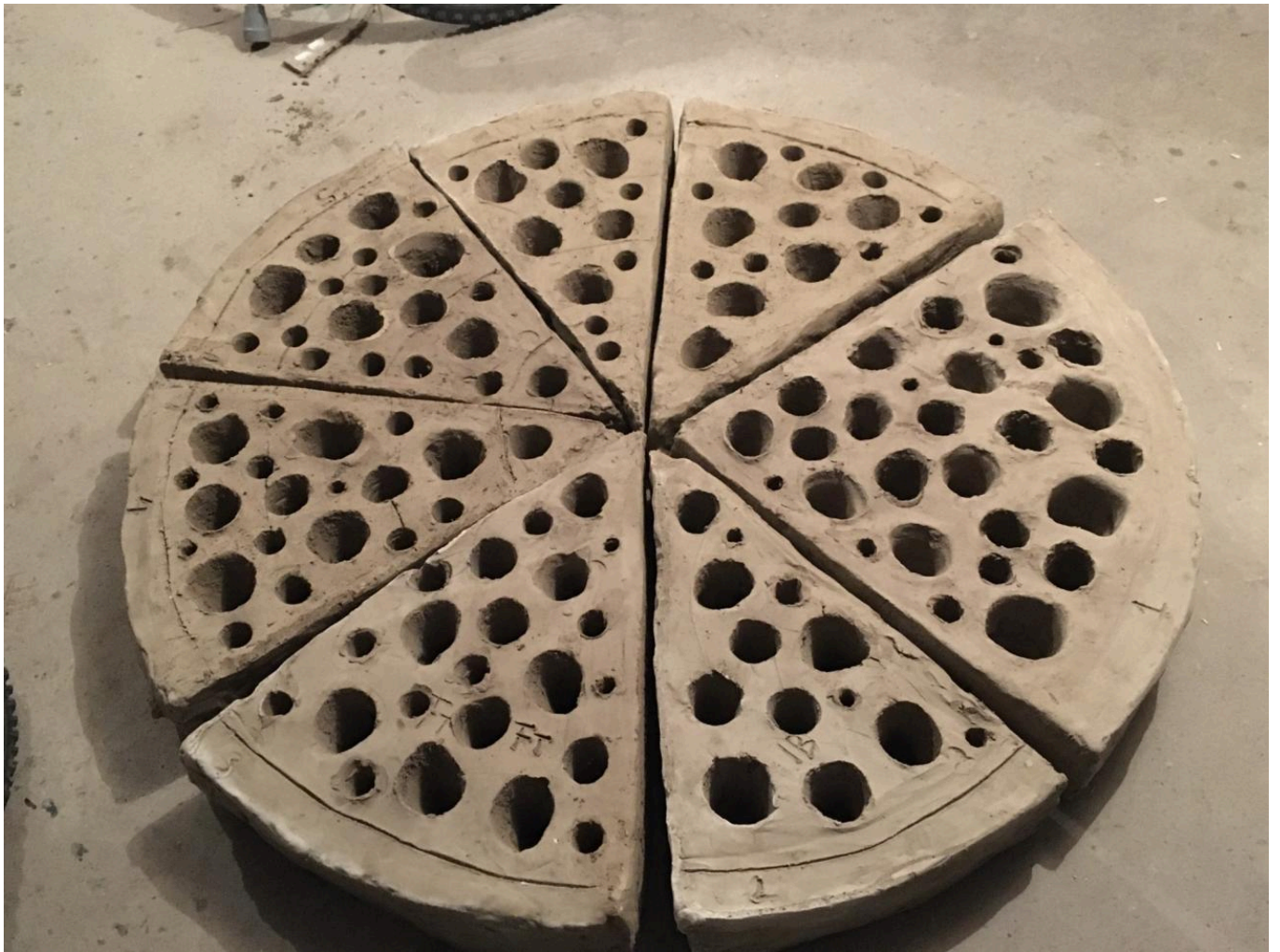
FIG 8. THE PERFORATED FLOOR COMPLETED AND DRIED OUT (TOMEI AND JIMÉNEZ RIVERO)
