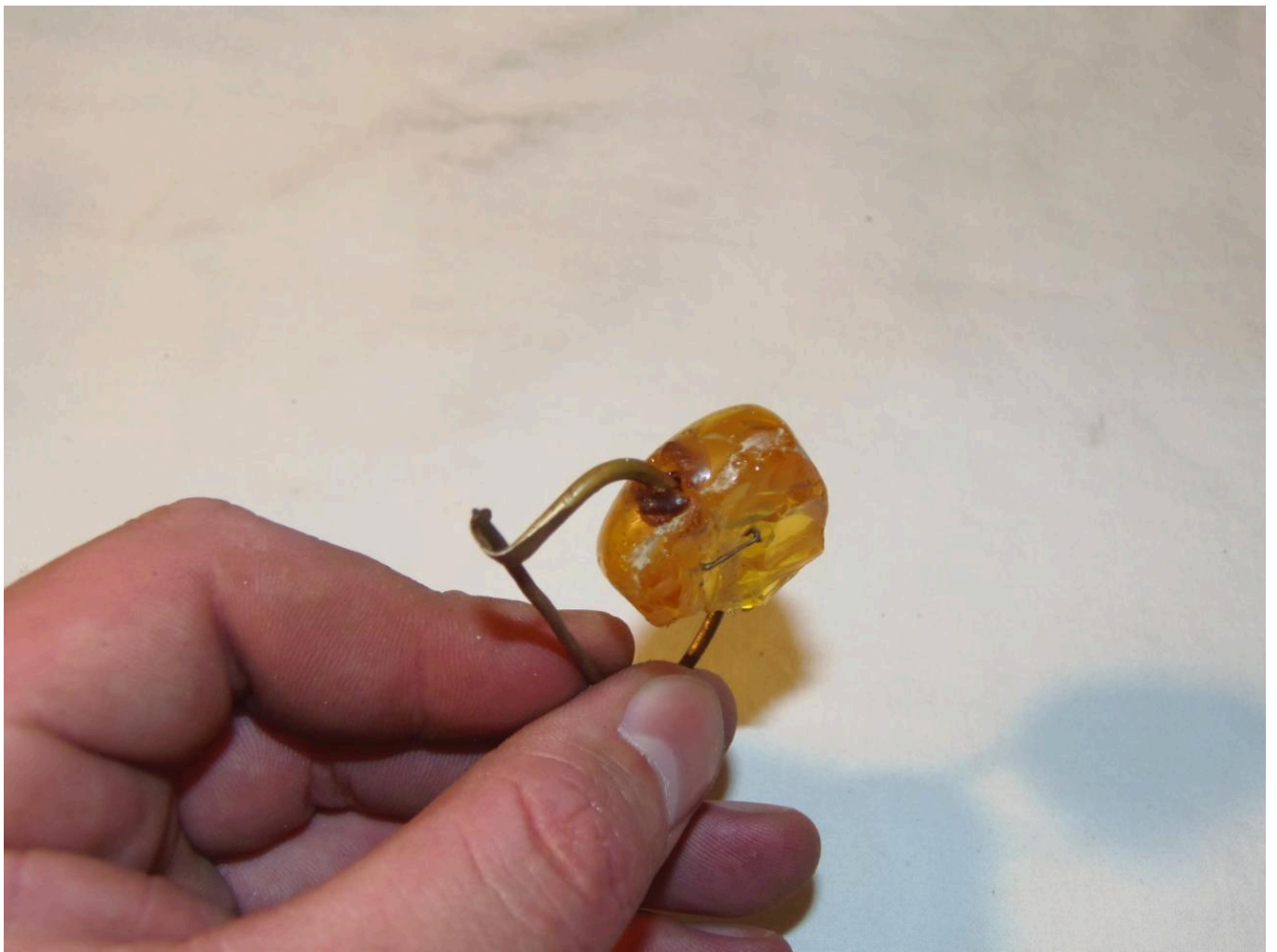
FIG 17. LUMPS OF MOLTEN AMBER CLOSE TO THE ENTRY HOLE IN THIS SMALL CORE. PHOTO BY MAURO FIORENTINI
