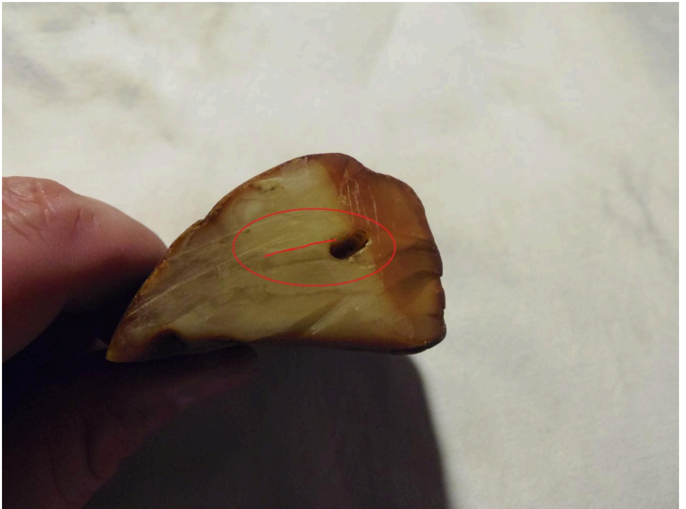
FIG 16. THE RED MARKS SHOW THE SUBTLE SLIT THAT OPENED WHILE PIERCING THE PIECE. PHOTO BY MAURO FIORENTINI
