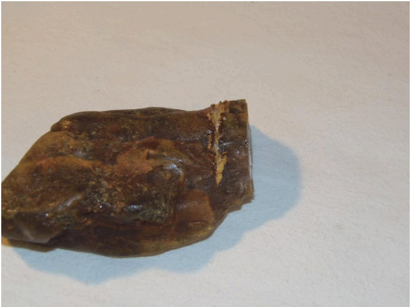
FIG 9. EVIDENT LUMPS OF MOLTEN AMBER LEFT BY THE RED-HOT KNIFE BLADE. PHOTO BY MAURO FIORENTINI
