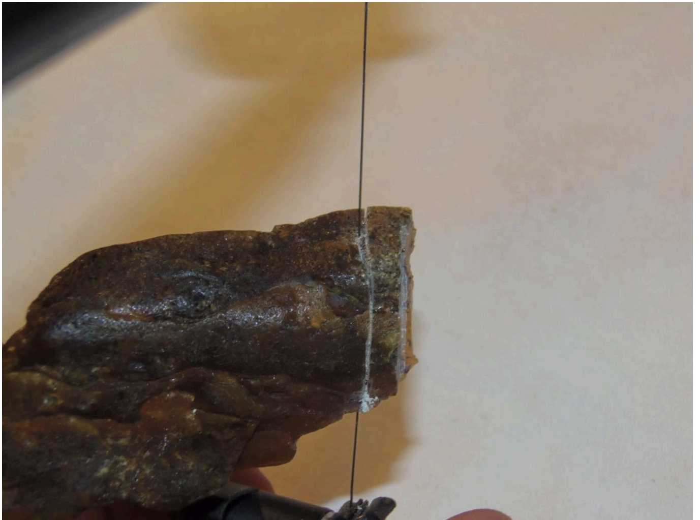
FIG 7. SHOWING INACCURACY IN THE CUT WITH THE WIRE HACKSAW. PHOTO BY MAURO FIORENTINI
