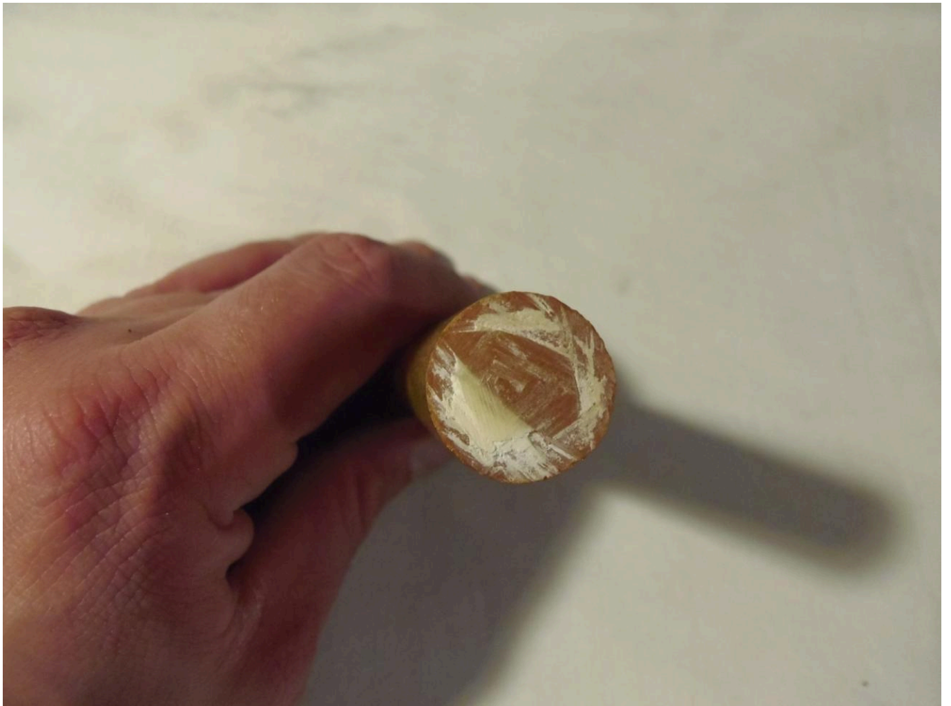
FIG 10. TRACES OF HACKSAW FOR METALS LEFT ON THIS CYLINDRICAL SEMI-WORKED PIECE. PHOTO BY MAURO FIORENTINI
