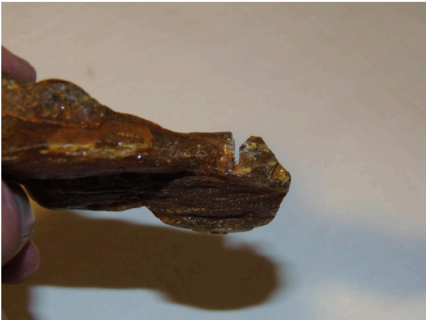
FIG 6. ZOOM ON THE CUT BEING CARRIED OUT WITH THE HACKSAW FOR METALS. PHOTO BY MAURO FIORENTINI
