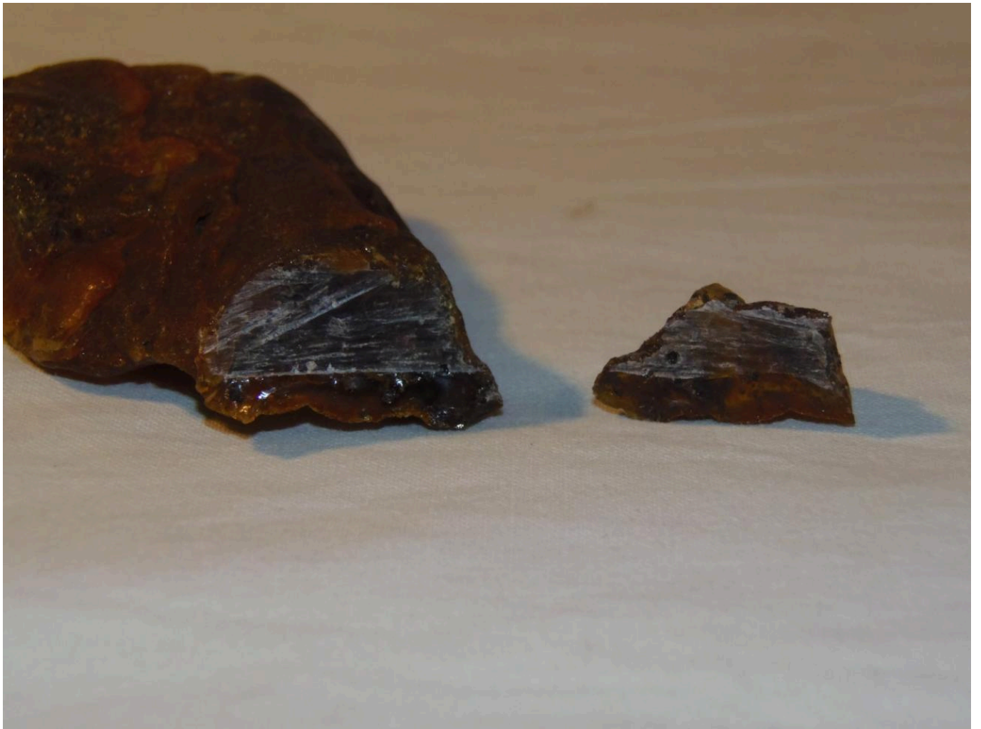
FIG 5. EVIDENT TRACES LEFT ON THE AMBER BY THE HACKSAW FOR METALS. PHOTO BY MAURO FIORENTINI
