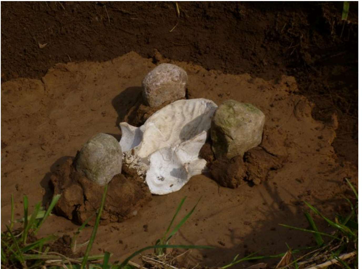
FIG 10. CONSTRUCTION STEP 1 FOR TAR PIT, CLOSED DISTILLATION.
