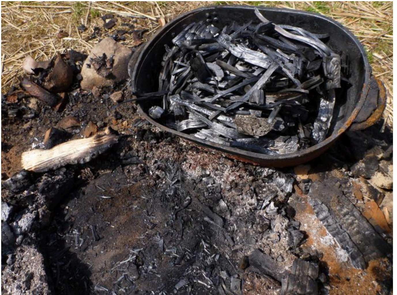
FIG 19. PINE WOOD TURNED INTO CHAR COAL AFTER FIRING.
