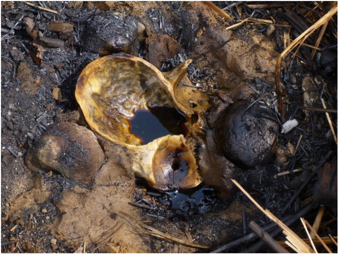
FIG 16. TAR IN THE DEER SKULL AFTER OPENING THE CLOSED DISTILLATION.
