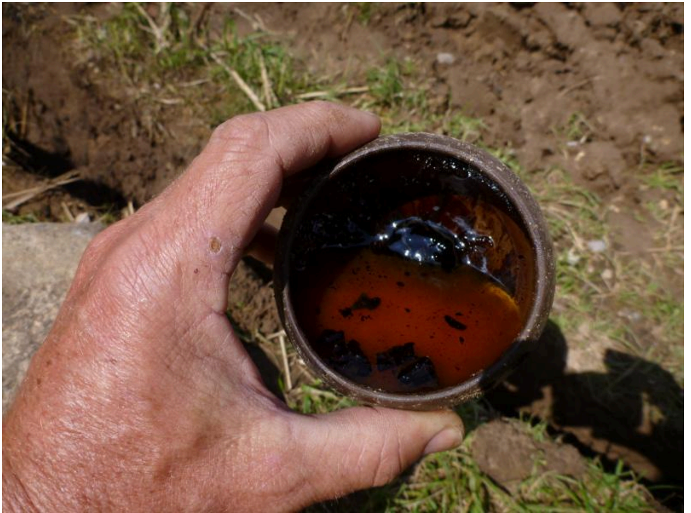
FIG 20. WATERY AS WELL AS TAR FLUIDS ARE THE RESULTS OF THE PINE WOOD DISTILLATION.
