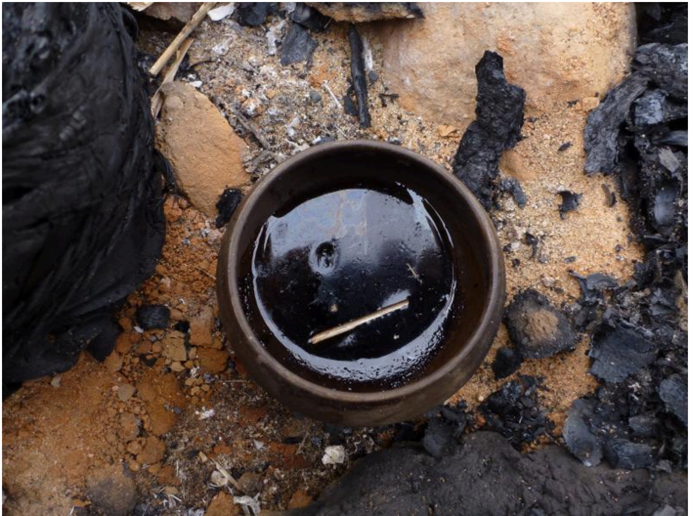
FIG 8. PITCH AFTER HEATING THE BIRCH BARK TAR FROM THE OPEN DISTILLERY.
