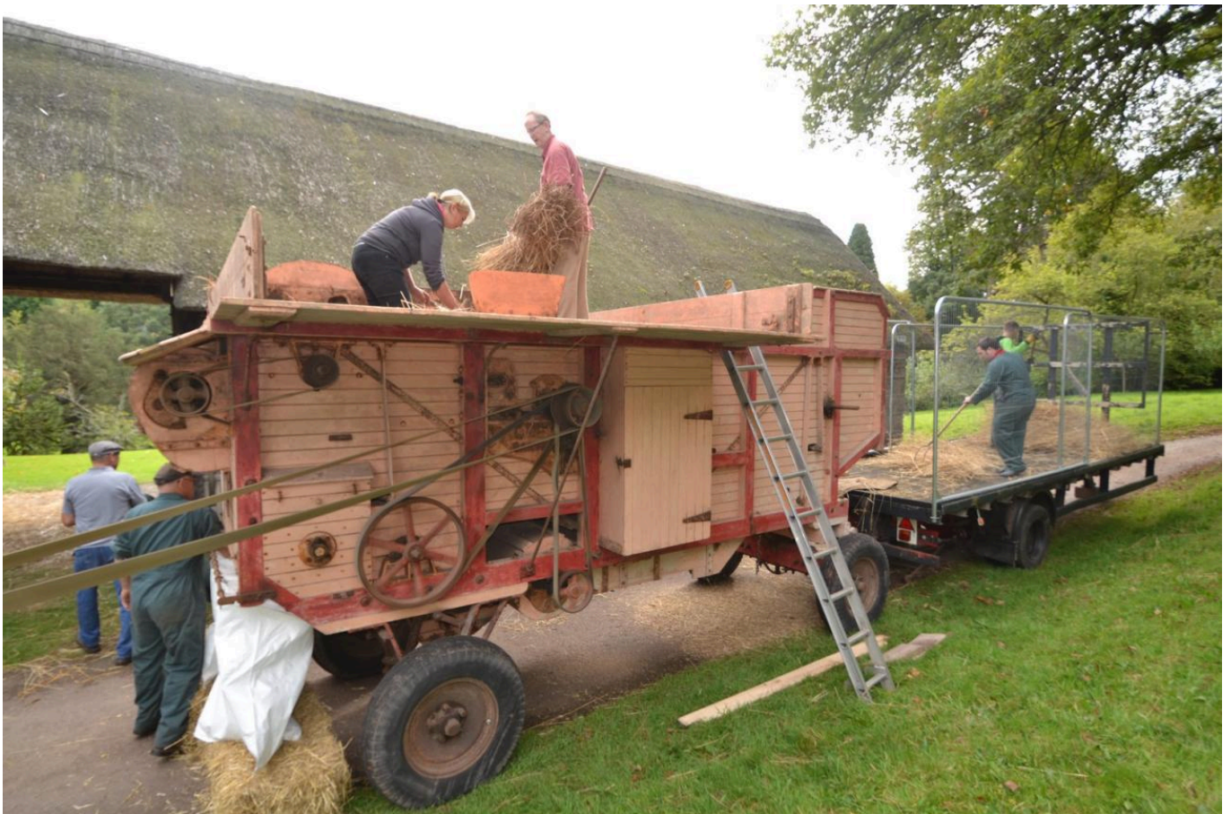
FIG 11. THRESHING MACHINE USED TO REMOVE THE HEADS FROM THE WHEAT, HAVING EXPLORED OTHER THRESHING METHODS, AS DETAILED IN THE TEXT.
