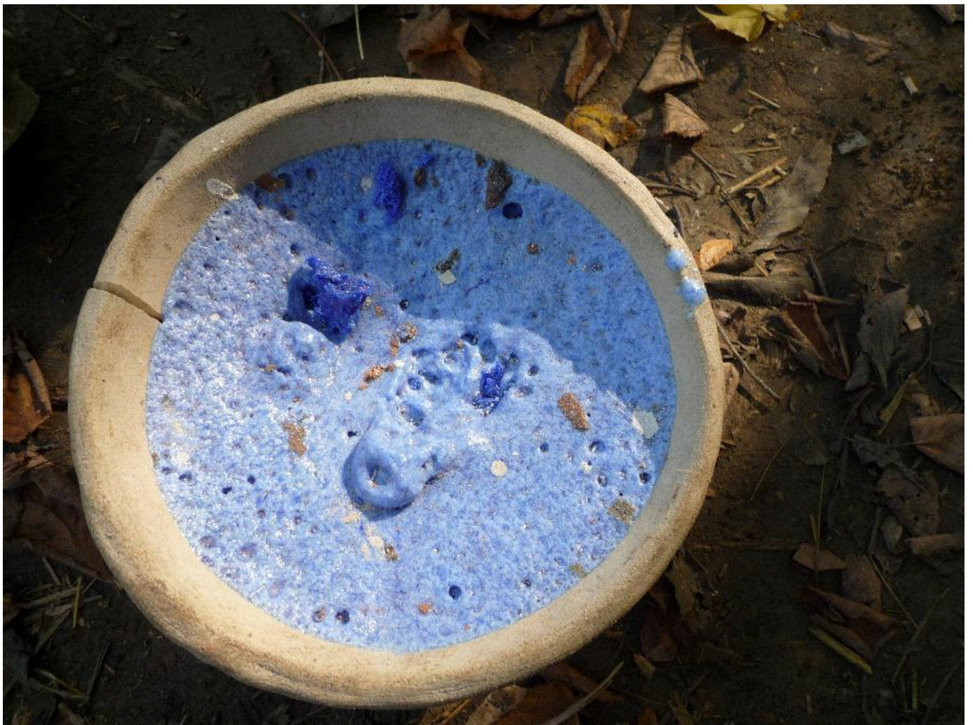
FIG 5. CRUCIBLE WITH A FAILED GLASS BATCH; BAKING SODA HAD BEEN USED BY MISTAKE
