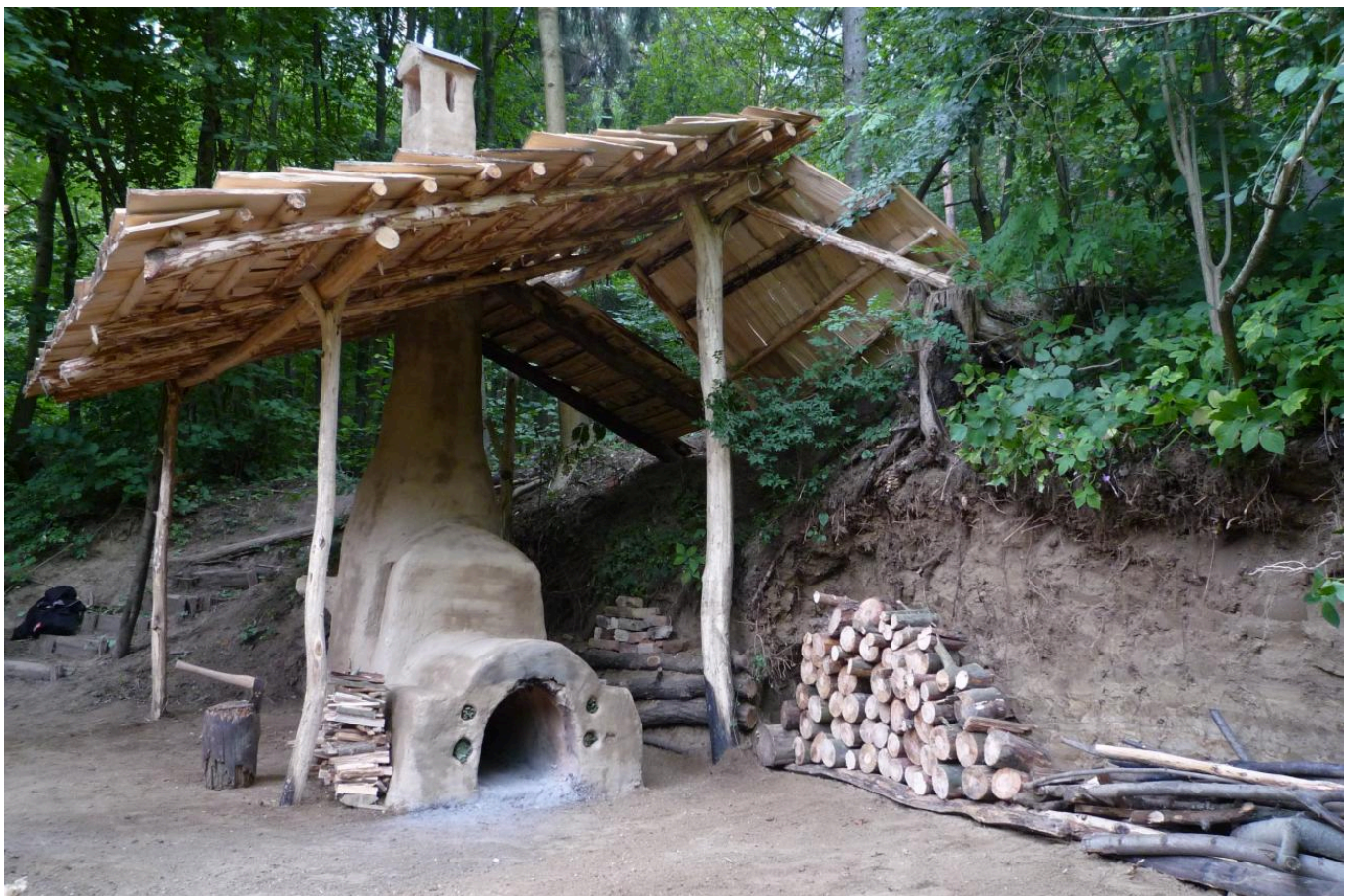
FIG 4. THE COMPLETED GLASS FURNACE WITH A TOTAL HEIGHT OF 4 M
