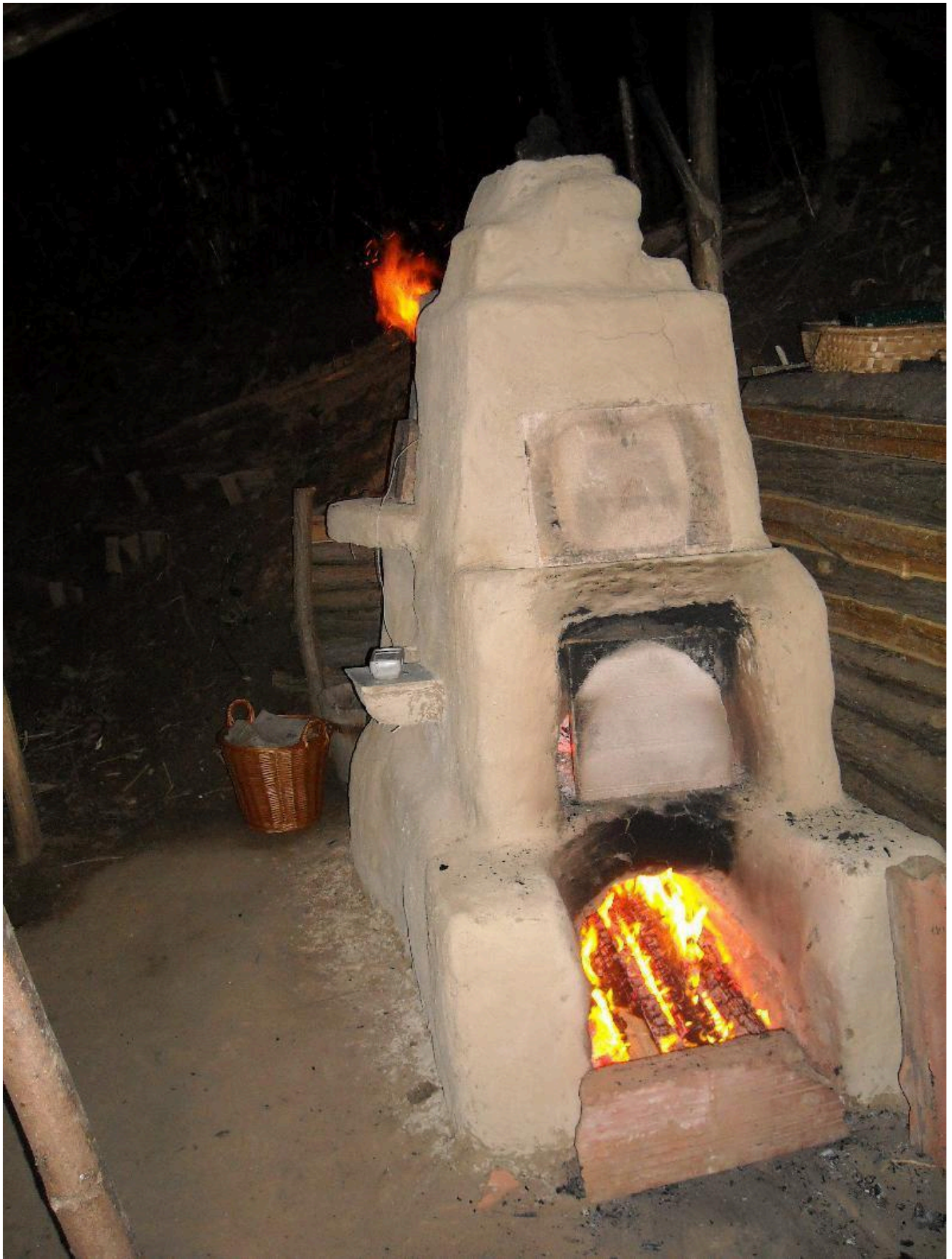
FIG 10. THE NEW GLASS OVEN WITH A SEPARATE COOLING OVEN
