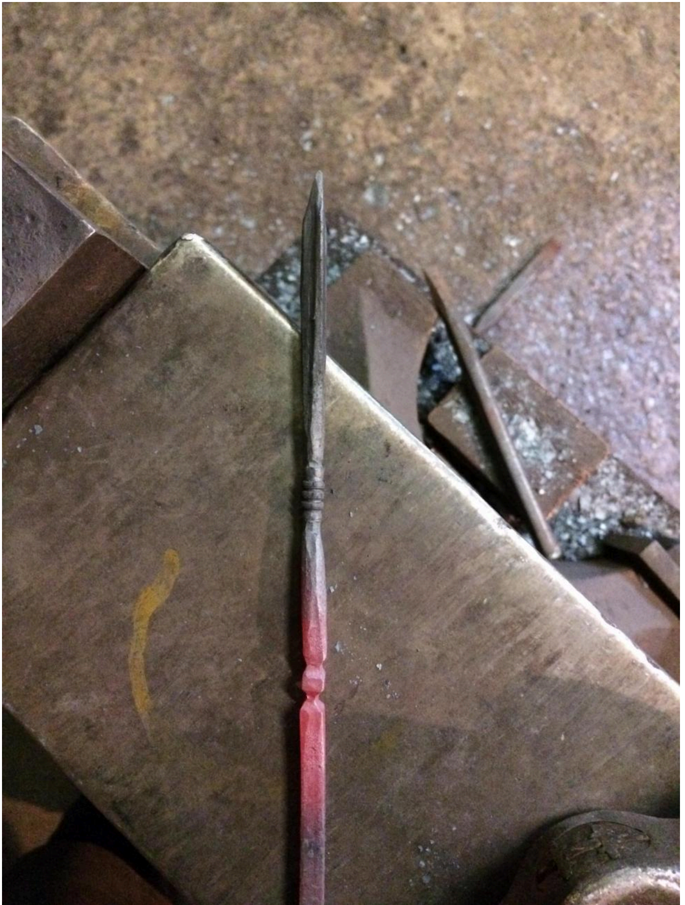
FIG 15. FORGING CUT OFF POINT OF THE TANG. PHOTO BY HECTOR COLE
