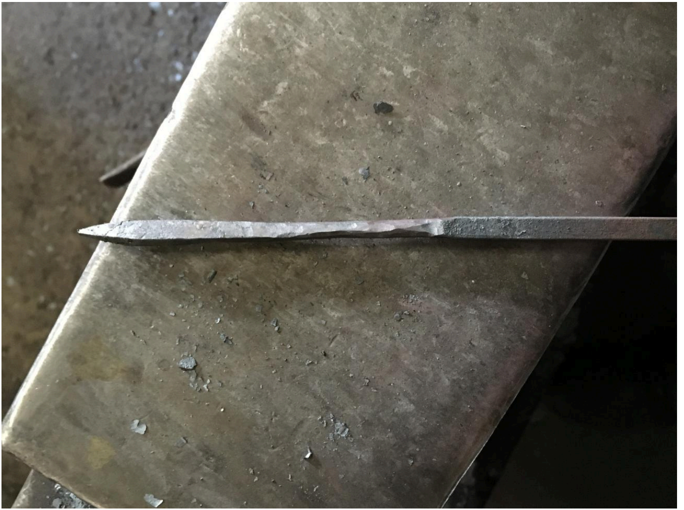
FIG 26. FORGING NECK TO LENGTH. PHOTO BY HECTOR COLE
