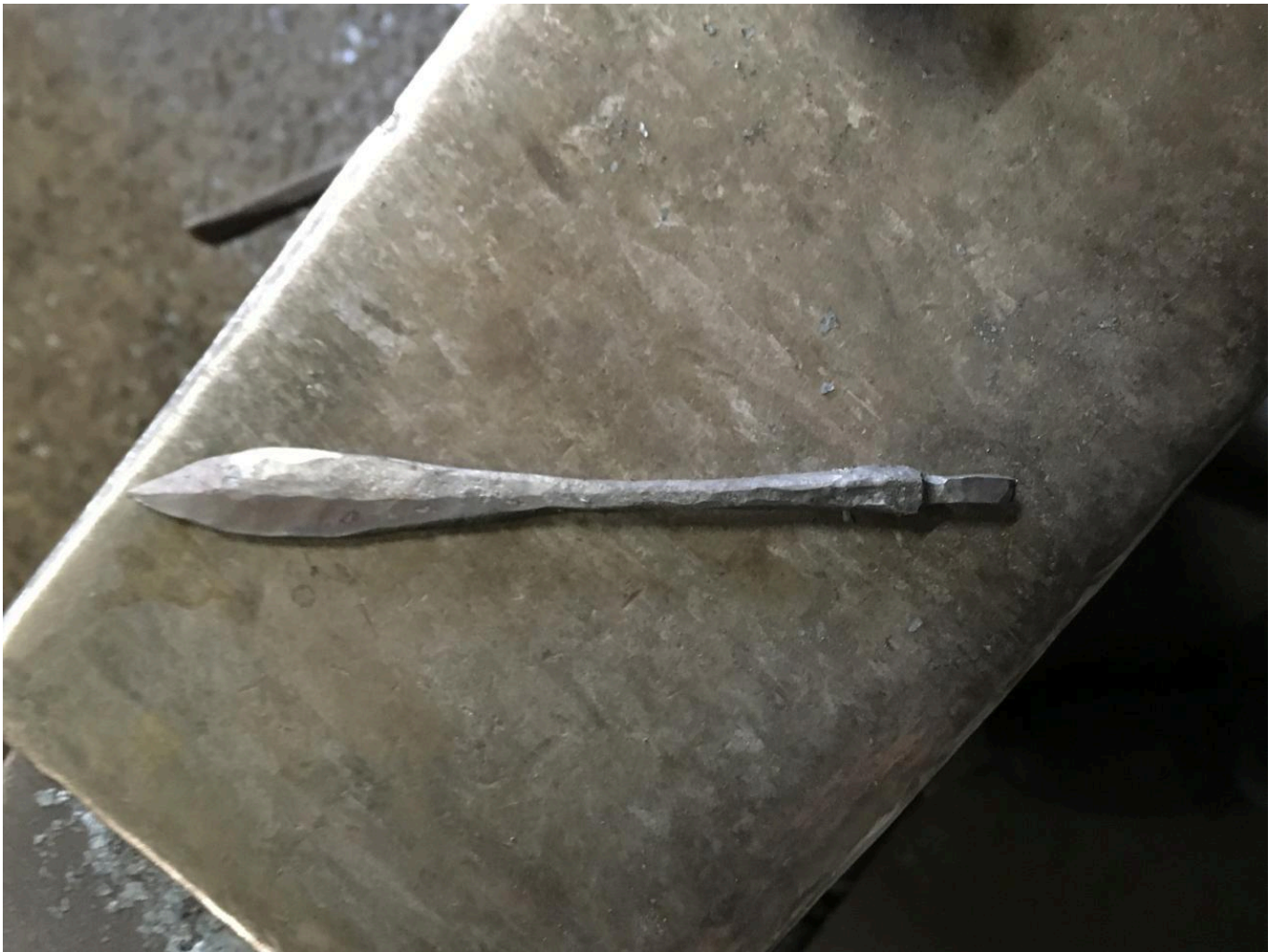
FIG 30. FORGING TANG. PHOTO BY HECTOR COLE
