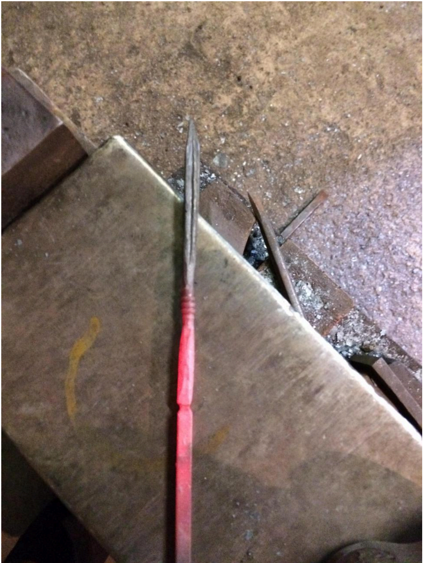
FIG 14. FORGING SHOULDER OF THE TANG. PHOTO BY HECTOR COLE
