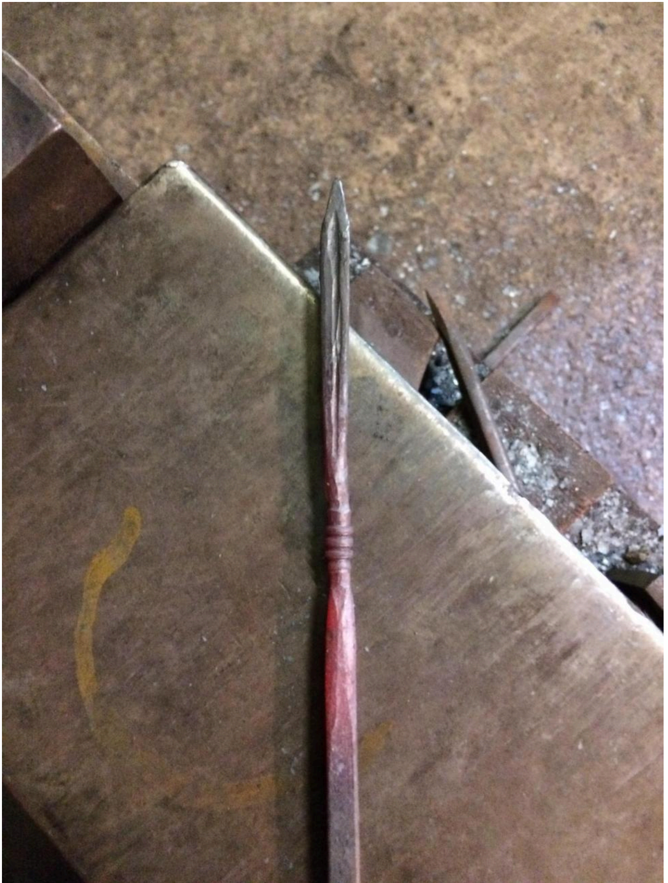
FIG 13. FORGING IN THE GROOVES ON THE BLADE. PHOTO BY HECTOR COLE
