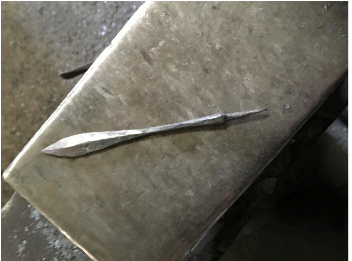
FIG 31. FORGING OF HEAD COMPLETED. PHOTO BY HECTOR COLE
