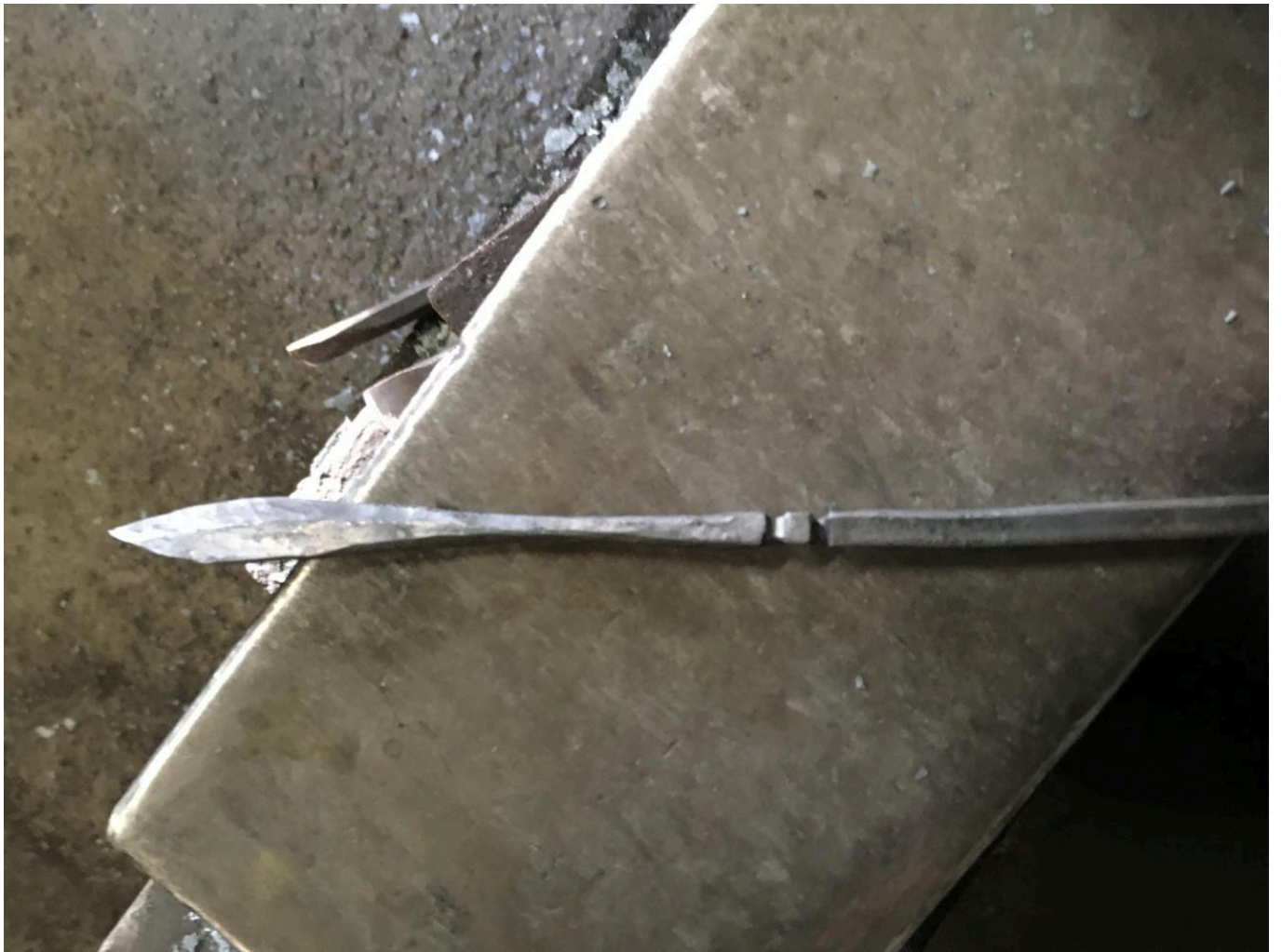
FIG 29. NECKING AND MARKING TANG. PHOTO BY HECTOR COLE
