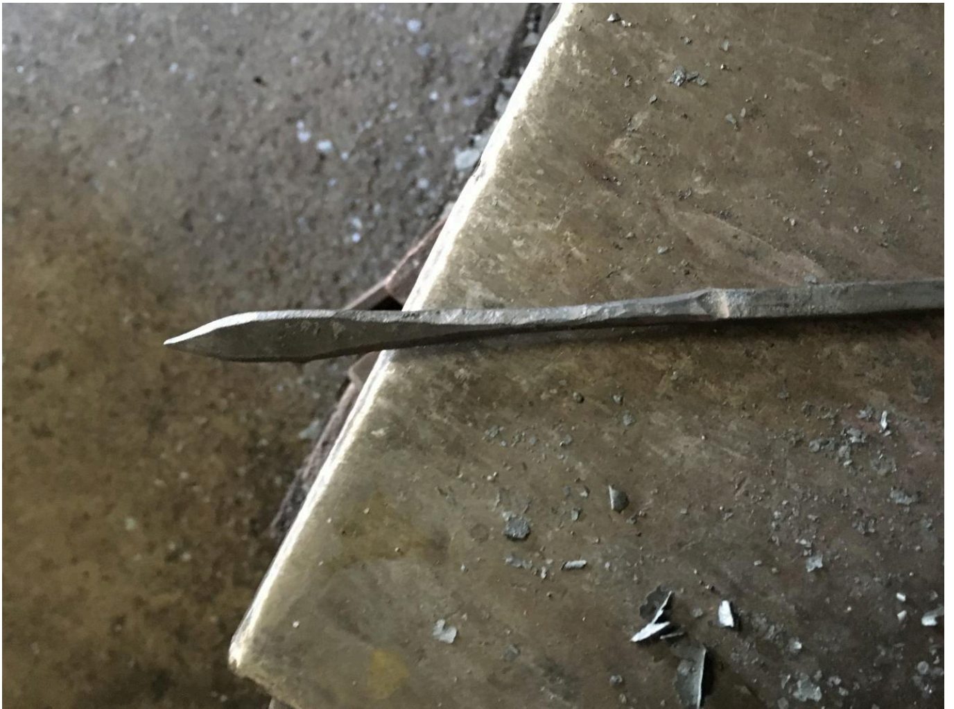
FIG 27. FLATTENING OUT BLADE. PHOTO BY HECTOR COLE
