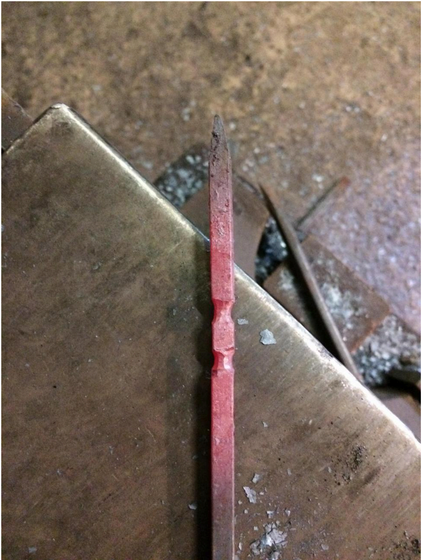
FIG 9. NECKING IN RING POSITIONS. PHOTO BY HECTOR COLE
