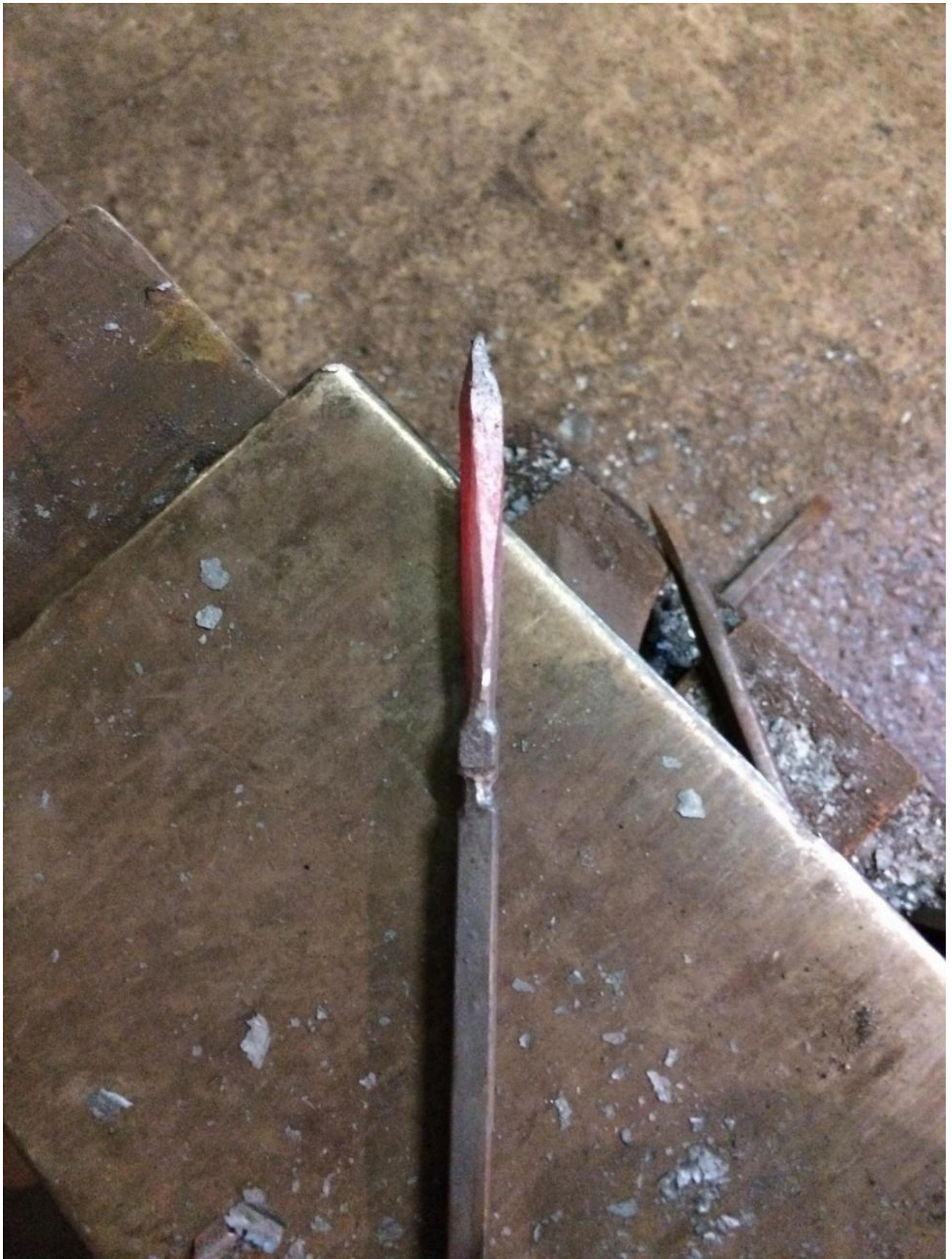
FIG 10. FORGING THE SHANK TO THE BLADE. PHOTO BY HECTOR COLE
