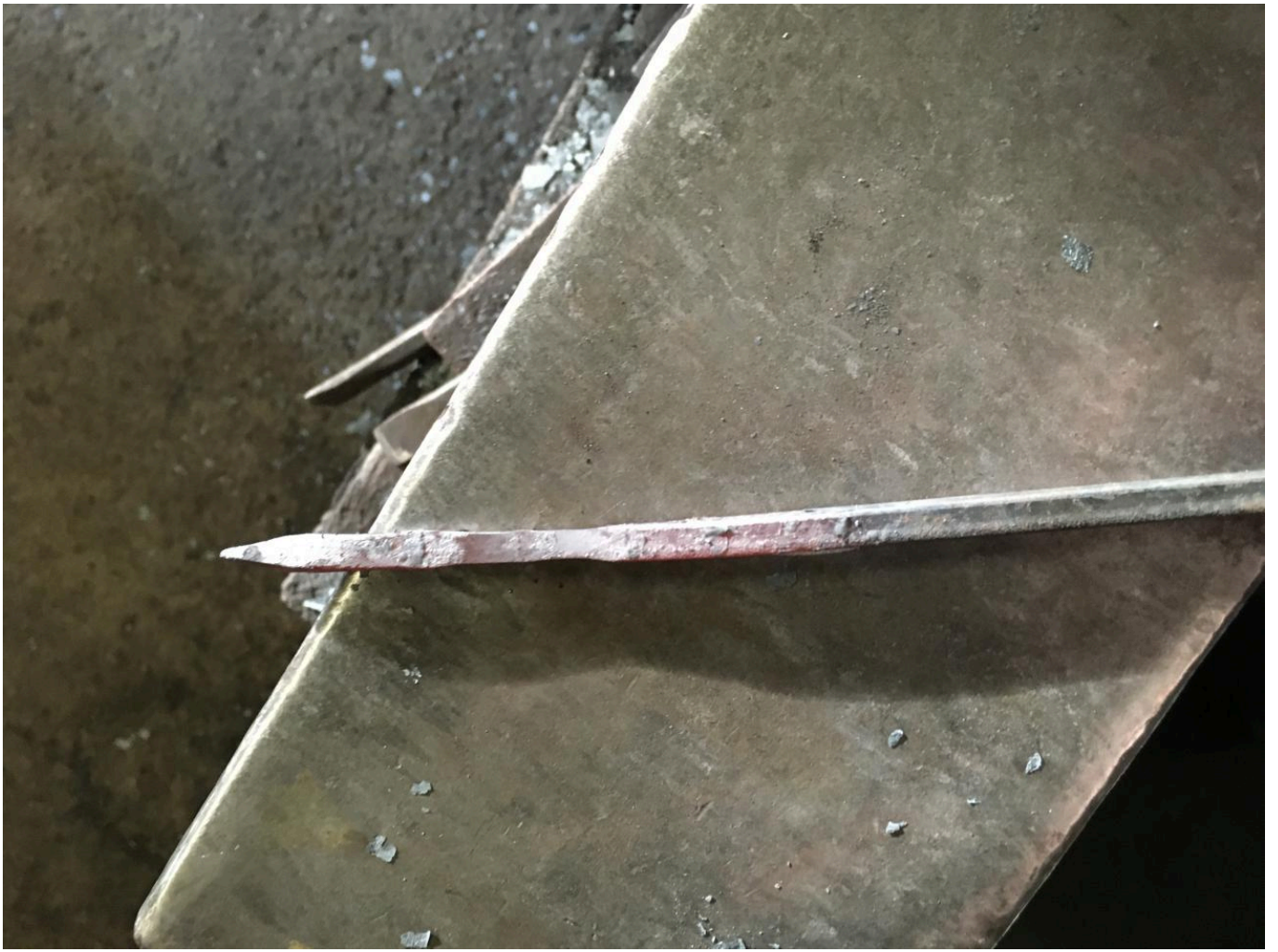
FIG 25. FORGING IN NECK. PHOTO BY HECTOR COLE
