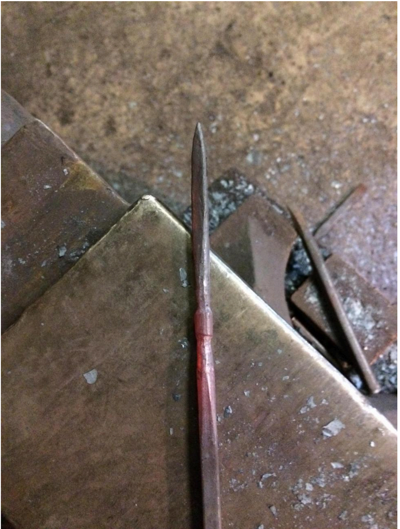
FIG 11. FORGING THE BLADE TO TRIANGULAR SECTION. PHOTO BY HECTOR COLE
