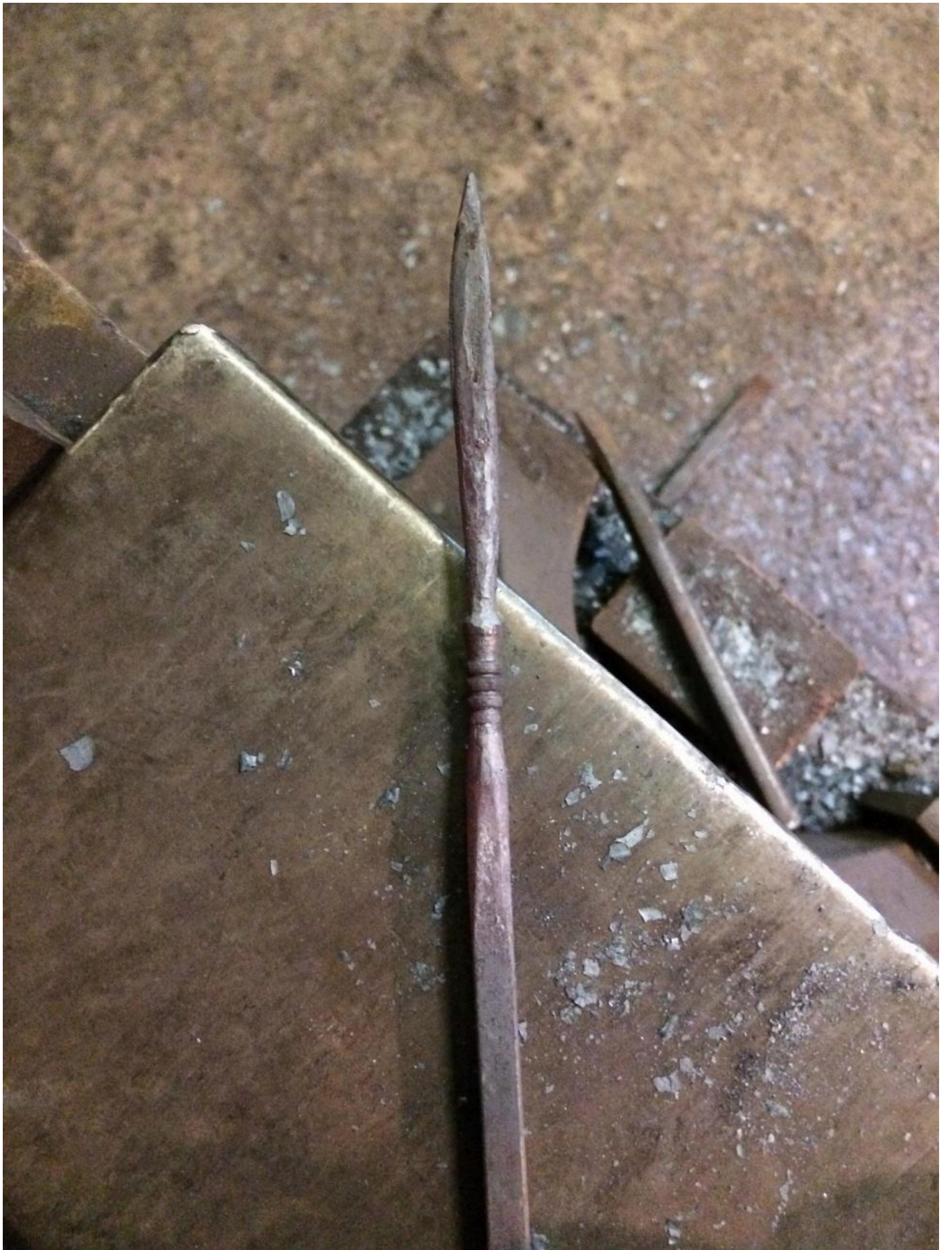
FIG 12. FORGING IN THE RINGS ON THE SHANK. PHOTO BY HECTOR COLE
