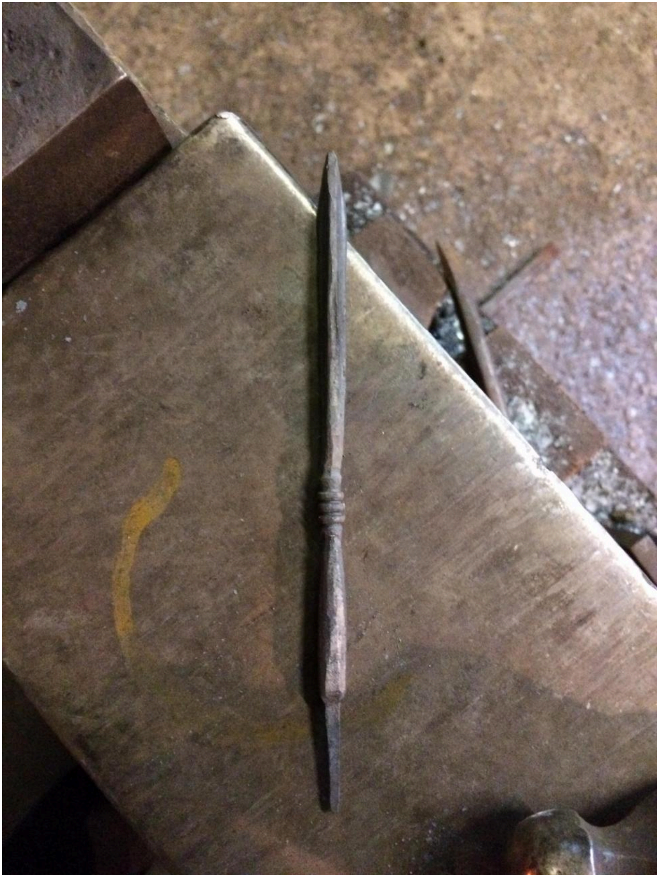
FIG 16. FORGED HEAD PRIOR TO FINISHING. PHOTO BY HECTOR COLE
