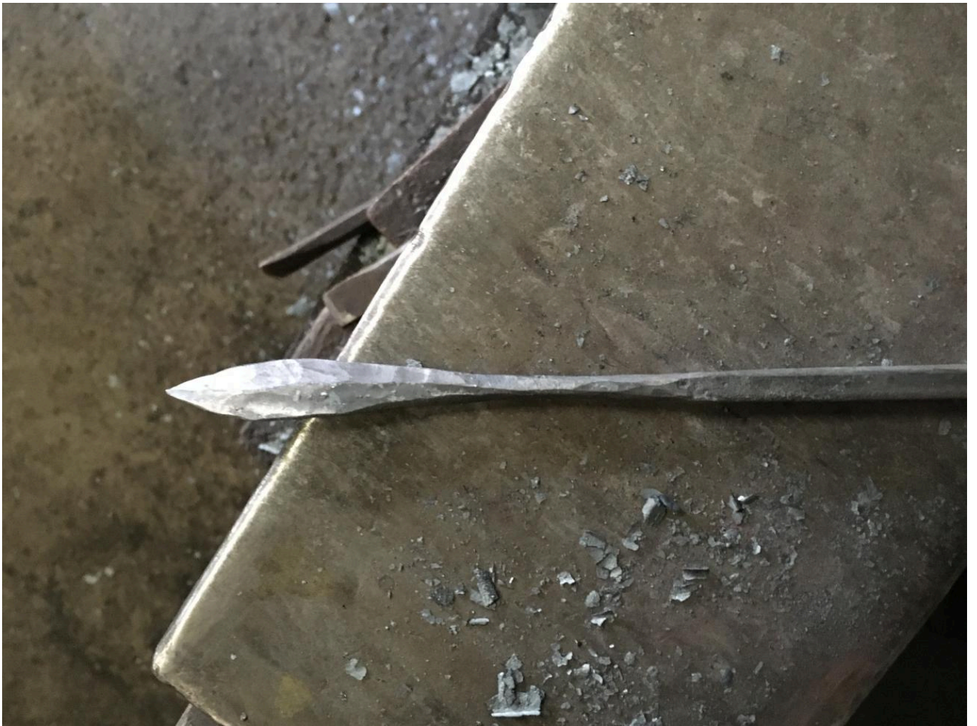
FIG 28. FORGING EDGES OF BLADE. PHOTO BY HECTOR COLE
