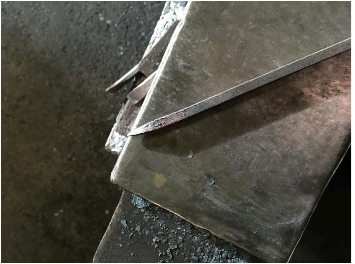
FIG 24. FORGING SQUARE POINT ON END OF BAR. PHOTO BY HECTOR COLE
