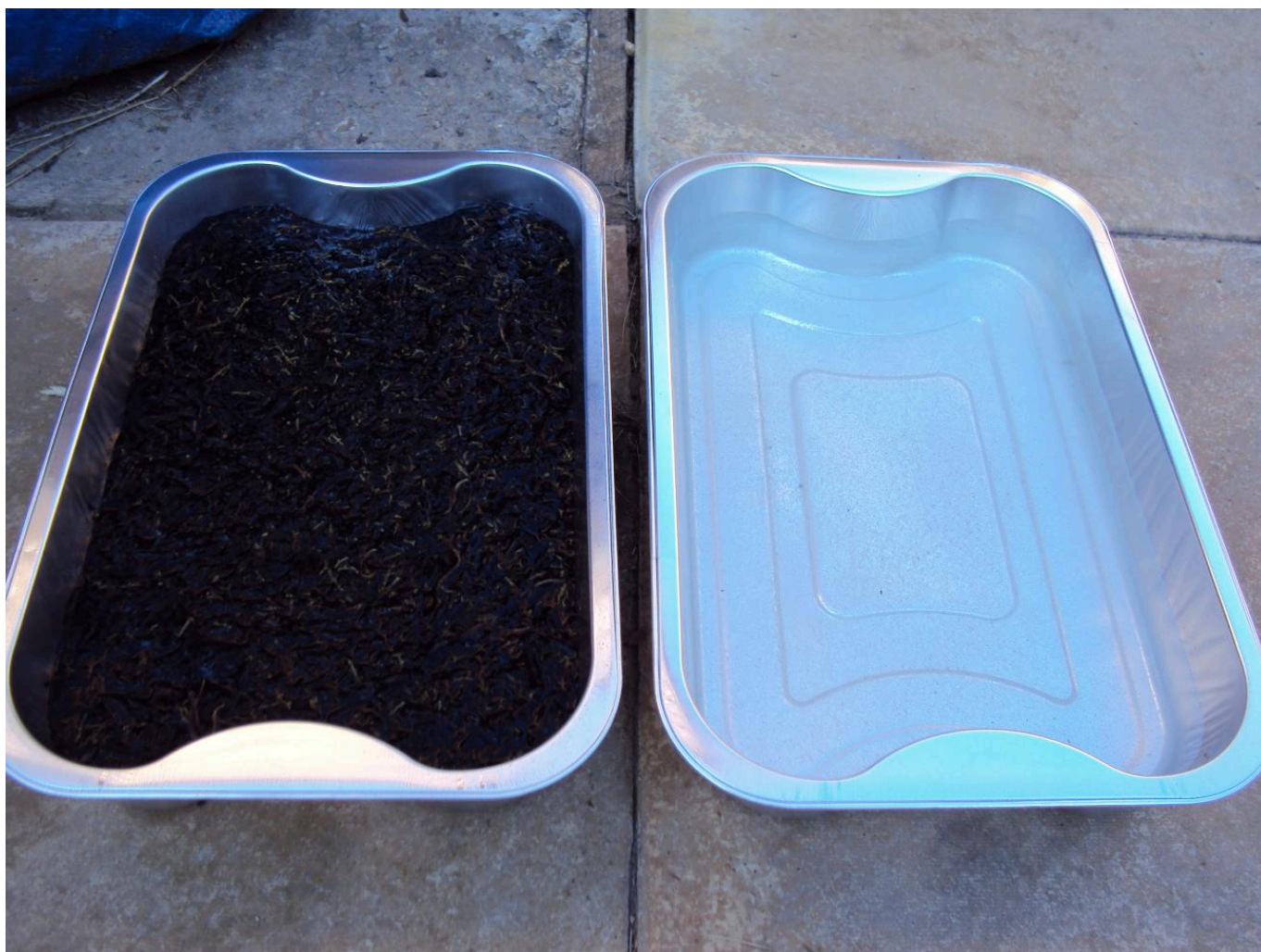
FIG 7. BRINE-MAKING (EXPERIMENT 2). ONE TRAY (LEFT) CONTAINS BURNT SAMPHIRE AND SEAWATER, THE OTHER SEAWATER ALONE.
