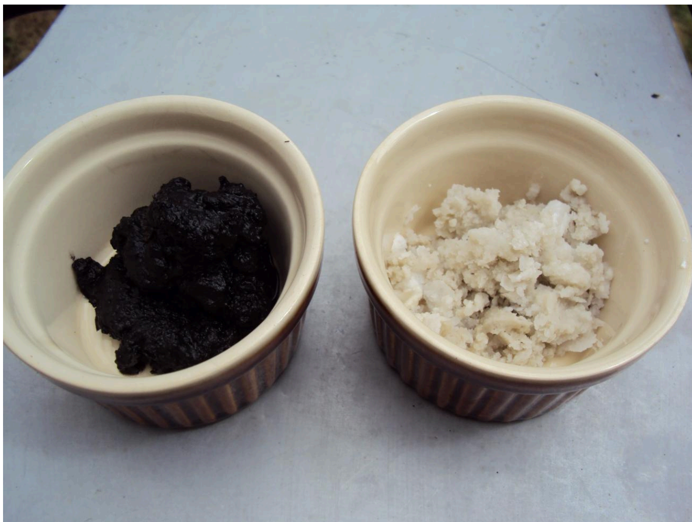
FIG 10. SALT RESULTING FROM EVAPORATING BRINE PRODUCED IN EXPERIMENT 2. THE BLACKENED SALT DERIVES FROM THE BRINE CREATED FROM BURNT SAMPHIRE AND SEAWATER.
