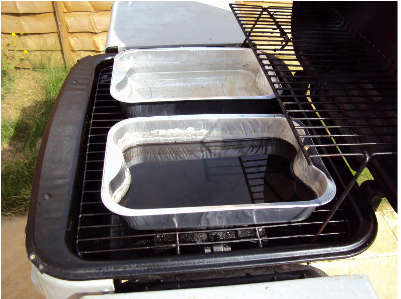
FIG 9. EVAPORATING THE BRINE OVER A MODERN HEARTH (EXPERIMENT 2)
