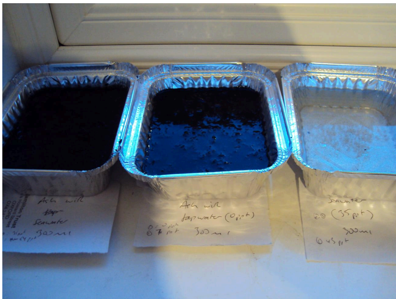
FIG 1. BRINE-MAKING (EXPERIMENT 1). ONE TRAY (LEFT) CONTAINS BURNT SAMPHIRE AND SEAWATER, A SECOND (CENTRE) CONTAINS BURNT SAMPHIRE AND HOUSEHOLD TAPWATER, THE THIRD (RIGHT) CONTAINS SEAWATER ALONE.
