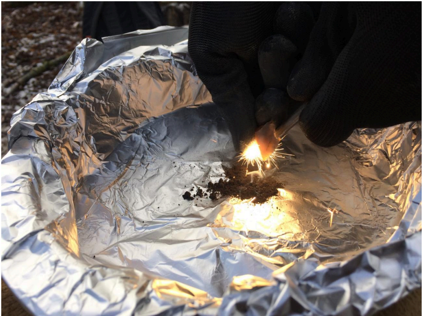
FIG 2. TESTING CHARCOAL AND \text{MnO}_2 . PHOTO BY ANDY LANGLEY
