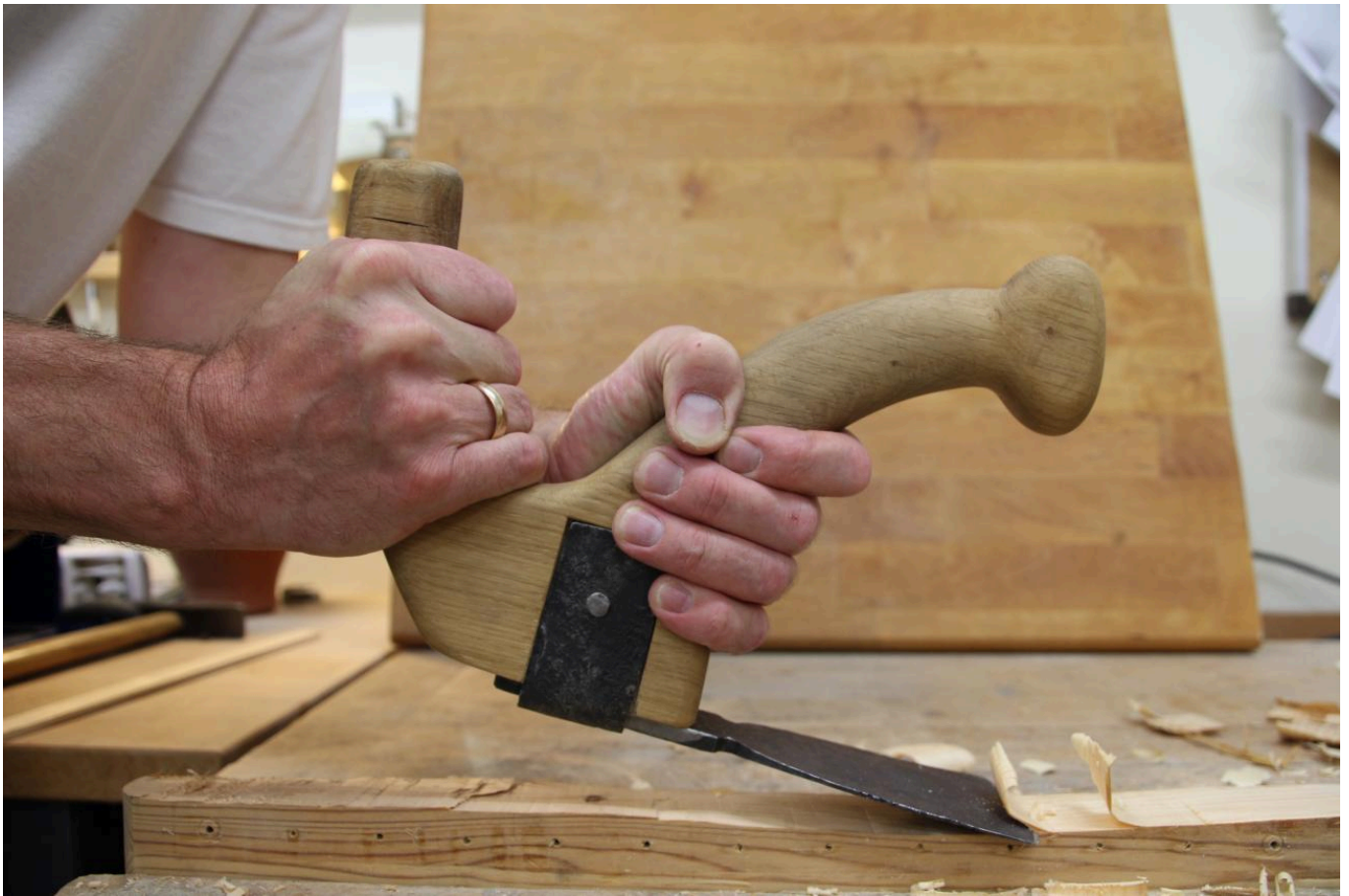
FIG 10. THE TWO-HANDLED ADZE IN USE FOR CARVING. PHOTO: ALEXANDER WEISGERBER
