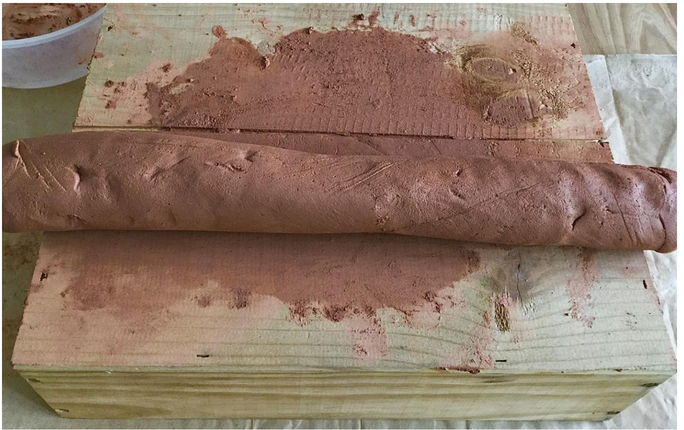
FIG 4. ROLL OF DOUGH, COLOMBINO, MADE ACCORDING TO THE ANCIENT TECHNIQUE STILL IN USE IN TUSCANY IN THE TERRACOTTA LABORATORIES. PHOTO BY L. ARIIS
