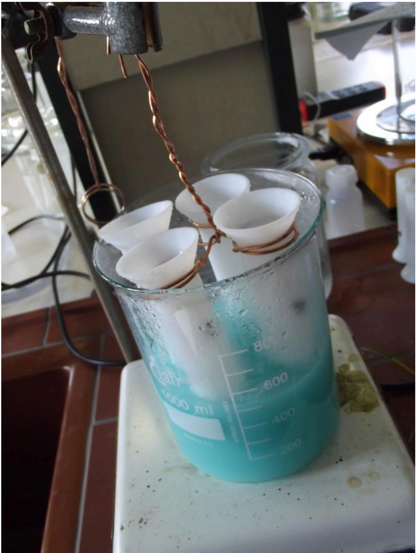
FIG 30. PATINATION SETUP WITH NIKOMI CHAKUSOKU PATINATION SOLUTION (MURAKAMI 1988)
