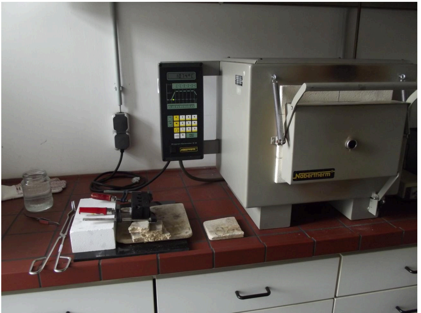
FIG 15. THE ELECTRIC OVEN WITH NITROGEN ATMOSPHERE
