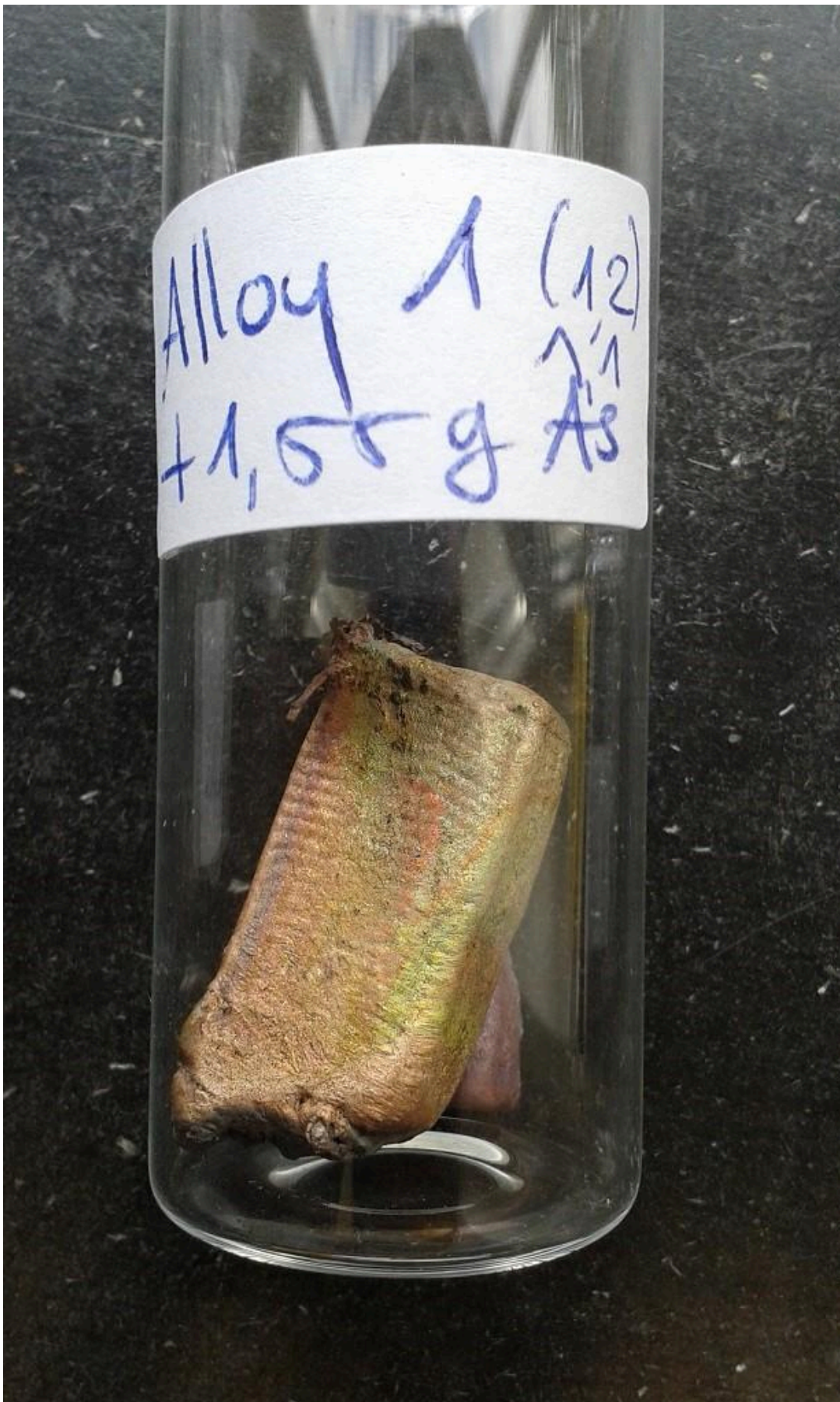
FIG 18. ALLOY 1 WITH ARSENIC AFTER CASTING IN GLASS CONTAINER
