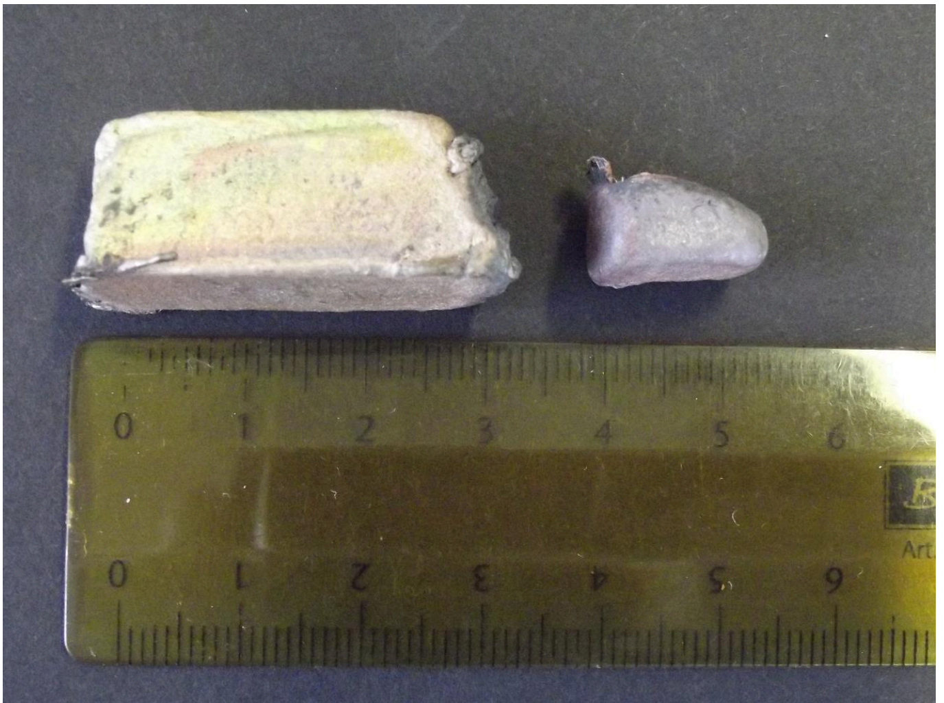
FIG 19. ALLOY 1 WITH ARSENIC AFTER CASTING WITH 1B1 PIECE
