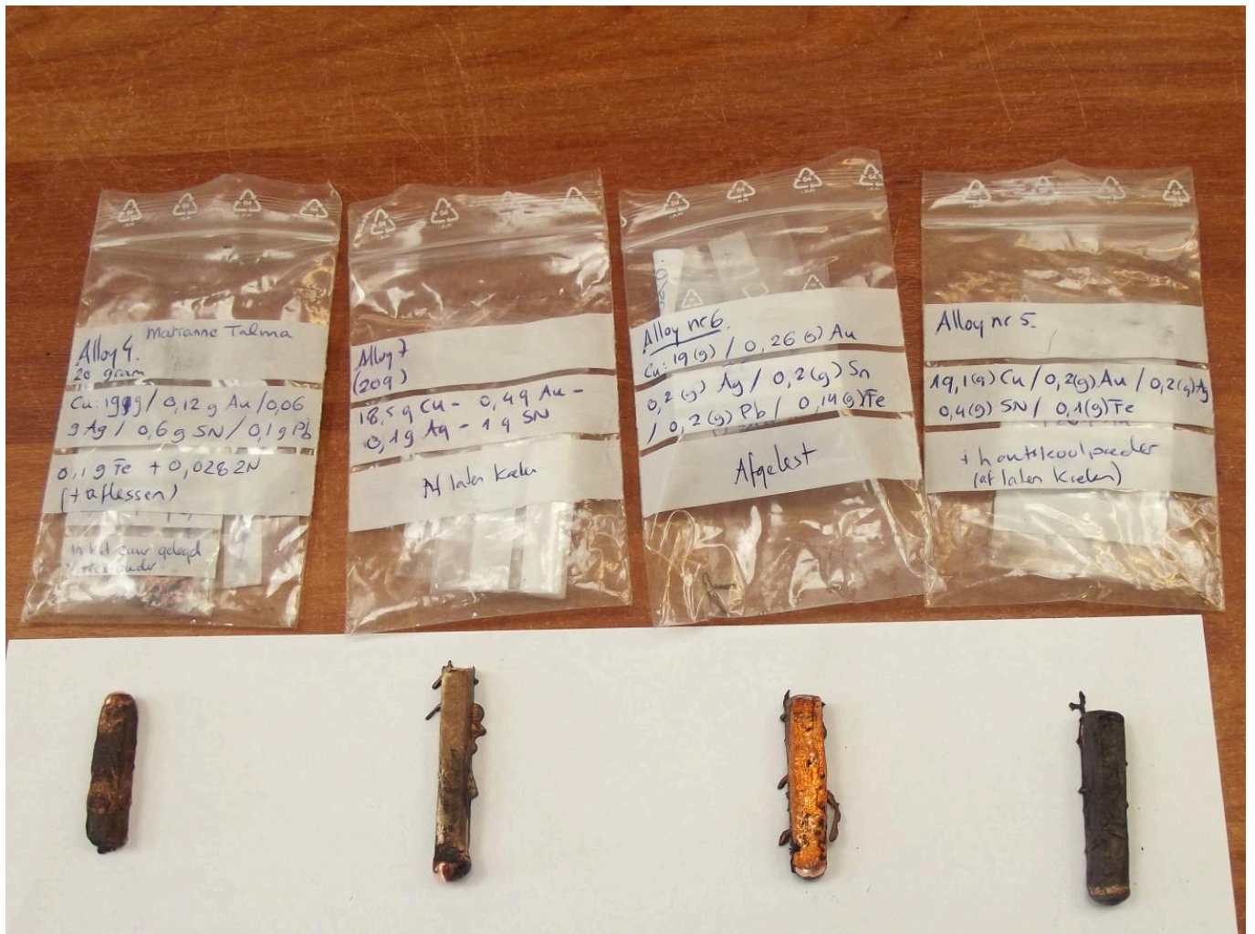
FIG 22. RESULT OF CASTING THE NON-ARSENICAL COPPER ALLOYS
