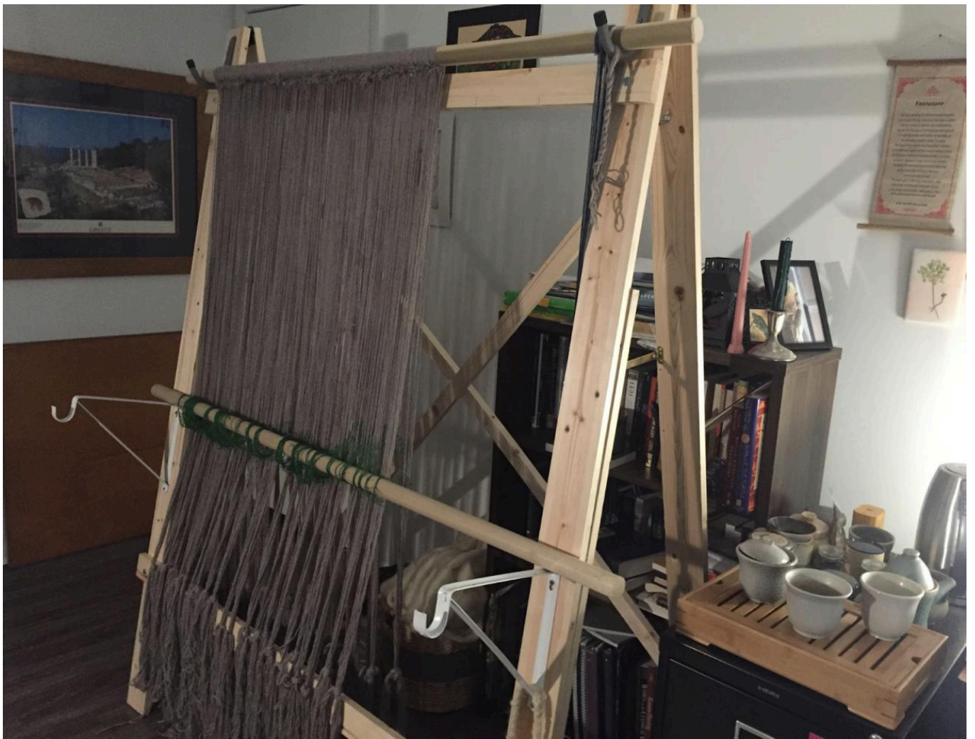
FIG 1. THE LOOM IS FULLY SET UP, AND ALL THE WARP THREADS ARE MEASURED BUT NOT TIED ONTO THEIR WEIGHTS. PHOTO BY RICHARD J. PALMER
