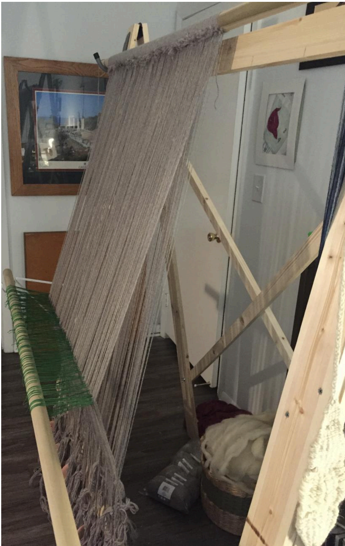
FIG 2. IMAGE SHOWS THE HEDDLES IN USE, CREATING AN OPEN SHED FOR THE SHUTTLE TO PASS THROUGH. ALL PHOTOS ARE MY OWN, UNLESS MENTIONED OTHERWISE. PHOTO BY RICHARD J. PALMER
