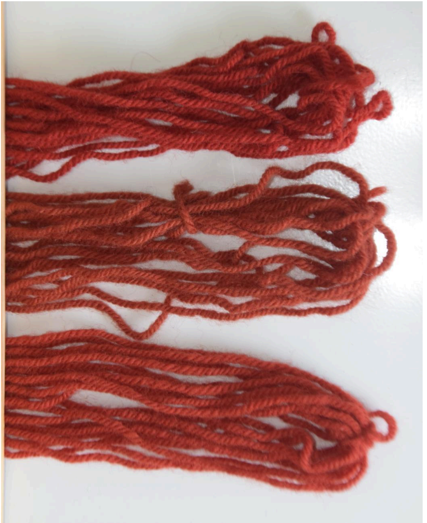
FIG 8. RESULTS FROM MORDANTING WITH VARIOUS FORMS OF ALUM. FROM THE TOP: SAMPLES MORDANTED WITH MINERAL ALUM, FIELD HORSETAIL, AND CLUBMOSS. PHOTO BY KATARZYNA STASINSKA
