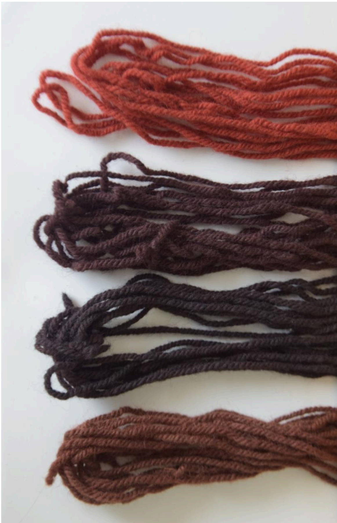
FIG 9. RESULTS FROM THE MORDANTING WITH IRON IN VARIOUS FORMS. FROM THE TOP: SAMPLES MORDANTED WITH: QUENCHING WATER (ADDED BEFORE DYEING), IRON SULPHATE, 'IRON WATER' ADDED BEFORE DYEING, AND 'IRON WATER' ADDED AFTER DYEING. PHOTO BY KATARZYNA STASINSKA
