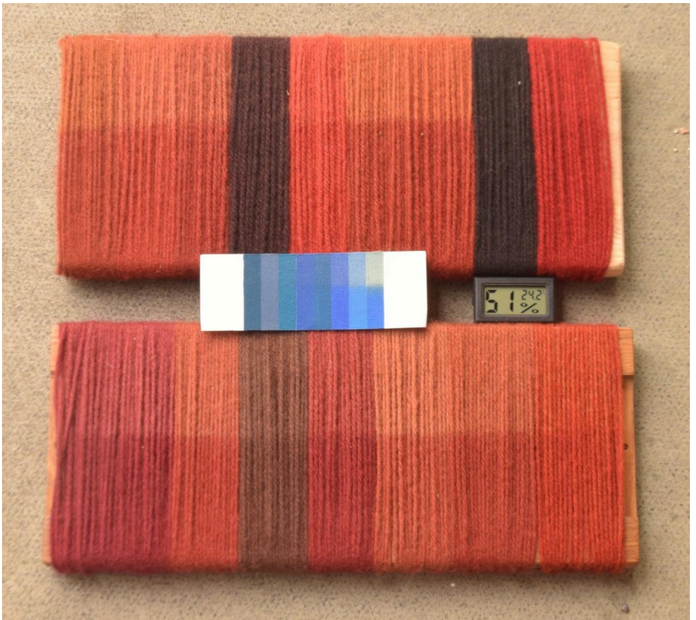
FIG 10. A VARIETY OF SHADES RECEIVED FROM MADDER COMBINED WITH VARIOUS MORDANTS AND ASSISTS (TOP HALF OF EVERY SKEIN EXPOSED TO THE SUN FOR APPROXIMATELY 150 HOURS). PHOTO BY KATARZYNA STASINSKA
