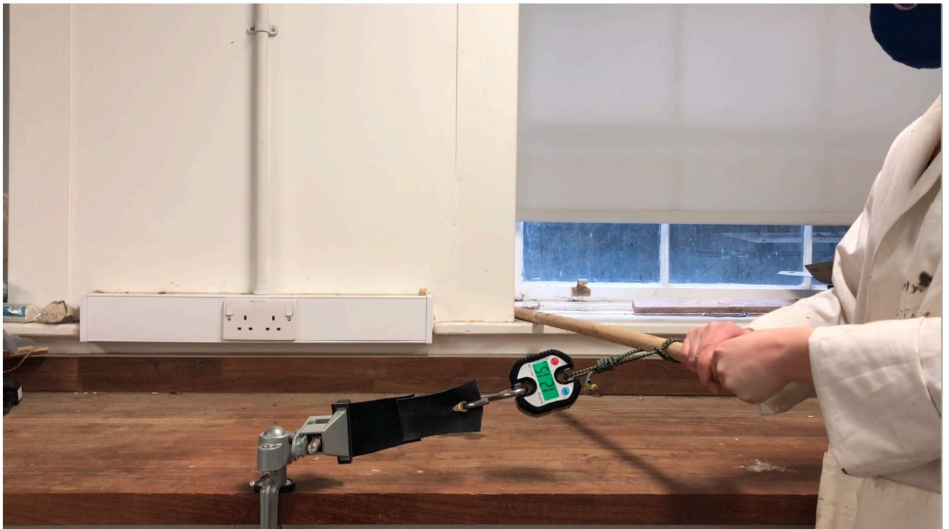
FIG 2. PHOTOGRAPH OF A LAP-SHEAR TEST IN ACTION. PHOTOGRAPH BY PHOEBE BAKER.
