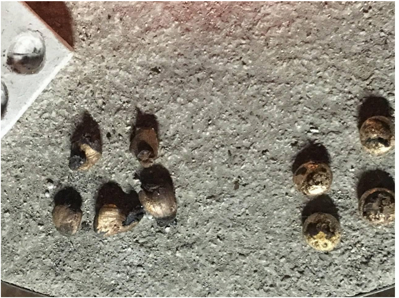
FIG 4. COOLED PELLETS MADE WITH AND WITHOUT FLUX.
