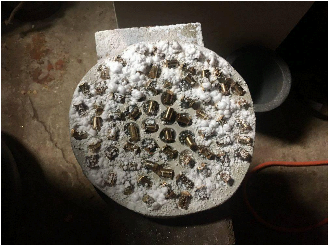
FIG 2. PELLET MOULD LOADED WITH COPPER ALLOY AND FLUX.
