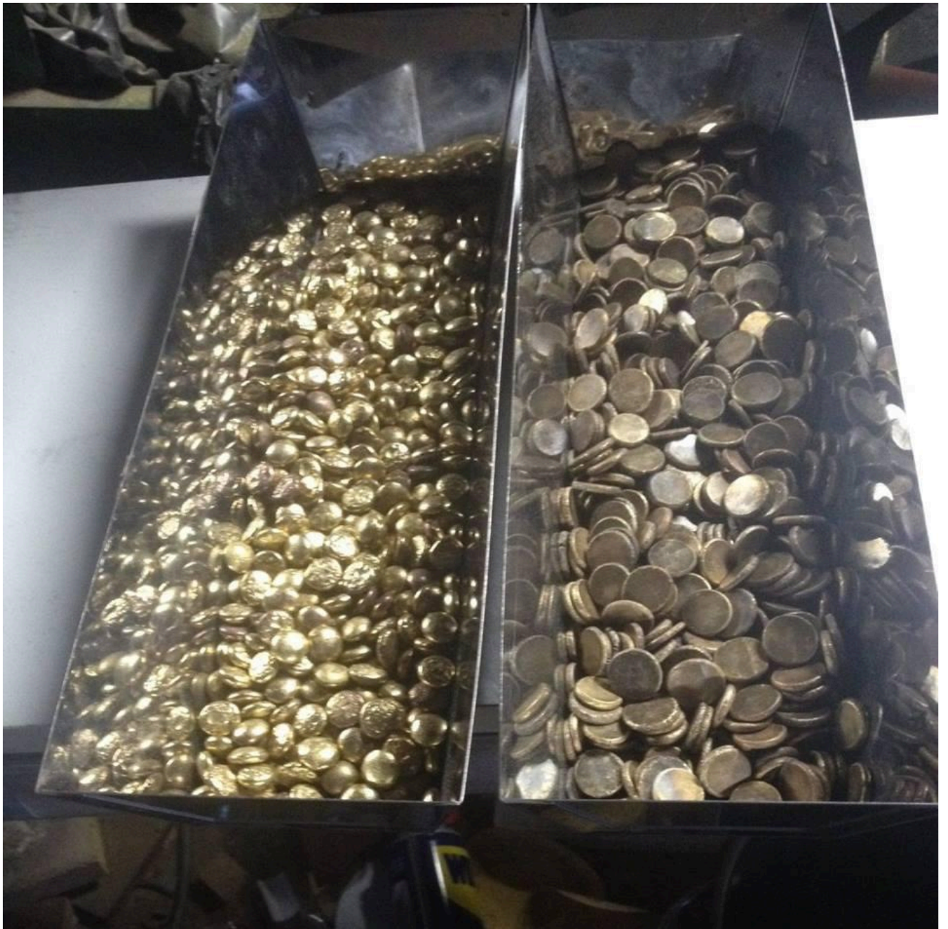
FIG 5. BINS OF PELLETS AND FLATTENED COIN BLANKS.
