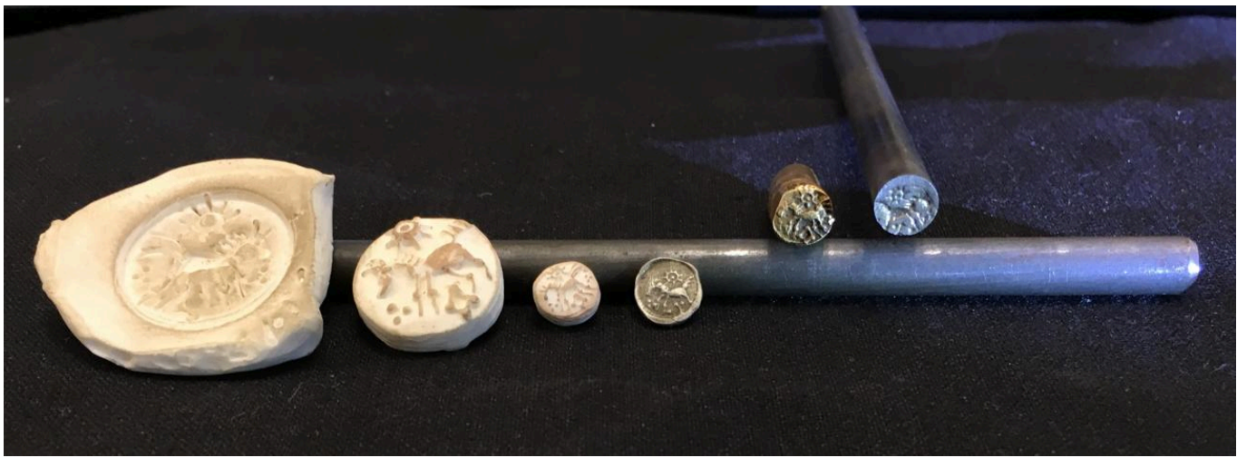
FIG 11. CLAY COIN, COPPER ALLOY SLUG, STEEL DIE, AND RESULTING COIN FOR THE SAME COIN DESIGN.
