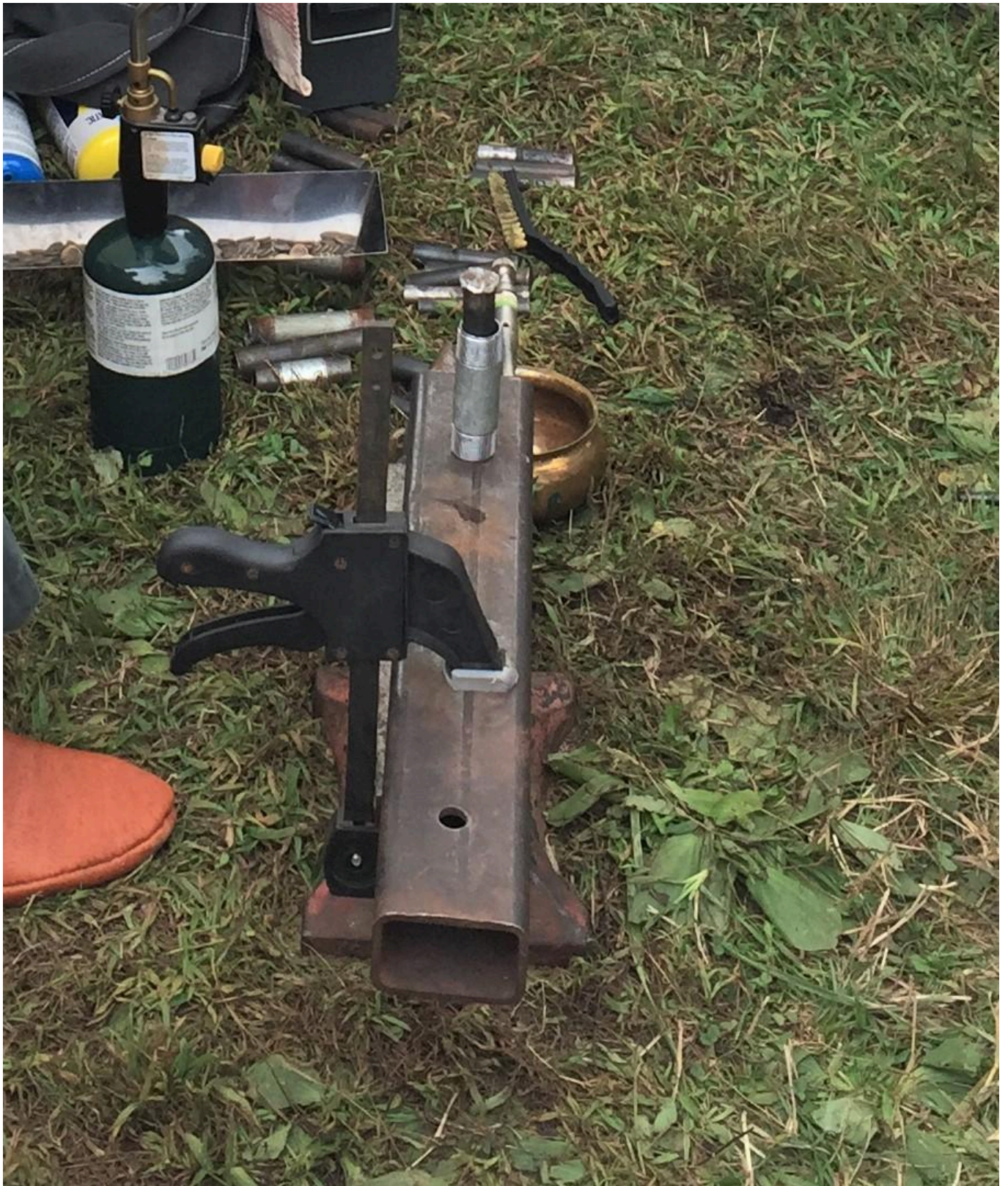
FIG 10. COIN STRIKING ASSEMBLY
