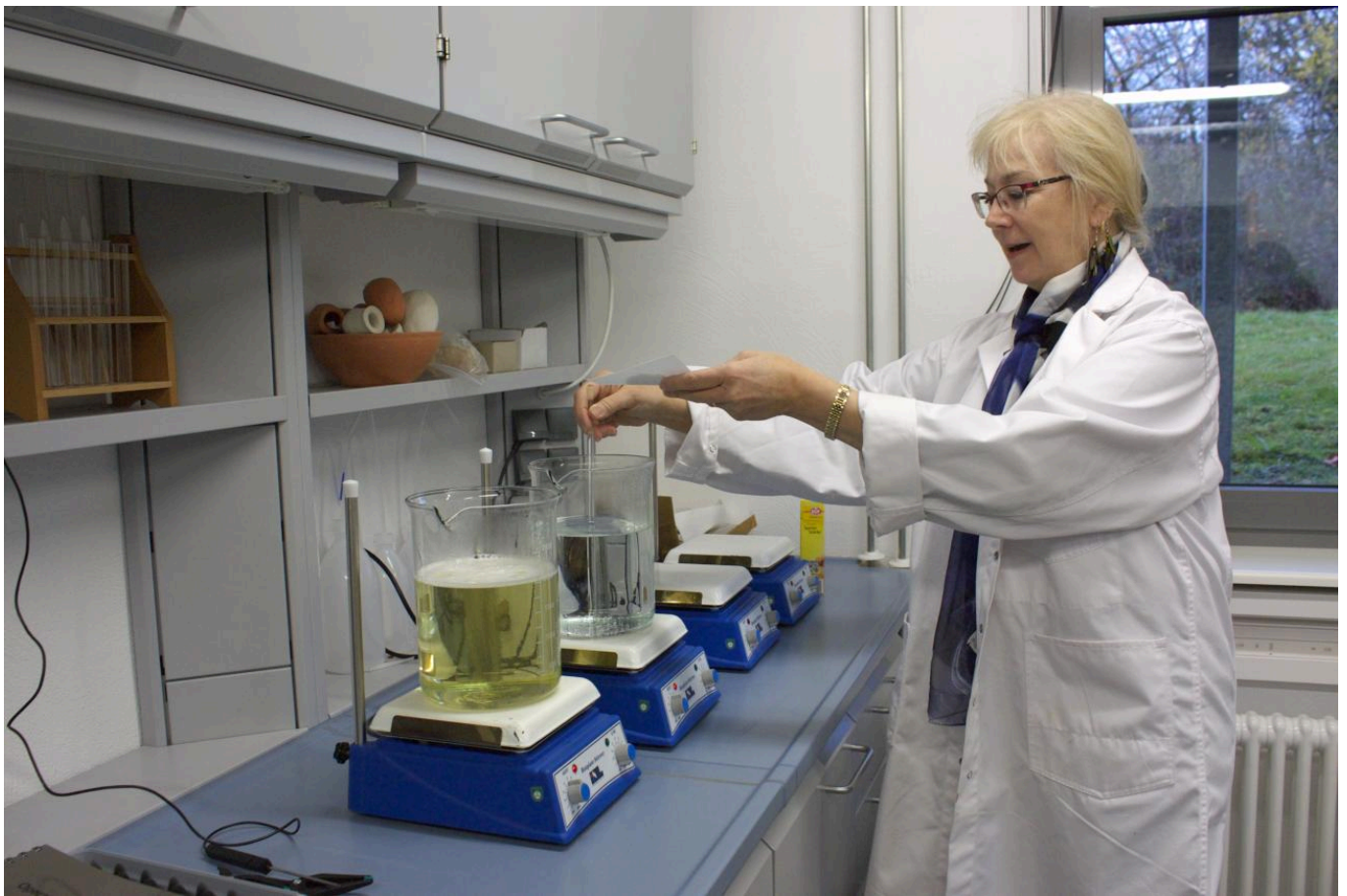
FIG 1. PREPARING DE-GUMMING BATHS FOR SILK. COPYRIGHT: KATRIN KANIA
