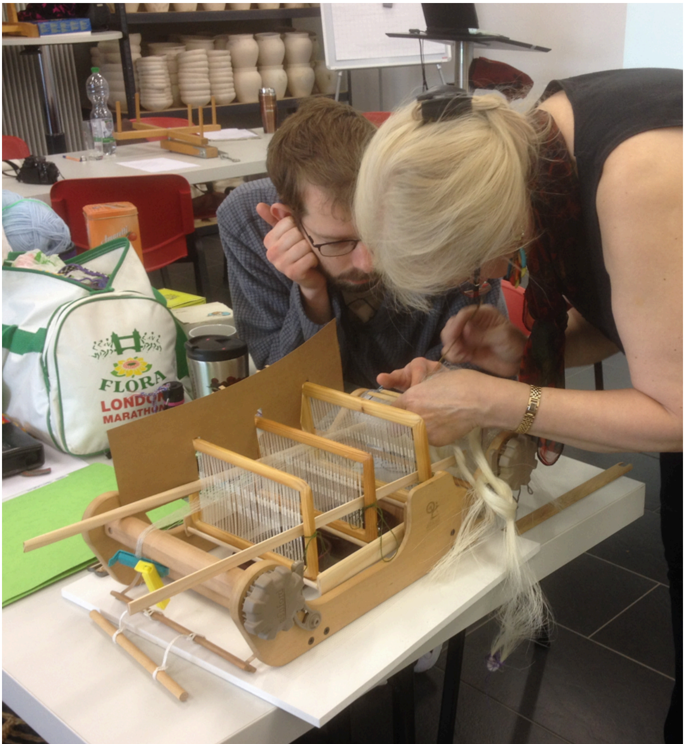
FIG 8. SETTING UP A SMALL LOOM FOR SILK WEAVING TESTS WITH NON-DE-GUMMED SILK IN THE WARP. COPYRIGHT: HEATHER HOPKINS
