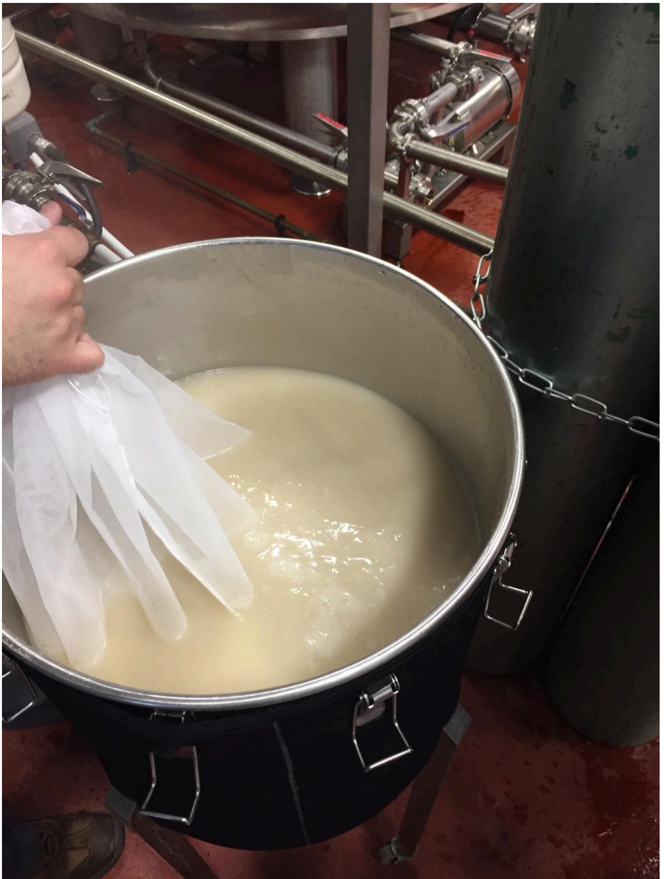
FIG 3. ADDING THE NYLON MESH BAG CONTAINING THE BREAD TO WATER.
