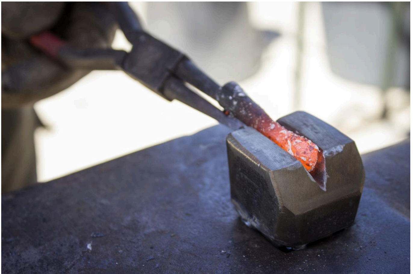
FIG 9. SHAPING THE TRIANGULAR POINT BY A HARDY TOOL. PHOTO BY RUBEN CATALDO.
