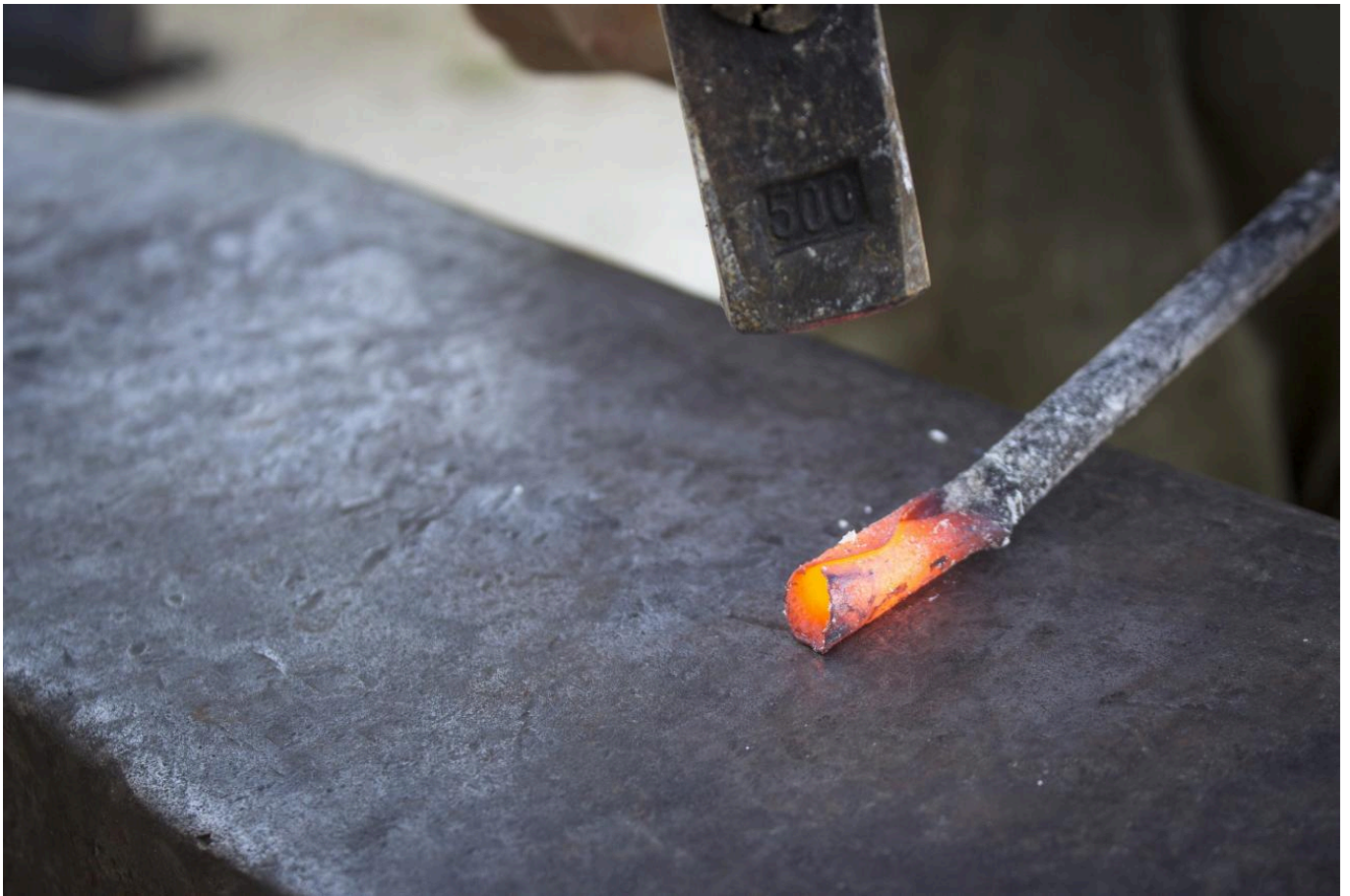
FIG 6. CLOSING OF THE SOCKET. PHOTO BY RUBEN CATALDO.
