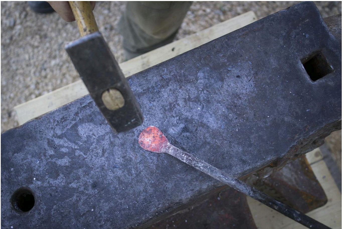
FIG 4. FLATTENING PHASE OF THE BAR'S EXTREMITY CREATING A "SPOON" SHAPE. PHOTO BY RUBEN CATALDO.
