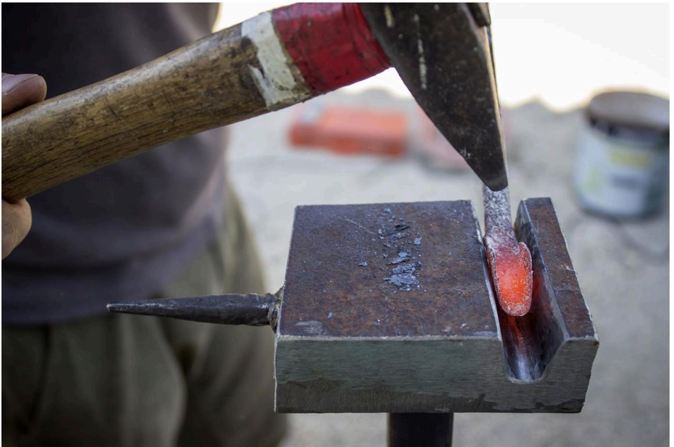
FIG 5. PUSHING THE BAR'S FLATTENED PART INTO A HARDY TOOL, FORMING A U SHAPE. PHOTO BY RUBEN CATALDO.
