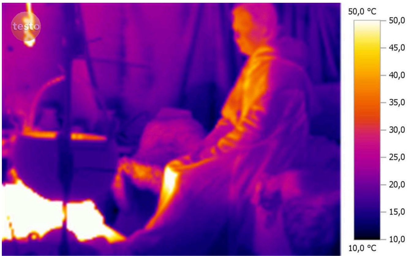
FIG 5. THERMAL IMAGE SHOWING THE ASYMMETRIC SURFACE TEMPERATURE ON A PERSON'S CLOTHES (APPROXIMATELY 15-50 °C) AND ON THE INTERIOR (DOWN TO 10-25 °C). PICTURE: CHRISTENSEN 2013A
