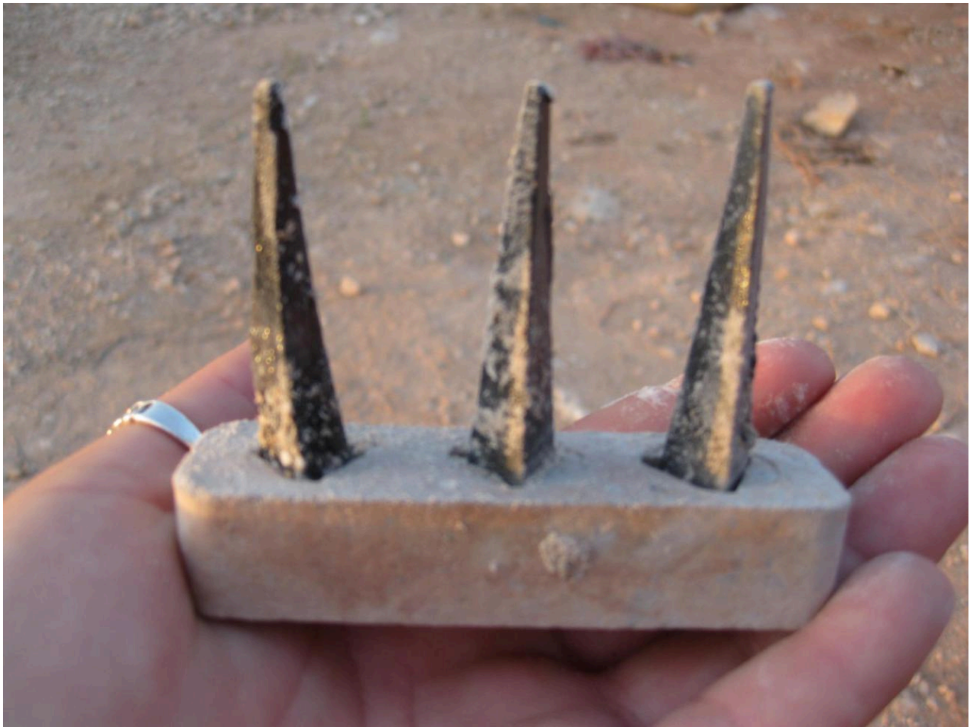
FIG 31. ORTON CONES DID NOT BEND IN THE FIRING TO CONFIRM TEMPERATURE BUT ONLY BLISTERED IN THE FIRING.
