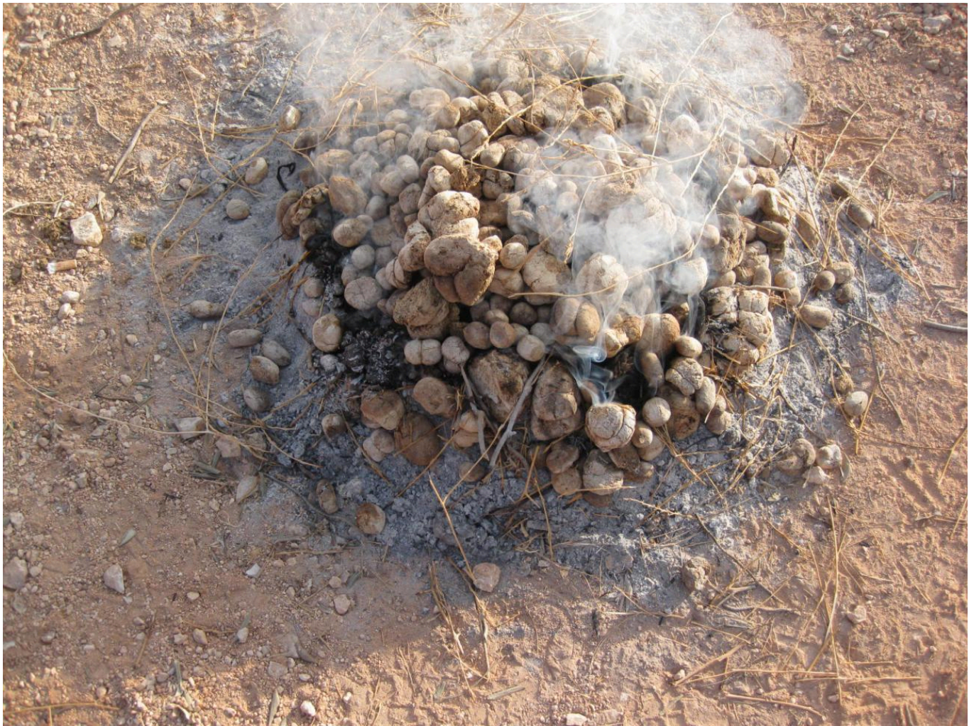
FIG 25. 7:15 AM: VESSELS COMPLETELY COVERED WITH CAMEL DUNG FROM 3RD AND 4TH BUCKETS, WHICH BEGIN TO CATCH ON FIRE.
