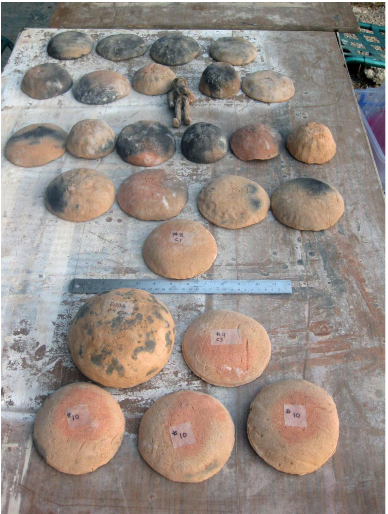
FIG 32. FIELD LABORATORY, MADABA, JORDAN: TWENTY-FIVE CLAY VESSELS FIRED WITH PREDOMINANTLY CAMEL DUNG FUEL. AVERAGE SIZE OF HAND-MADE CLAY VESSELS: DIAMETER 9-11 CM, DEPTH 3 CM, THICKNESS OF WALLS 0.3 CM. ONE LARGER COIL-MADE VESSEL MEASURED: 14 CM DIAMETER, 11 CM DEPTH, AND THICKNESS OF WALLS 0.3 CM.
